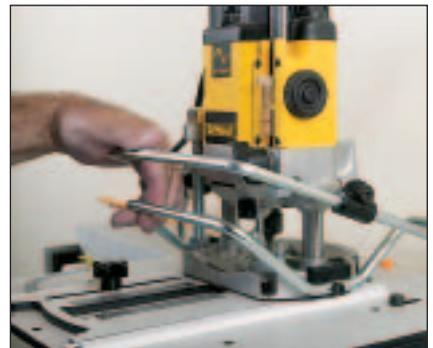
The PlungeBar accessory, available for most plunge routers, enables you to plunge the router with one hand.
