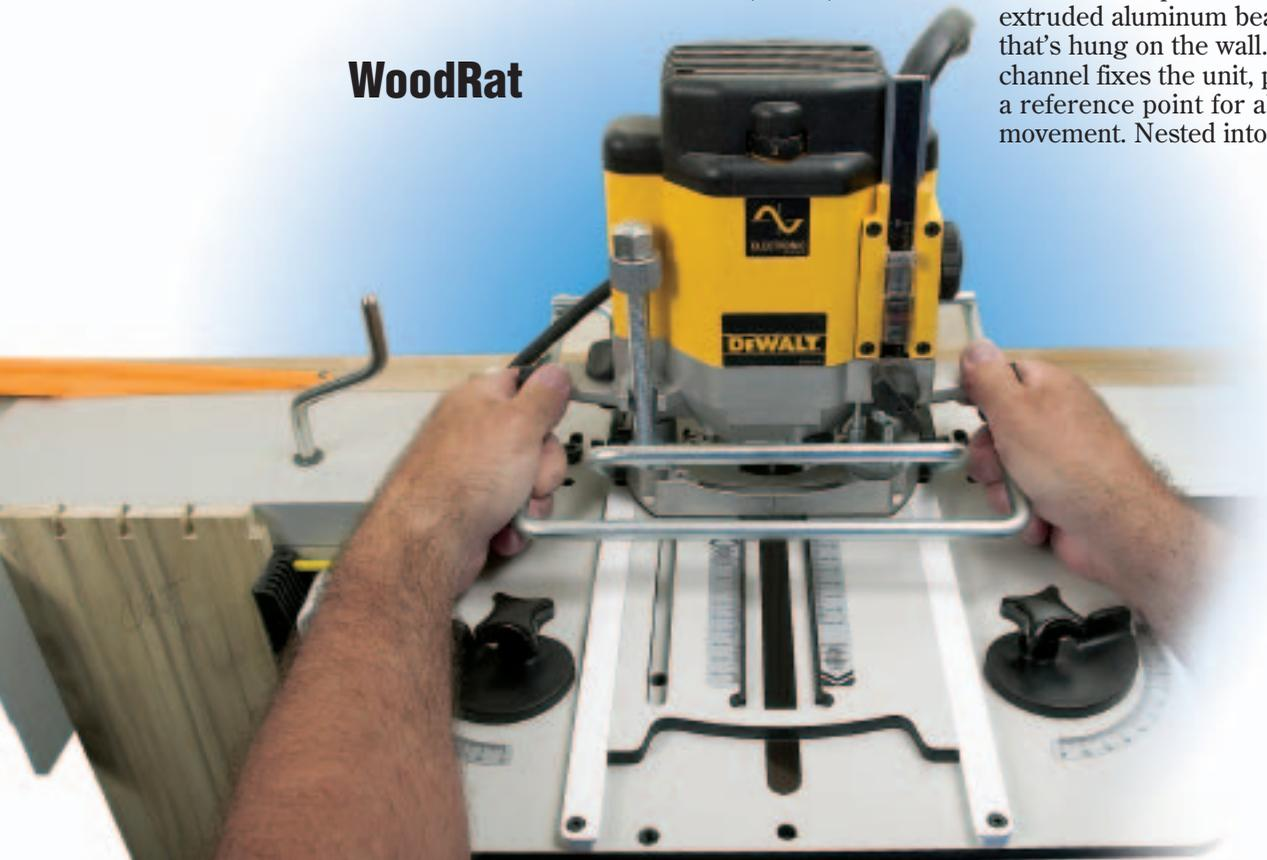
of the channel is the sliding bar. Two parallel vertical fences, each opposed by an adjustable cam clamp, enable you to secure work to the sliding bar, and a crank and cable mechanism allows you to move the sliding bar left and right, taking the work with it. This is the first axis of movement.
