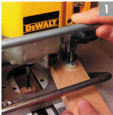
▲ Make two test boards. Zero the dovetail cutter on one board while using the other board to set the depth stop.
