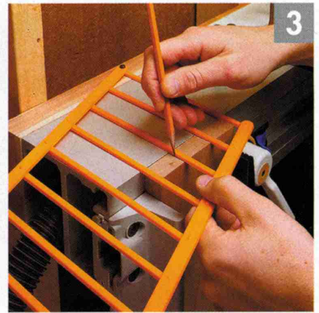
▲ Use the parallelogram to mark tail locations on a workpiece. The parallelogram adjusts for custom layouts.
