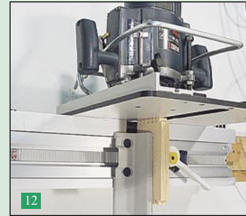
above Aluminum guide rails can be used to cut comb joints
