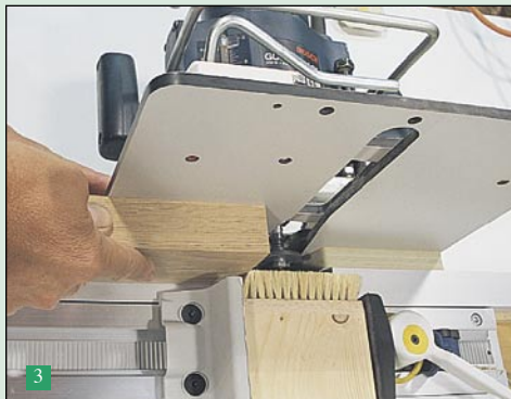
above Feeding the wood past the bit by hand. The brush acts as a featherboard and a guard
