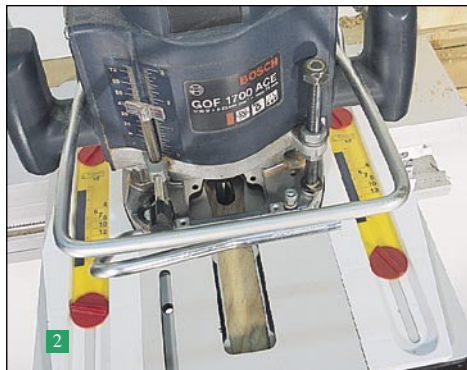
above A dovetail slot being cut in a table leg. The center line is now removed
