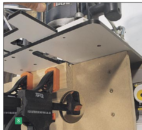
above The mortise is cut with the wood clamped to the shop-made mortise rail
