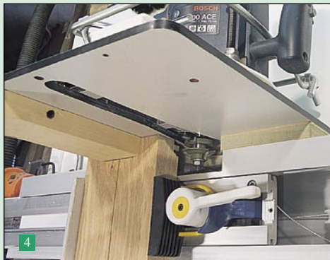
above The vise has a sacrificial face that prevents breakout when cutting joints like this rail & stile
