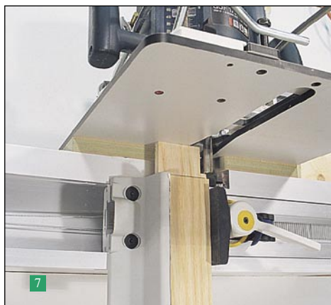
above Cutting a tenon with the LittleRat
