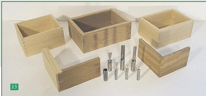
above A range of dovetails that can be cut with the LittleRat
