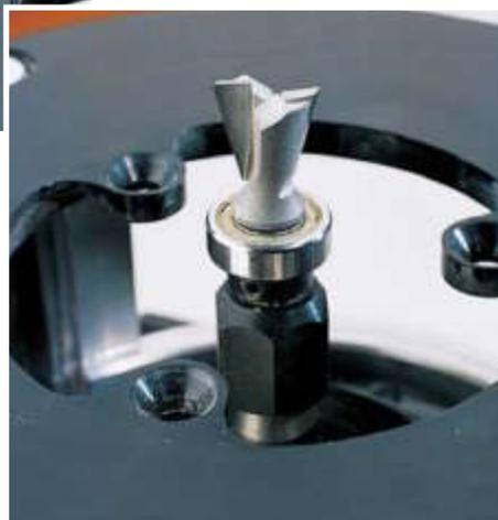
**4** A special bit with a bearing comes with the Woodhaven dovetail jig. The bearing replaces a template guide. This bit won't work with other jigs, however, because it requires an extra-thick template.
