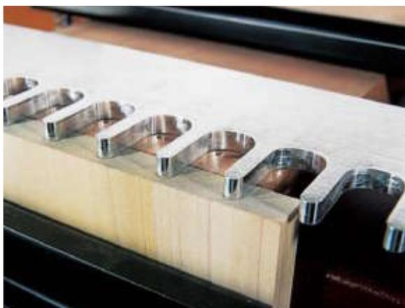
**5** A rigid template makes it easier to align the pin and tail boards. You're more likely to get consistently accurate results with a rigid template (such as the Hart, shown here) than with one that bends slightly.
