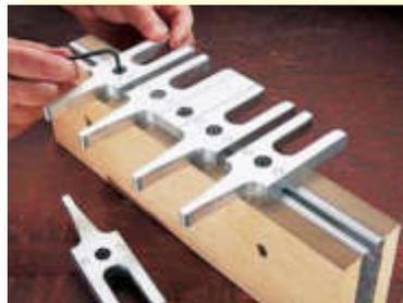
**It's adjustable.** Move the jig's guide forks to customize the spacing between dovetails.
