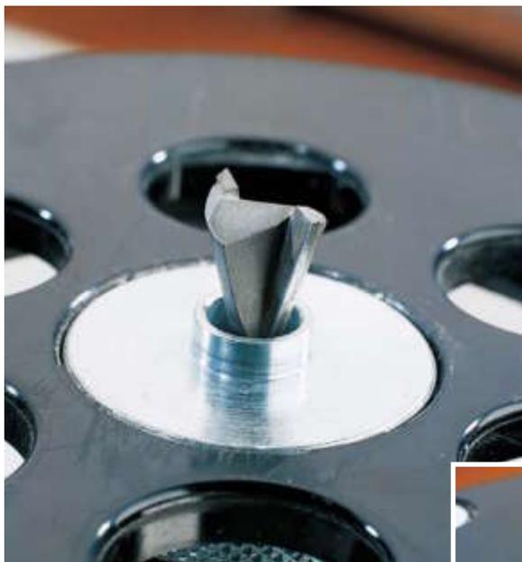
**3** You'll need a specific-diameter guide to follow the template of a half-blind dovetail jig (see Chart, page 70). Woodworking catalogs offer template guides for most fixed-base routers, but you may have to special-order yours from a dealer.
