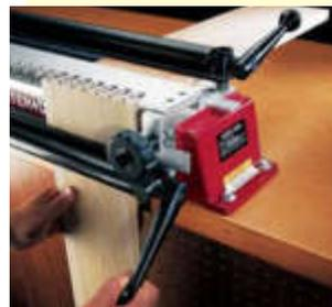
**Quick-action board clamps** let you move lumber through this jig at a rapid rate. The clamps are as stout as the rest of the jig, which looks like it can take years of hard use.
