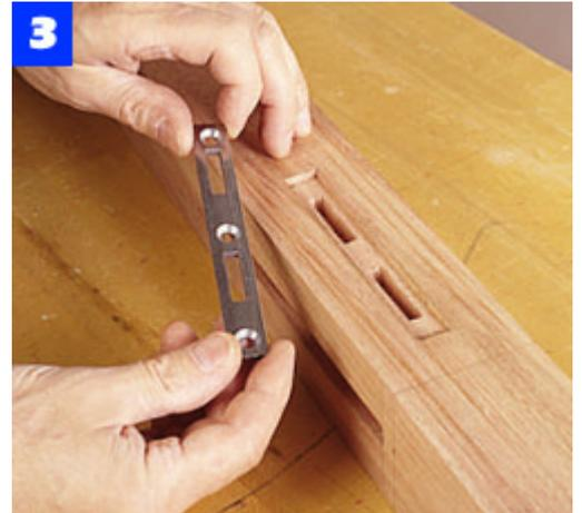
3 Rout the mortises in the posts for the rail-hanger hardware. Then, test the fit and bore screw pilot holes.
