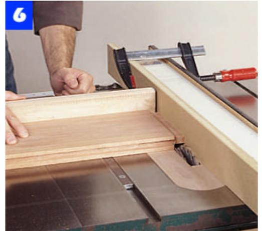
Clamp a scrap board to the rip fence to act as a stop when cutting the tenons on the ends of the rails and stiles.
