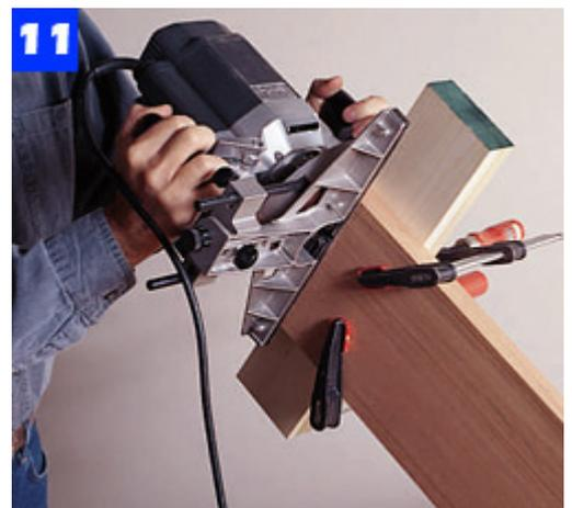
To rout the hanger mortises, clamp a board to the rail for router support. Use a small chisel to cut the deeper recesses.
