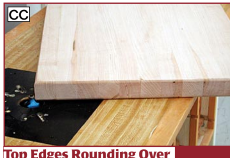
Top Edges Rounding Over
