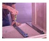
14--Install the case tracks by screwing through the horizontal slotted holes. Place tracks flush with the front edges of case.
