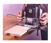
10--Rout grooves for the drawer bottoms in the drawer front and side panels. Use a 1/4-in. straight bit and router edge guide.
