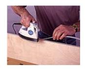
1--Heat the hot-melt adhesive on the back of the veneer tape with an iron. Slowly advance the iron with firm pressure.
