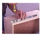
13--Fasten the drawer halves of each track to the drawer sides with screws driven through the vertical slotted holes.
