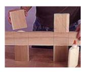
6--Spread glue in the slots and on the plates and assemble short rails to the mullion. Clamp the subassembly until the glue sets.
