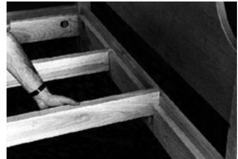
16 Use a bed bolt wrench and an open-end wrench to tighten the connection between the rails and posts.
