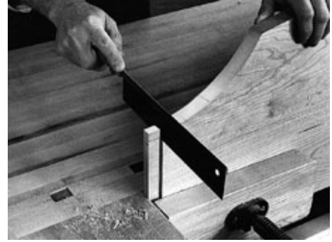
10 With the headboard edges smoothed, mark and cut the shoulders at the top and bottom of the tenon.
