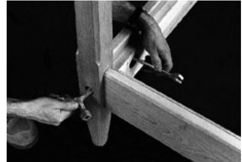
16 Use a bed bolt wrench and an open-end wrench to tighten the connection between the rails and posts.
