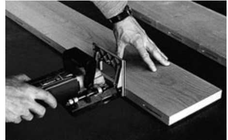
7 Rip and crosscut the headboard stock oversize. Cut joining plate slots in the stock, then glue and clamp the stock.
