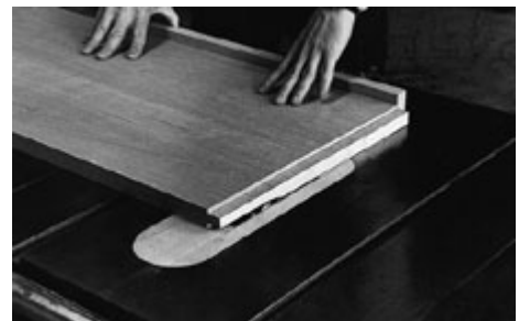
7 Rip and crosscut the headboard stock oversize. Cut joining plate slots in the stock, then glue and clamp the stock.
