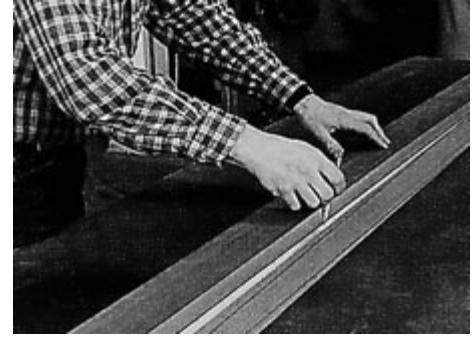
1 Rip and crosscut the post blanks, and use a long straightedge to mark the taper. Also mark the mortise positions.
