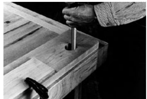
11 Use a long bit to bore slowly through the post holes and into the headboard and rail tenons.
