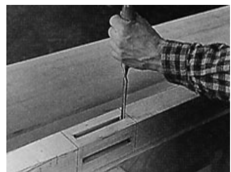
2 Cut the post mortises before sawing the tapers. Use a plunge router or bore out the mortises on the drill press.
