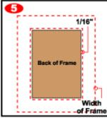
Transfer the measurements to the front and draw lines for the miter cut. Cut the miters with your compound miter saw. Then sand the frame parts to make them smooth.
