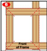
7. After gluing the joints, use bar clamps or framing clamps to clamp the pieces together, making sure to keep the frame perfectly square and the corners smooth and even. Once the glued frame is set measure for the inlay and cut it with a razorblade making three to five passes. Fit the inlay in the channel with slight pressure. If it does not quite fit, make a couple shaving strokes with the edge of the razor blade until it matches perfectly.
