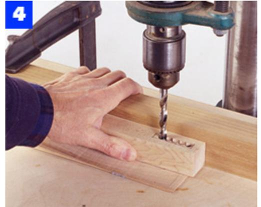
Begin the upper back rail mortises by boring a series of 3/8-in.-dia. holes. Then finish the job with a sharp chisel.
