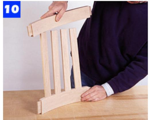
10 Begin stool assembly by joining the slats to the curved back rails. No glue is necessary in these joints.
