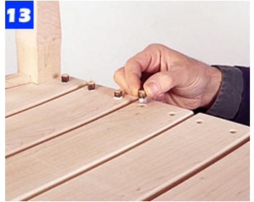
Screw the seat slats to the rails and install the plugs. When the glue dries, pare the plugs flush to the seat surface.
