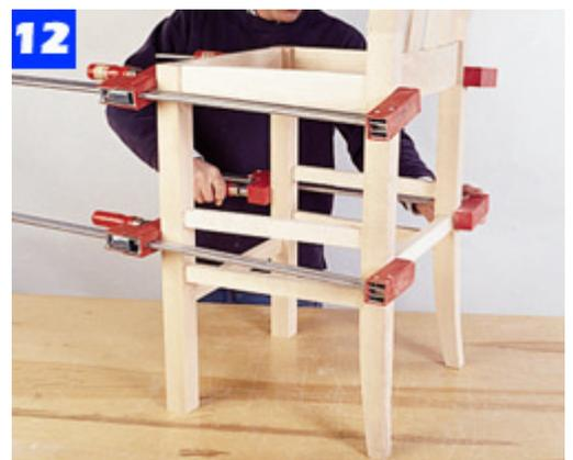
12 Join the rear and front subassemblies with the side rails. Set the stool on a flat table to check that the legs are even.
