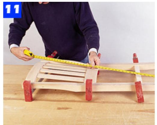
11 Join the back rails to the rear legs and clamp. Compare opposite diagonals to check that the assembly is square.
