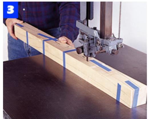
After cutting the leg profile along one face, tape the waste back on the leg to provide a base for the adjacent face cuts.
