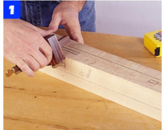
Use a tape measure, square and mortise gauge to lay out the locations of the mortises in the leg blanks.
