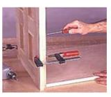
8--Clamp the grid assemblies to the case sides. Bore and countersink screw pilot holes and drive screws to fasten the grids.
