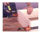
11--Apply glue to the drawer box joints. Then clamp the boxes together and drive nails at the corners. Set the nailheads.
