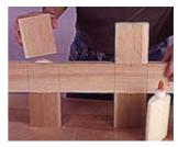
6--Spread glue in the slots and on the plates and assemble short rails to the mullion. Clamp the subassembly until the glue sets.
