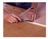
2--Use a sharp chisel to trim the overhanging edges of the veneer tape. If the tape begins to tear, reverse the cutting direction.
