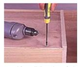
12--After sliding the 1/4-in. bottom panels in place, secure them to the drawer backs with 3/4-in. No. 6 rh screws.
