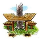
**9. Set the bench.** Set the section with four bench supports in the postholes first. Then lower the other section into place. Make adjustments until the bench is level all around. Install the final screws, set the posts into the holes, and tamp in place.
