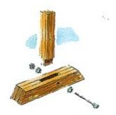
**8. Install the posts.** Cut six 4x4 posts to the correct length—the depth of the hole plus 16 inches. Cut a tenon on one end so that the post will fit into the bench support. With your bench sections upside down, install each post, fastening it securely with a 5-inch hex bolt, a washer, and a nut.
