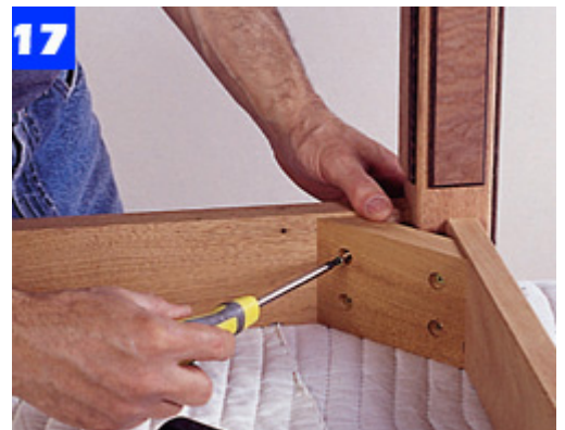
Cut corner blocks to size with 45° angles at each end. Countersink screwholes in the blocks and secure to the aprons.
