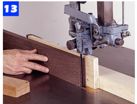
13 Resaw the wenge decorative panel stock on the band saw. Use a tall fence to hold the work parallel to the blade.
