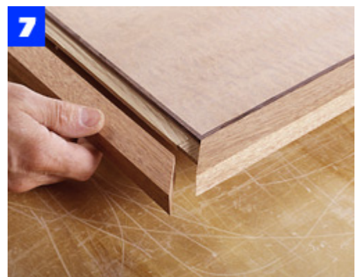
After routing spline grooves and cutting mahogany edge strips, test fit splines. Then glue edging one piece at a time.
