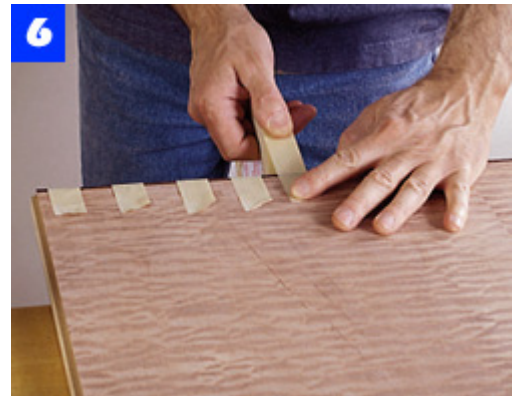
Apply glue to the rabbet and use masking tape to clamp the inlay to the panel. Sand the inlay flush to the top.
