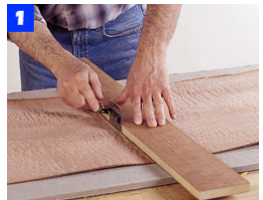
Stack all top veneer pieces and cut them at one time. Align the grain and use a straight board to guide the veneer saw.
