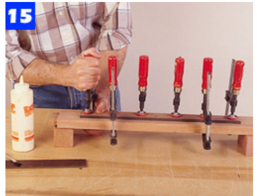
After trimming and beveling the panels, lightly spread glue on each and clamp in place until the glue sets.
