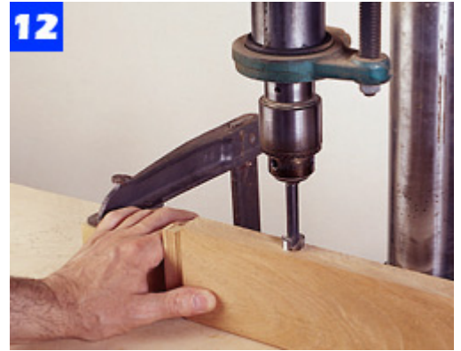
12 Clamp a fence to the drill press table to help position the aprons when cutting the tabletop fastener mortises.
