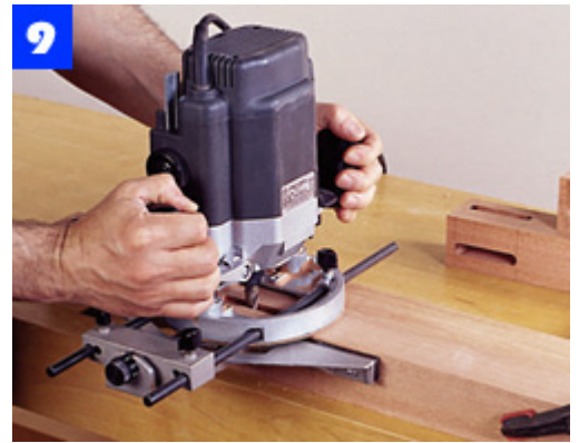
Use a spiral up-cutting bit to rout the leg mortises. Make the cut in several passes to ease the load on the router.
