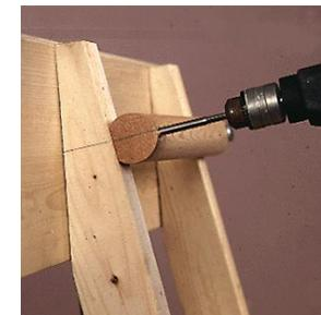
frame. Secure the ladder in place with 8-inch-long carriage bolts. (Tip: If the ladder attachment bolts don't reach all the way through on the inside, you can countersink the nuts with a 1-inch bit or get 9-inch bolts and trim them with a hacksaw.)
