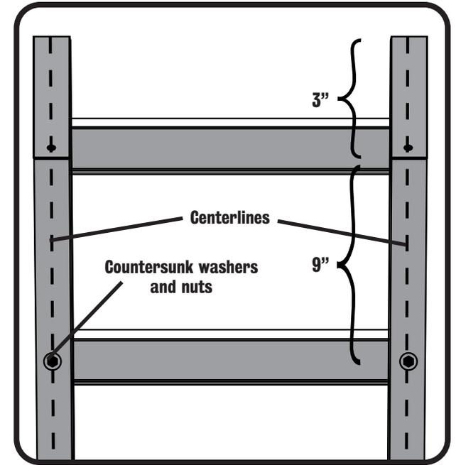
inch-long carriage bolts, with washers and nuts countersunk on the back side. Position the ladder against the bed, 4 inches in from the end. Draw guidelines on the ends of the top rung, as shown in the bottom photo, and hold the rung so the lines match up with your earlier marks on the sides of the 2 by 3's. Drill through the rung into the frame with a long ⅜-inch bit. When you have sunk the bit in as far as you can, remove the ladder and continue the hole through to the inside of the
