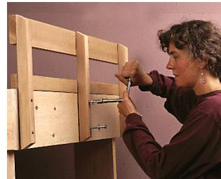
end of each post on the three fixed railings with a  $\frac{3}{8}$ -inch bit, 2 inches and 6 inches up from the bottom, and  $\frac{3}{4}$  inch in from the side.
