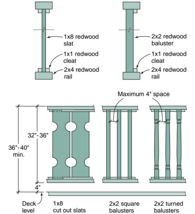
**Cutout slats** This style often expands on a custom design detail from the frieze and it can be as simple as the oval pattern shown above, or as elaborate as the gingerbread designs of the Victorian era. Create a template from hardboard and transfer the pattern to the 1x8 redwood slats. Use a band or saber saw to cut the pattern from several boards at a time. Secure the redwood slats to the rails with nailing cleats.
