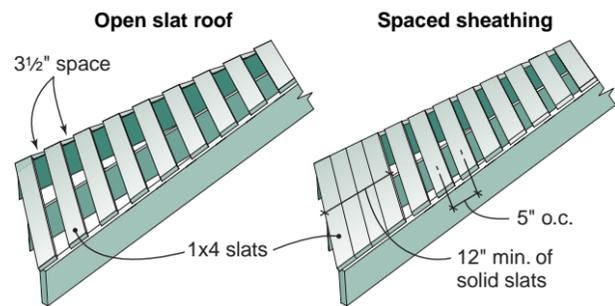
**Shingles over spaced sheathing** Follow the basic slat roof construction steps. Add two more slats at the roof's edge to simplify installation of the starter course. Space the rest of the slats five inches on center or to match the weather exposure. Other installation details are the same as for shingles installed over plywood sheathing.
