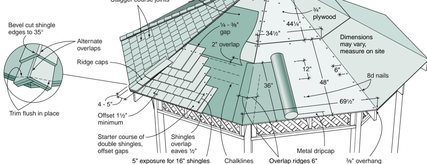
**Shingles over plywood sheathing** Each two-piece section of sheathing is cut from one 4x8 sheet of plywood. Use 8d nails to install the roof panels, allowing ⅛-inch expansion gaps at the joints. Attach metal drip caps at the eaves.
