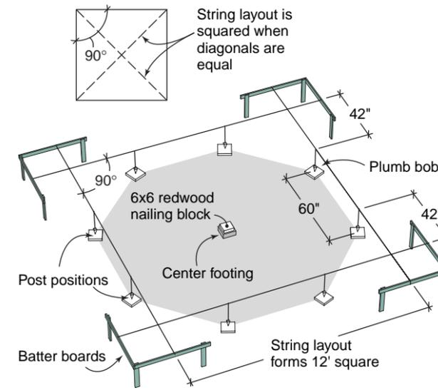
**Layout** If you think of an octagon as a square with its corners cut off, you'll realize how simple the shape truly is. A common measurement and trim angle to remember throughout the layout and construction process is  $22\frac{1}{2}^\circ$ . The key, as with any project, is both careful planning and precise measurement.
