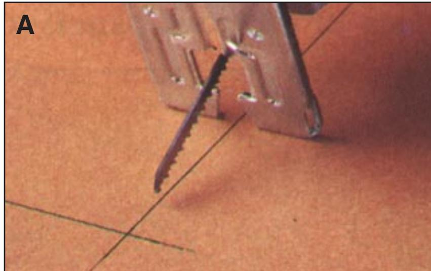
To start the plunge cut for the window, position the jigsaw on the plywood with the blade not touching the wood but centered over the cutline.
