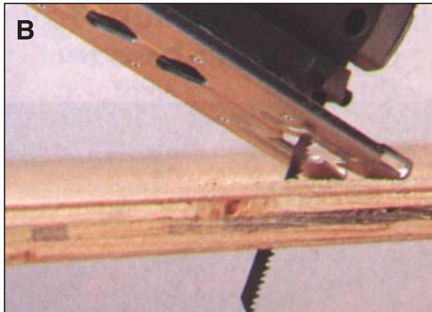
Turn on the saw, and lower the blade into the wood, causing the reciprocating blade to cut through the plywood at the marked cutline.
