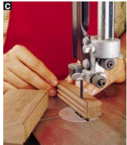
C After separating the upper block from the beads, mark a cutline and bandsaw a \frac{3}{16} "-thick blank for part C.
