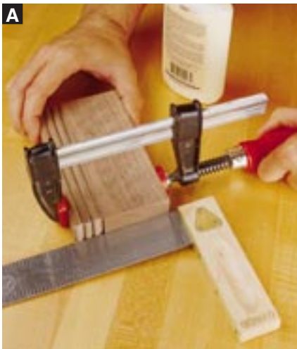
A Glue and clamp the beaded parts and the upper block together, keeping the ends and edges flush.
