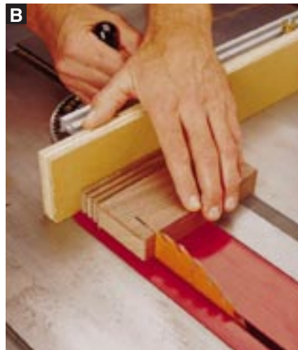
B An extension attached to your miter gauge eliminates chip-out when cutting the sides (B) from the glued-up blank.
