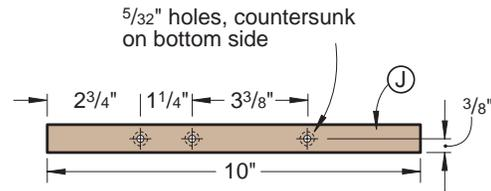
**Note:** Size width and thickness to fit miter-gauge slots on your table saw.
