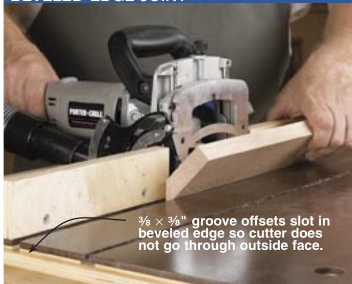
Hold the part against the fixed fences with the beveled edge in the  $\frac{3}{8} \times \frac{3}{8}$ " groove. This offsets the slot toward the inside face.
