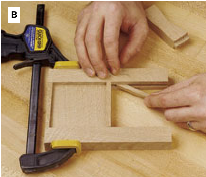
Glue and clamp a long filler in each stile's groove, sliding it behind the bottom face-trim piece and tight against the face. Remove any squeeze-out.
