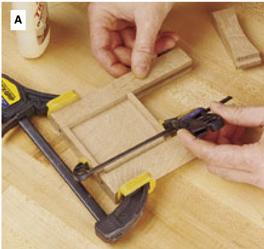
With the face (B) clamped (no glue) between the stiles (A), glue and clamp the face trim (C) to the face's top and bottom edges.
