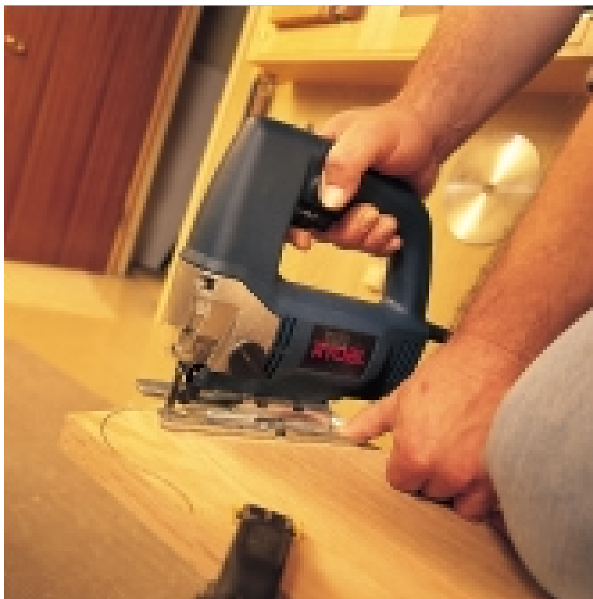
Gary uses a Ryobi JS048 jigsaw to cut the corner shape on each leaf. The piece is securely clamped, and Gary uses his thumb on the base plate to guide the saw
