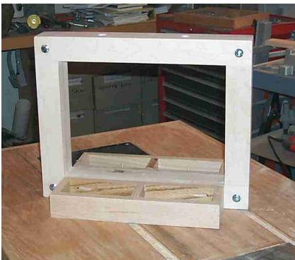
*Small "wings" to support the lower platen are secured to the sides of the main frame with glue and screws.*
