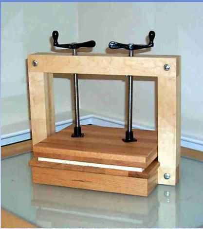
This design uses veneer press screws commonly available from mail-order suppliers. The dimensions were set by what was in the scrap bin and the 12 inch press screws I had on hand. The press could as easily be built with a single press screw, but I felt the double screws would spread the pressure a bit more evenly. I was aiming for a capacity of 11X14 inches, as that covered about 95 percent of my needs and wouldn't pose much of a storage problem.
