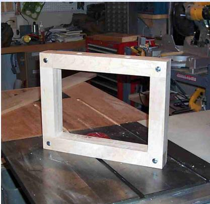
*The main frame is laminated from three layers of hardwood, glued and bolted together.*
