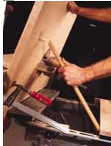
**3** Once the tabletop is hinged to the Workmate's front board, it's easy to locate the the positions for the prop stick and stick bracket. Note the shop-made replacement board for the Workmate top.
