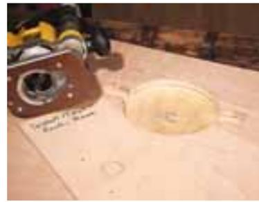
**1** A larger base for the router was the ticket for bridging the open areas left by routing out the plywood for the router's base. It was later used as a small circle cutting jig for the tabletop and plastic inserts. Use the same cutter and it's easy to keep track of dimensions for cutting inside or outside circles.
