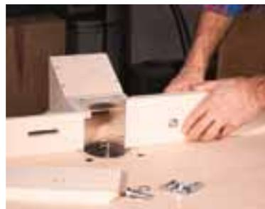
**7** Attach the fence faces using  $\frac{3}{8}$ " roundhead machine screws, a star washer, flat washer and wing nut. I tried using hex-head bolts but switched to screws because a screwdriver can be used and makes a more secure attachment with less trouble.
