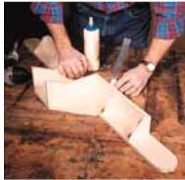
**4** As you assemble the fence, make sure it is square along its length. Be sure and check it again after it is clamped up.
