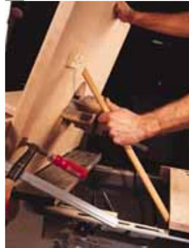
**3** Once the tabletop is hinged to the Workmate's front board, it's easy to locate the the positions for the prop stick and stick bracket. Note the shop-made replacement board for the Workmate top.
