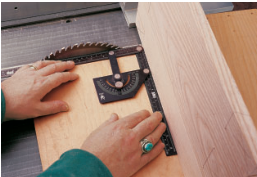
Photo G: To cut the outside tenon shoulders, reposition the box fence 3 degrees to the blade.
