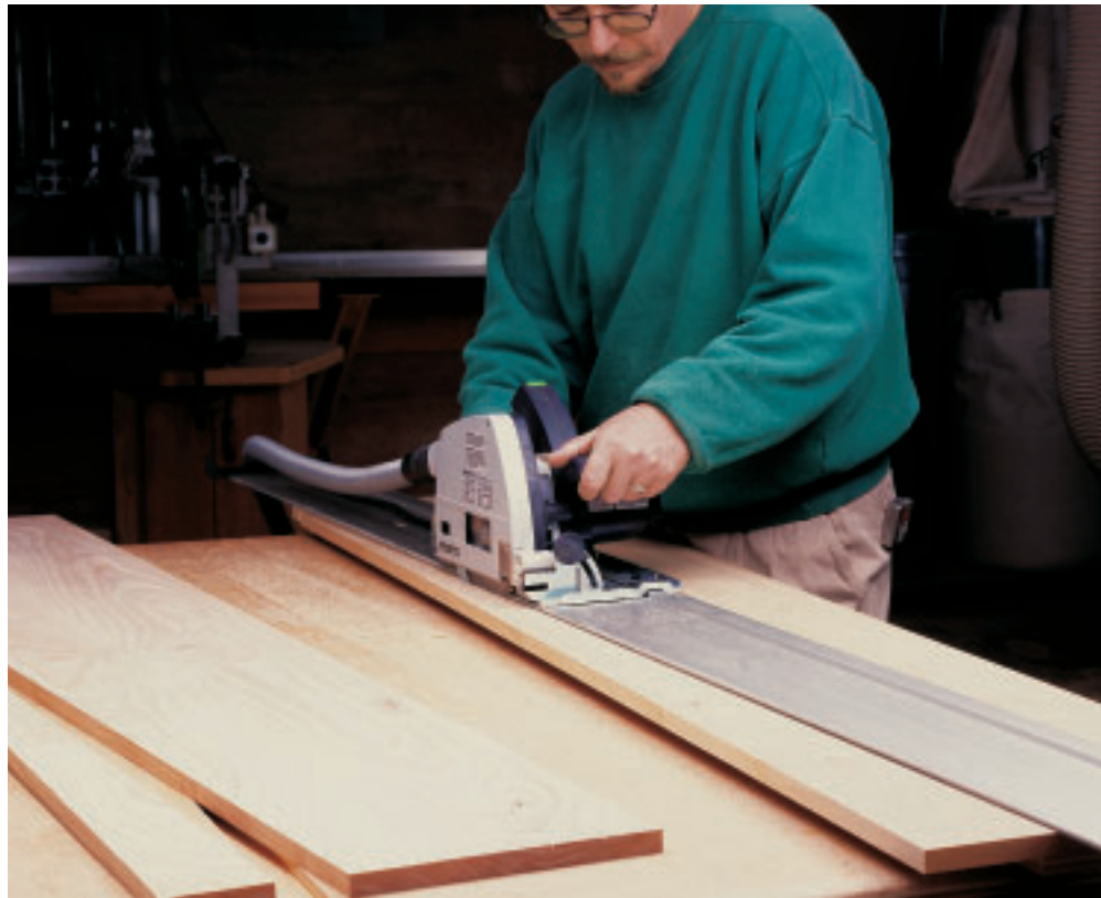
Photo B: A circular saw and straightedge guide make cutting the tapers on the sides a cinch.
