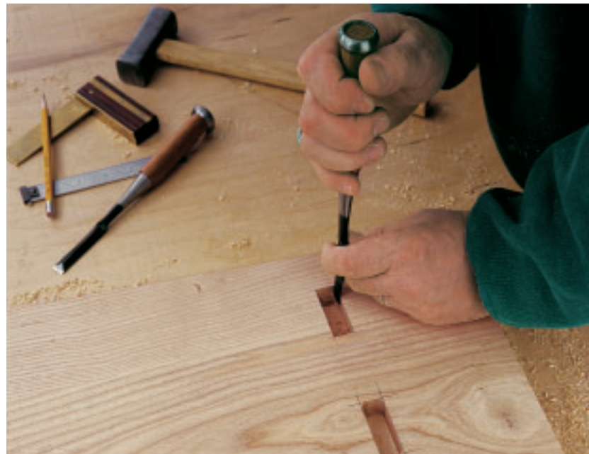
Photo E: Square up the routed mortises with a sharp chisel.
