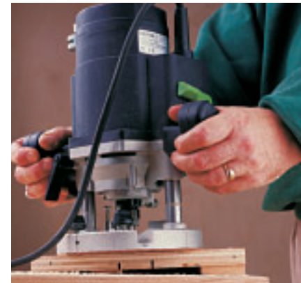
Photo D: The mortising jig tilts the router 3 degrees and cuts the mortise walls at the same angle.
