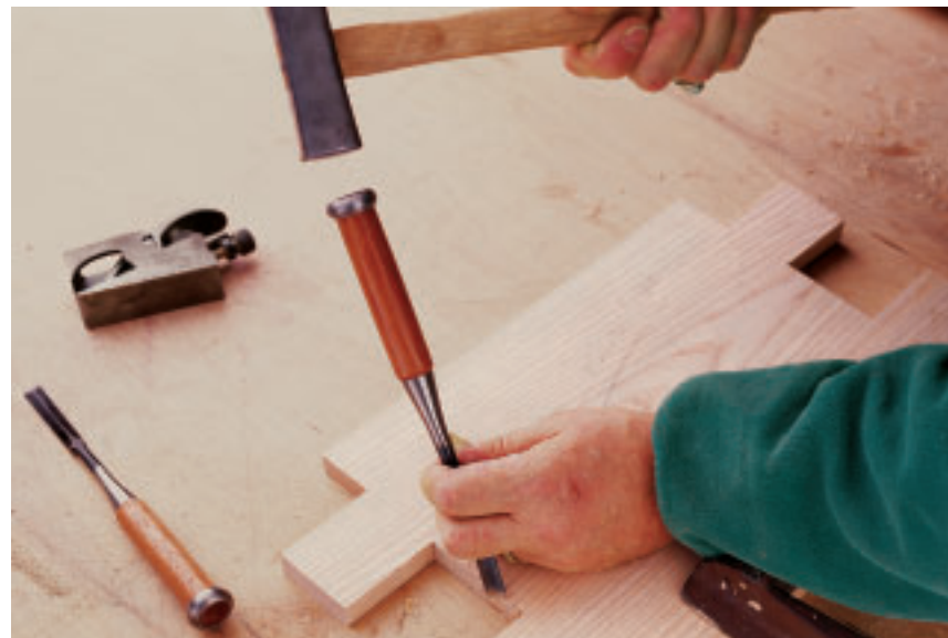
Photo H: Clean up the jigsaw cut with a chisel.
