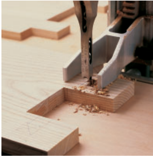
Photo I: A hollow-chisel mortiser with a \frac{3}{8} -in. bit is fast and accurate for cutting the mortises for the wedge.
