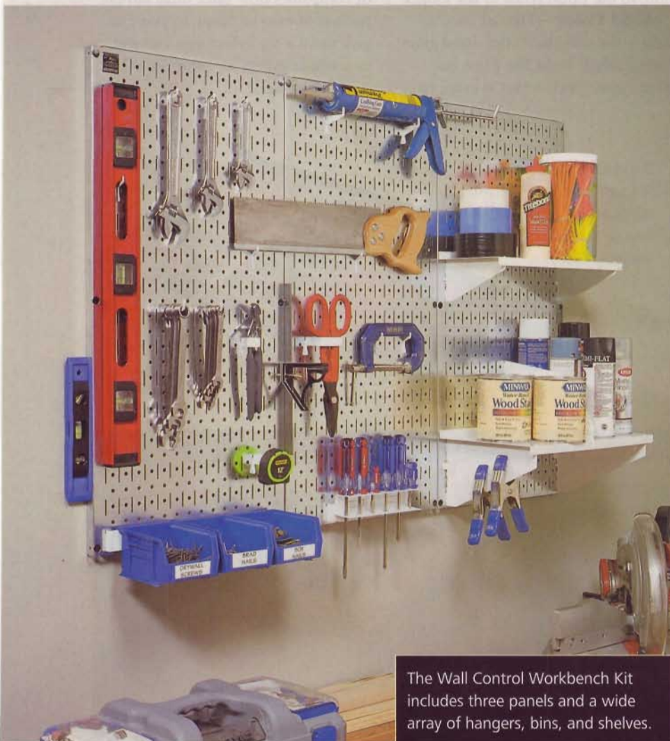
The slot-mount hangers that come with the Wall Control panels use rubber O-rings for a rattle-free fit.
