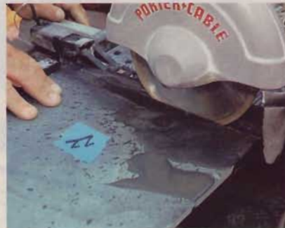
2] A tile saw uses a diamond-grit wheel and water to cut smoothly through stone tiles without a lot of dust.
