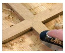
**Payday.** Flush the surfaces of the completed joints with a sharp block plane, and take a moment to feel proud. Then get back to work; there are a bunch of these.
