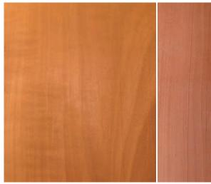
**Raking is revealing.** Here we see two photos of the same board. In the one on the left, light is aimed directly at the board, obscuring the surface. In the one on the right, a raking light (light coming in at a low angle) reveals surface imperfections.
