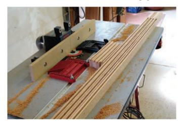
A furrow for your panel. A powerfully quick method to form grooves for the plywood panels is a sharp . <sup>1</sup>/4" router bit and a nice router table setup.
