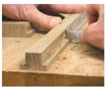
**Run in reverse.** The back of a chisel makes a great scraper, just the ticket for cleaning out the corner of rabbets.
