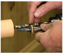
A matter of judgment. The depth of the hole should be somewhat deeper than the length of the tang. The end will be trimmed to fit.
