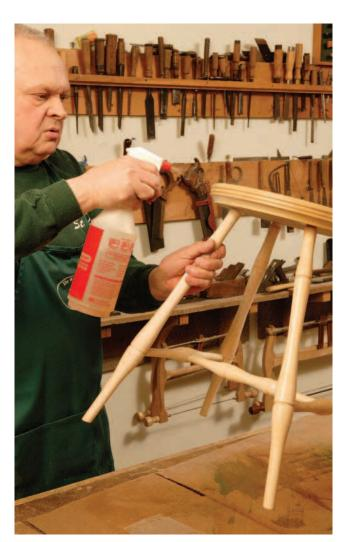
**Spray.** Moisten your workpiece surface thoroughly (but not so much that the water runs) to raise the grain.
