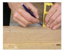
**Better than numbers.** A combination square does an excellent job of laying out repeating spaces, in this case the openings in the door.
