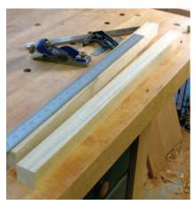
Connect the dots. With the start of the taper drawn on one face, rotate the leg, mark the amount of the taper at the foot of the leg then connect the lines to show the total taper.
