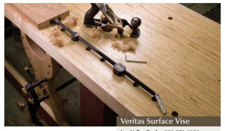
it mounts on the surface of your bench, it's going to stick up and could interfere with your tools, especially the soles of long hand-
