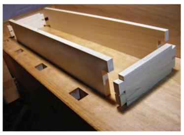
Till parts. Till components cut with the ends already dovetailed.
