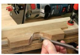
**Double duty.** This jig guides the bearing on a flush-trim router bit, then is used to guide a chisel to pare into the mitered corners.
