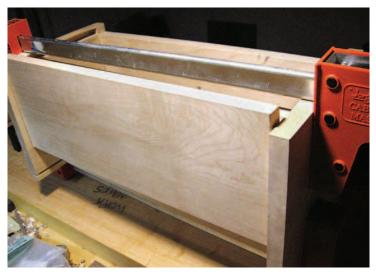
**Dado work ahead.** You can see the lid stops at this point; I will disassemble the tool chest and lengthen the 'L' shaped dado so, when open, the lid will be ush with the top of the sides.
