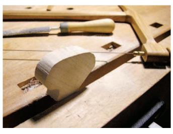
Trace. Here, I'm shaping one of two cleats that will become back saw holders. These were simply traced from my hand saws and cut out.
