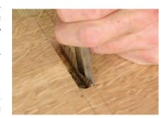
**And swing it.** Keep the back of the chisel pressed against the routed edge of the mortise and carefully rotate the edge into the corner.
