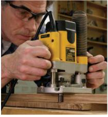
**Under control.** Cut the tenon shoulders first, using a straightedge and a bearing-guided router bit. Adjust the depth of cut in small increments to achieve the proper thickness.
