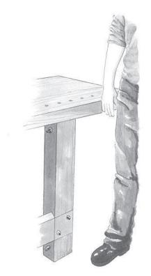
The general rule for measuring the ideal bench height for hand-tool use is to stand upright alongside the bench, with your arms hanging straight down. The top of the bench should be about level with the knuckle joint of your pinky finger. That height is a good compromise between using the bench for planing and using the bench for sawing dovetails and the like.
