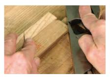
**Complex geometry.** Test the fit often while fitting the miters. Trimming one edge will lengthen or shorten an adjacent edge as well.
