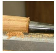
Room for compression. A small gap between the socket and the shoulder will keep the handle tight over time.
