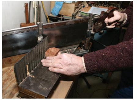
**Perimiter.** I use a miter box and saw to safely and accurately cut out the head, but a scrollsaw or backsaw also would work.
