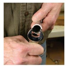
**An open-ended question.** Use a wrench to gauge the large diameter of the socket.
