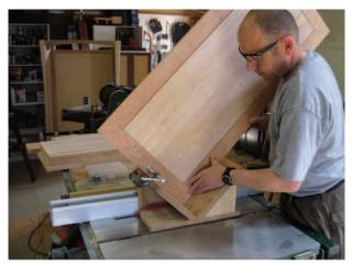
**Jig it up.** Splines reinforce the mitered corners on the top unit. To cut the slots, it's best to make a jig that slips over your table saw fence as it holds your assembly at a 45° angle.
