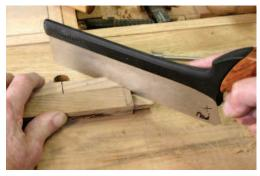
**Miters, too.** 45° cuts in the fence guide the saw to cut the short miters. Preserve the line at this point, and work down to it while fitting.
