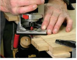
This will work. Remove the bulk of the waste between the tenons with a jigsaw or coping saw. Then clamp a straightedge between the two tenons and use a router to make a clean, straight cut.
