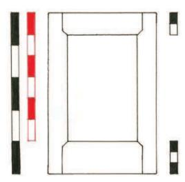
Frame-and-panel door frames. On these two examples, the top and bottom rails are weighted differently. At first impulse, which looks right?
