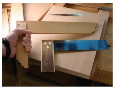
A handle for hands. The narrower and longer stock of a wooden square makes it easier to hold and more accurate in use.
