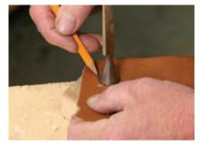
**Drill then trim.** Use a twist drill to make a hole in the leather, then trace around the taper before cutting the disc with scissors.
