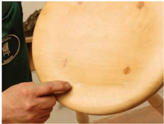
**Glue alert.** In addition to raising the grain, the water also highlights areas from which glue needs to be removed before painting.
