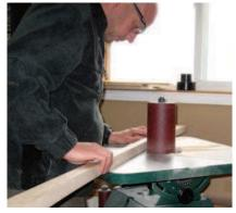
Shape a gentle curve. Use a spindle sander to shape one leg exactly to your layout line.
