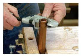
The right tool. An inexpensive pipe cutter makes a cut quickly and leaves smooth edges on the copper ferrule.
