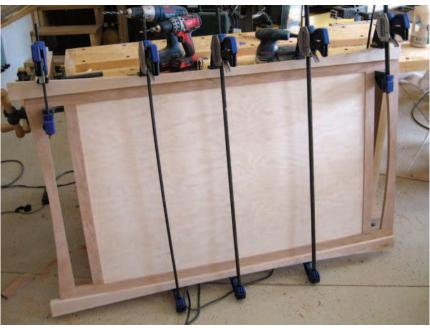
**A strong hold.** Long-grain-to-long-grain joints have plenty of hold once you get things located. A few well-placed dowels work wonders to align and reinforce the joint.
