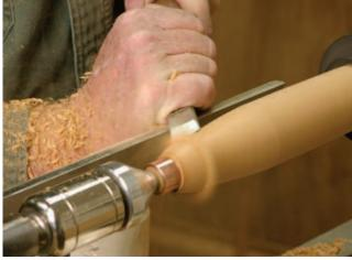
Shaping up. As the handle takes shape, carefully taper the end of the handle to the edge of the ferrule.
