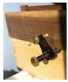
Field jointing. With the surface clamp in one of the front holes and a 3/4" dowel in the other, I can edge joint a board up to 24" long!
