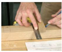
**The real thing.** A scrap of muntin stock is held against the square to mark the stiles. This speeds the process and ensures accuracy.
