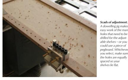
A dowelling jig makes easy work of the many holes that need to be drilled for the adjustable shelves - or you could use a piece of pegboard. Whichever you select, make sure the holes are equally spaced so your shelves lie flat.
