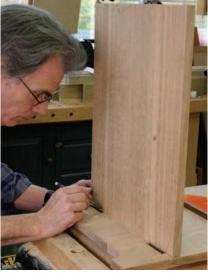
Make your mark. Wait until the mortises are completed to lay out the tenons on the cabinet top and bottom. Mark the locations from existing edges.
