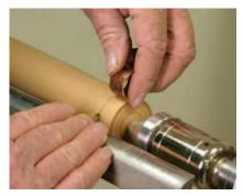
Be direct. The cone center fits in the tang hole. keeping the work centered. Use the ferrule to gauge the length of the turned tenon.
