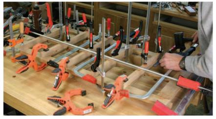
**You need more clamps.** The mitered lap joints in the center of the assembly will tend to pop up as clamp pressure is applied to the ends. Battens across the faces hold things together.
