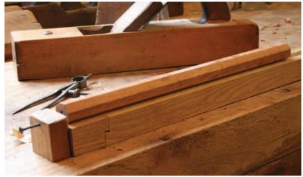
**Octagon.** Begin by making the bar stock. You can turn it round to  $^{3}/_{4}$ " on a lathe, or use a spoke-shave to make an octagon, then true it with a  $^{3}/_{8}$ " hollow plane to  $^{3}/_{4}$ " diameter. Or, use a length of dowel
