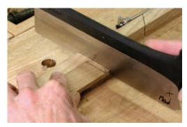
**Use the fence.** Saw cuts in the fence of the bench hook guide the saw to make clean and accurate cuts.
