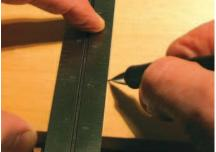
**Shadow play.** These photos show the value of moveable lighting. In the shot on the left, the marked line is invisible, hidden by the shadows of the square's blade and my hand. In the photo on the right, you can see the marked line.
