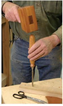
A dab will do ya. A small amount of epoxy in the hole will keep the tang connected. Place the leather over the tang and drive the handle on.
