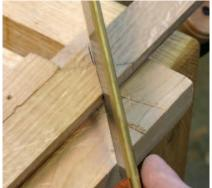
**On the right side.** For the points of the miters to meet, the saw cuts must be on opposite sides of the lines on each side of the mullion.
