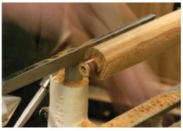
Almost home. Make a slight taper on the tenon, then test the fit of the ferrule.
