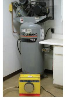
Compressors. Compressors big enough to supply spray guns sometimes come with wheels but are otherwise not easily portable. Turbines are small and fairly light so they are very portable. This compressor is 5 hp, produces 15 CFM and has a 60-gallon tank. The turbine is three stage – the smallest that atomizes adequately.
