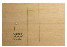
Vernier acuity. This photo illustrates vernier acuity. The pair of lines on the left were marked with the ends of the pieces aligned. The pair on the right were marked with one of the boards offset with a .002" shim. The pieces were then realigned and the photo taken. Thus, the lines on the right show an offset of .002", which, remarkably, is fairly easy to see.
