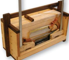
**Small but mighty.** This tool chest will hold a surprising amount of hand tools and features some handy "on the road" benefits. In the "open" picture above, you can see the backsaw holders, the shooting board on top and the cam clamps that are used to secure the chest to any surface.
