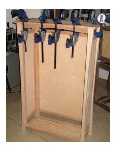
**No nails needed.** The frame of the top is glued to the front and back panels while the top's panel is dowelled to the cabinet sides. Get your clamps ready.
