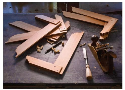
**Built-in accuracy.** Wooden try squares are more than accurate enough for woodworking. Plus they have other advantages – less weight and more reach.
