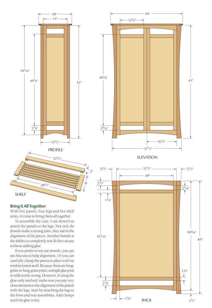
The next step is to attach the sides to the front and rear assemblies and insert the bottom. If you're using dowels, position them in such a way that at least one dowel passes through the tenon in the front assembly. This way the dowel not only serves to hold the side panels in position, but it also creates a pegged-tenon joint in the front assembly. Test-fit the front and rear assemblies with the side panels.
