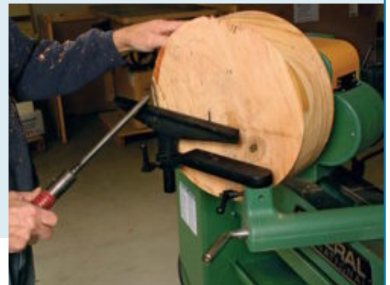
A questionable outrigger. An extension bar for the General tool rest is designed for outboard turning. But it flexes considerably and is a weak spot.
