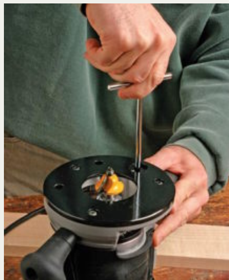
Ready for a router table. The Milwaukee allows for height adjustment and bit changes from above using an included T-handle wrench.
