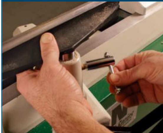
Skimpy. The Rikon's tool rest is nicely designed, but it is held in place with a small locking lever that's uncomfortable to hold.
