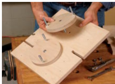
Attach the circles. With outside bolts in place, secure the circles to the front plate with 3/8-in. bolts through the center holes. Hand-tighten double nuts over the washers and lock the washers.
