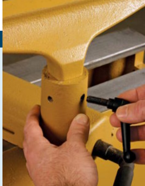
Versatile. The locking lever on the Powermatic and the Jet fits in one of three holes. You can move it to keep it clear of the tools.
