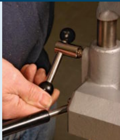
Comfy. The two Nova lathes have a substantial locking lever for the tool rest that's easy on the hands.
