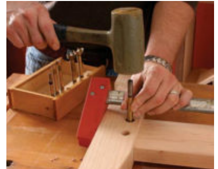
Mark the tenon. With the joint re-assembled and clamped together, mark the center point of the hole. An easy way to do this is to insert a Forstner bit into the hole and tap lightly.
