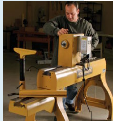
Slider. The Powermatic headstock slides the length of the bed. A bed extension and an accessory for the tool rest give it very useful outboard-turning capability.
