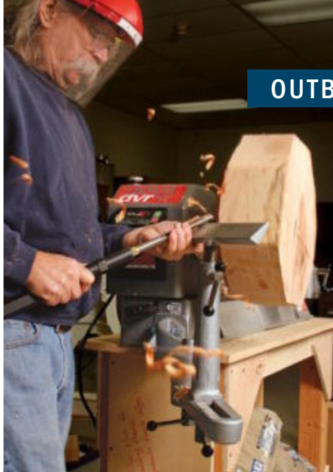
A substantial outrigger. The Nova models come with a hefty, well-made accessory to hold the tool rest for outboard turning.
