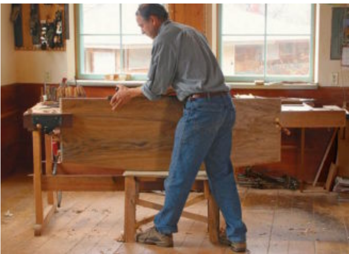
Steady a wide panel. A sawhorse provides support underneath, with the opposite end clamped to the bench apron.
