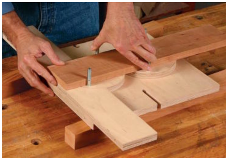
Attach the circles. With outside bolts in place, secure the circles to the front plate with 3/8-in. bolts through the center holes. Hand-tighten double nuts over the washers and lock the washers.
