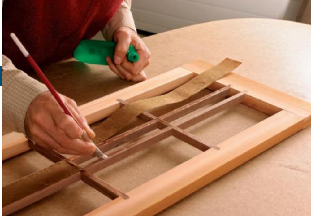
Glue on the paper. Apply a thin coat of rice paste to the back of the frame and dividers. You cover a larger area with small pieces of paper by overlapping joints at a divider.
