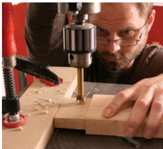
Drill through the tenon. Align the tip of the Forstner bit so that it engages the crosshairs marked previously. If you need to drill multiple holes, using a fence helps ensure consistency.
