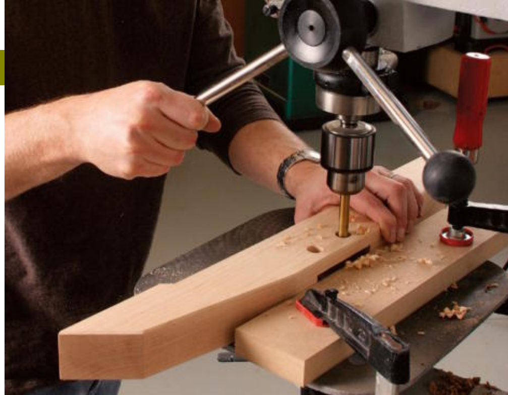
Drill the mortised piece. Go through one side and partway into the other. Use a Forstner bit for a clean cut.
