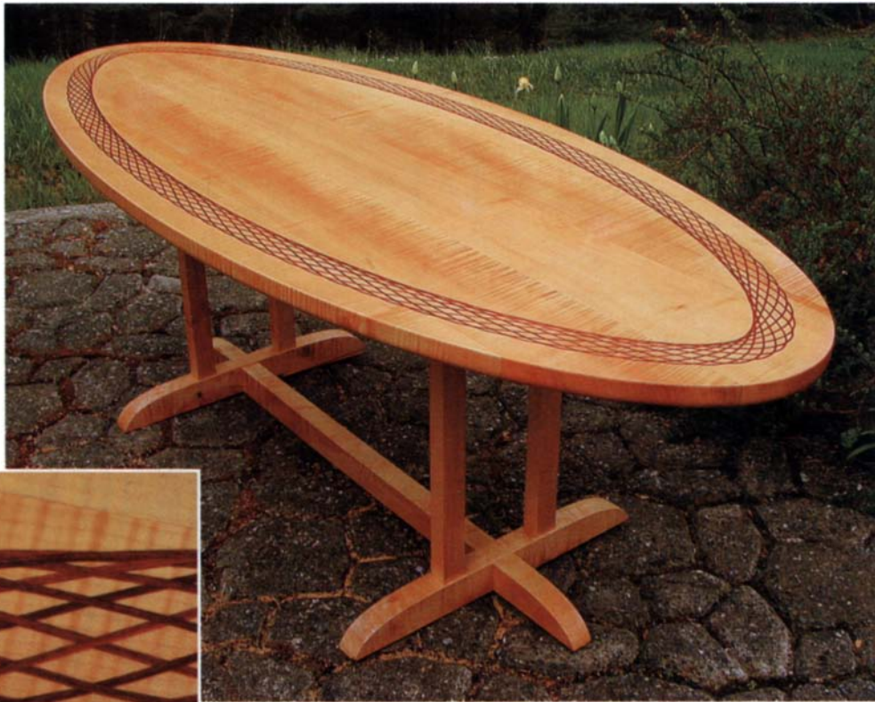
An intriguing web. The purpleheart inlay in this western curly maple table was made using a router as a form of spirograph. A gear attached to the router base runs in a chain on a jig just larger than the tabletop.
