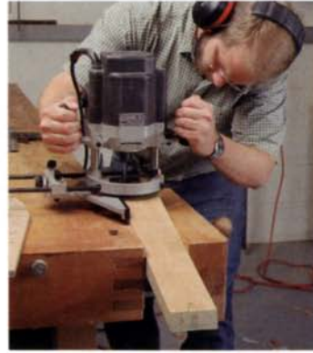
Cut the mortises for both legs at the same time. Use a router and edge guide, and clamp the legs together to provide a larger bearing surface for the baseplate.
