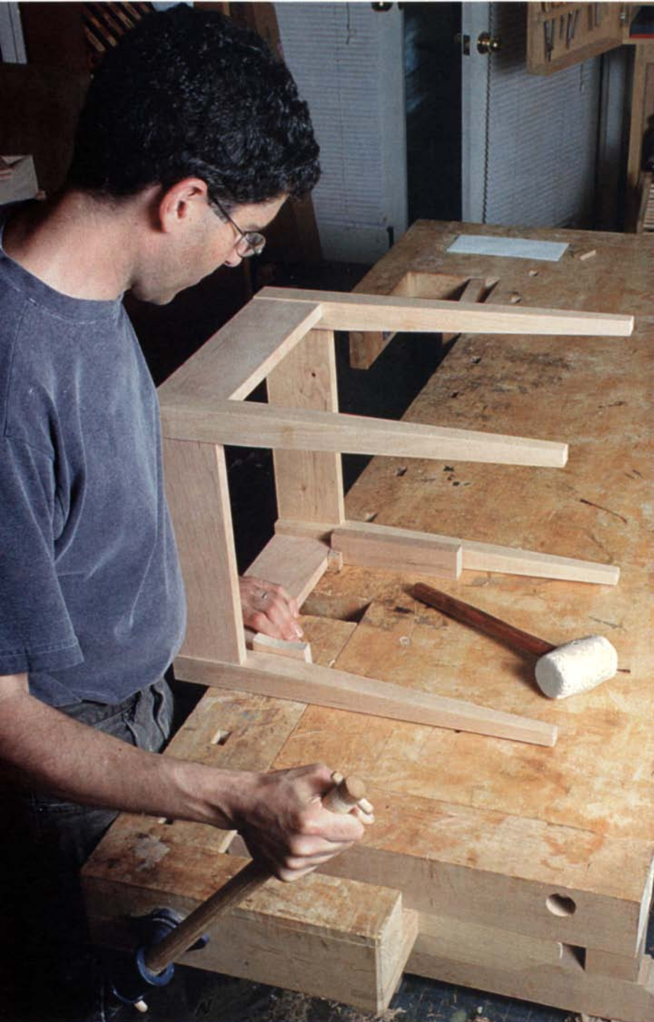
Stubborn joints cause many problems during dry-fitting or final glue-up. Working from opposite sides a little at a time, use a bench vise to pull apart tight joints.
