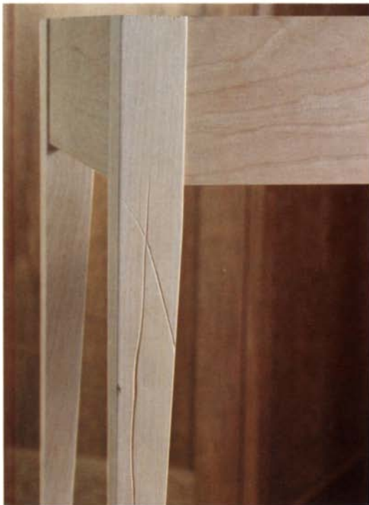
Don't give up on a piece, even if the damage seems severe. Shopmade veneer can be used to cover up cosmetic damage.
