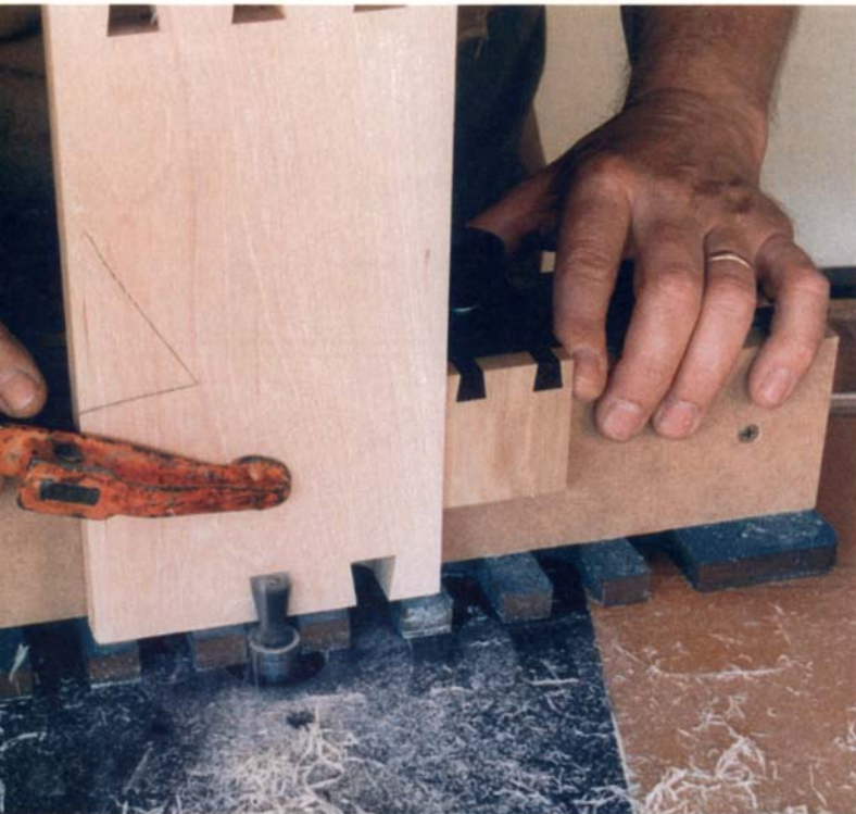
The latest jig for through-dovetails. Teamed with a router table, the Gifkins dovetail jig is easy to set up and use.
