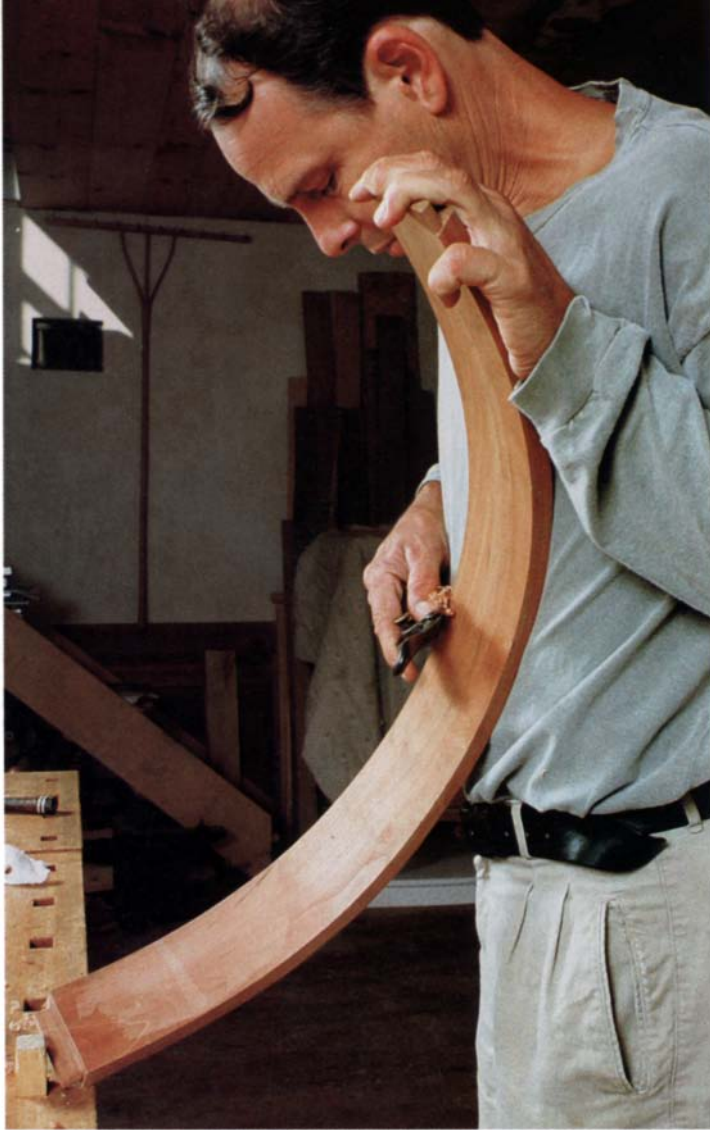
Spokeshaves are good for concave curves. Lightweight enough to use with one hand, this Stanley No. 54 has an adjustable mouth to help control the depth of the cut.
