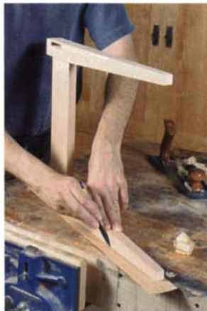
Align the grain of the veneer. Trace the shape using the part to be fixed, and cut it slightly oversized.
