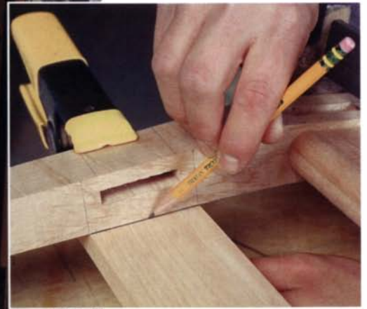
Mark tenon shoulders from the assembled back. With the rear seat rail clamped in place, make sure the assembly is square, then clamp the crest and lower back rails into place. The tenon shoulders, which are angled slightly to match the leg tapers, can be marked directly off the leg.
