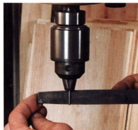
File down the alignment pin. If the alignment pin (a 6d nail) is to slip smoothly into a mating hole, it must be filed down a bit as it spins in the drill press.
