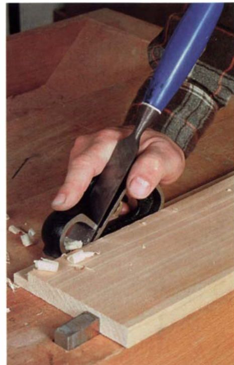
Transform a chisel into a plane. Once secured in the plane, a chisel becomes a sturdy, economical shoulder or rabbet plane.
