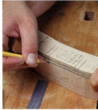
A story stick saves time. Layout is simplified by marking out all mortises directly off the rear-leg template.
