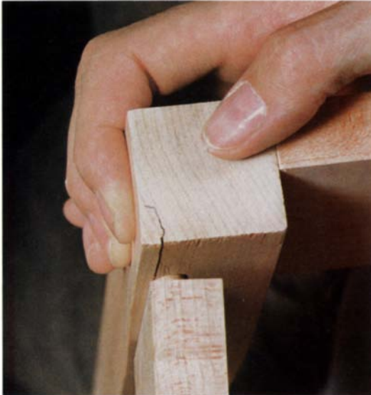
Overly tight joints may crack when fit together. After disassembly, pare the tenon for a looser fit.
