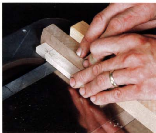
Mark and cut. After adding a pair of index marks, the tablesaw is used to cut off the short-block portion of the tool.
