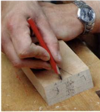
Mark out the legs. Tick marks on the front of the legs indicate which faces will be tapered after the mortises are cut.
