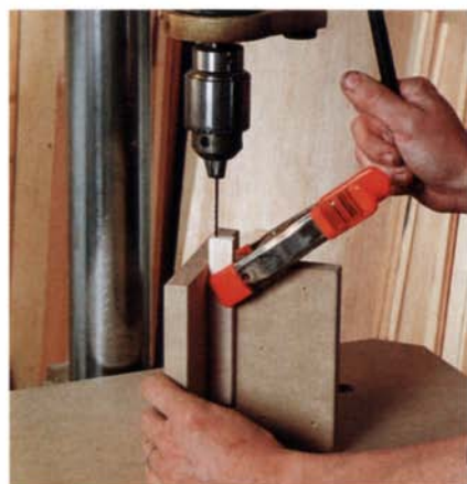
Drill the alignment-pin hole. Cut a hardwood strip to size, then drill a hole in the end for the alignment pin. A T-shaped fixture keeps the strip square to the table.
