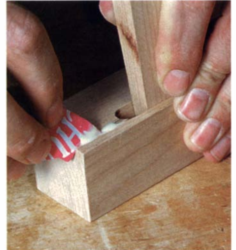
Get glue deep into the crack for a good repair. A piece from a snack-food package or candy wrapper can be used to force glue into a crack.
