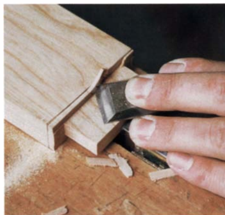
Cutting angled shoulders. After the bulk of the tenon has been cut on the router table, backsaw to the angled shoulder line. Quick work with a chisel trims away the excess.
