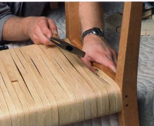
Ending the warp. When you reach the side rail, pull the reed underneath the seat and use a #3 upholsterer's tack to secure it to the seat rail.
