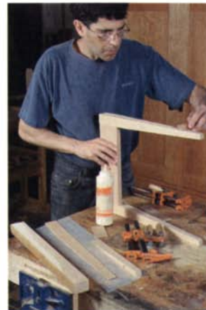
Glue the patch in place. Use cauls to protect the stock from the jaws of the clamps.
