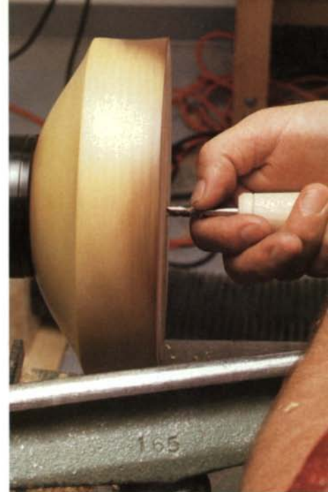
Push the drill bit into the hole left by the screw chuck. A depth drill is simply a \frac{1}{4} -in. or \frac{3}{8} -in. bit jammed into a shop-made handle.
