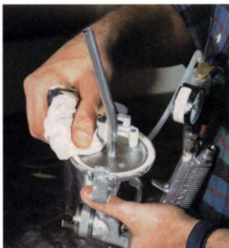
Clean the gasket. The gasket needs to be free of debris; otherwise, the gun will not seal properly and will leak when tipped.
