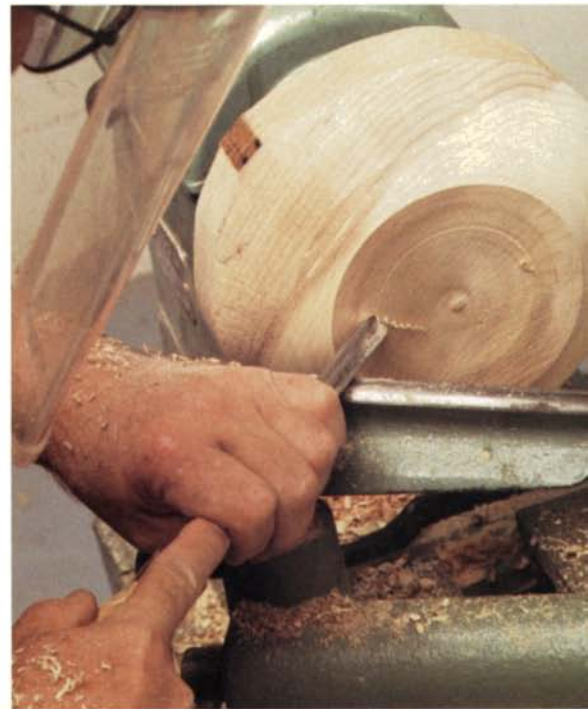
True the rest of the base. Rotate the gouge so that the flute faces outward, and take a light shear cut from the rim to the center.
