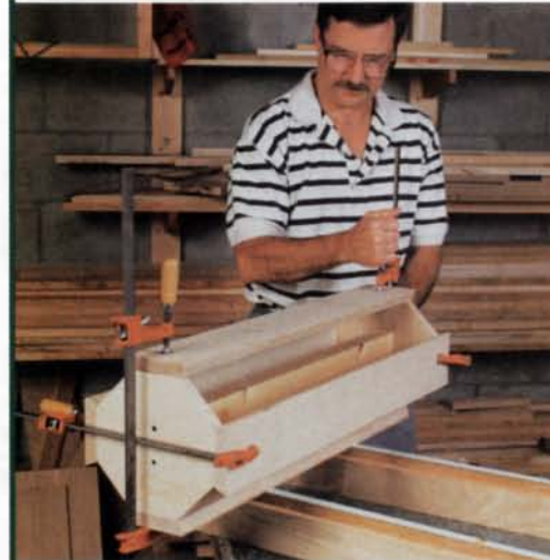
Clamp four sides. Every other side of the column is clamped to the holding fixture. The remaining sides float into position.
