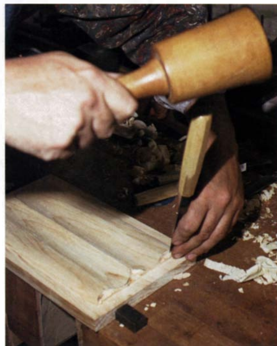
Retrace your steps. After shaping the top surface of the panel, retrace the template (above) and then chop the ends to shape (right).
