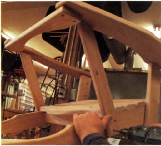
Arm supports butt into arms and rest against middle stretcher. The curved stretcher holds the arms apart at the proper distance. The chair's back splats will be screwed to the stretcher.
