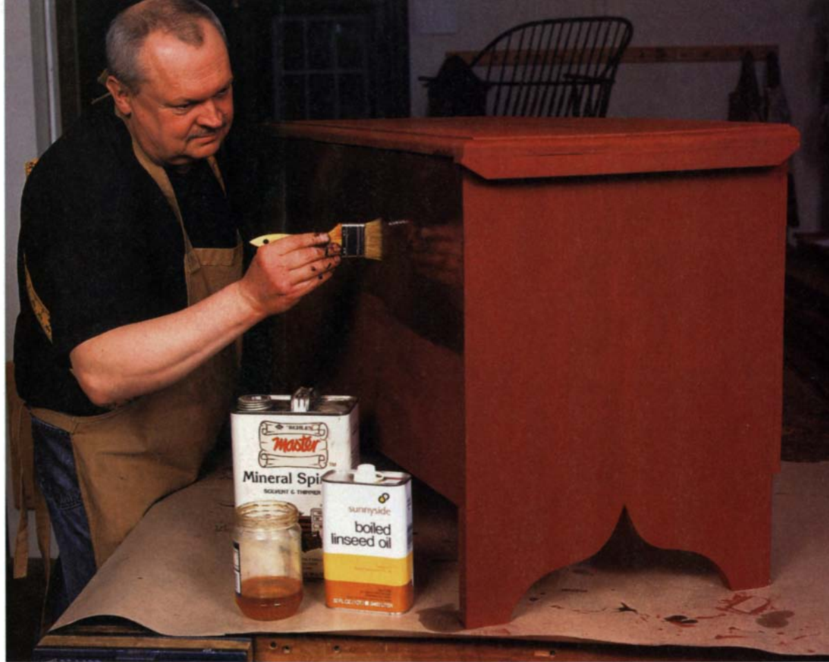
Thinned linseed oil over flat paint. A mixture of five parts boiled linseed oil and one part paint thinner is brushed on as a final coat. Excess is wiped away with a lint-free rag.
