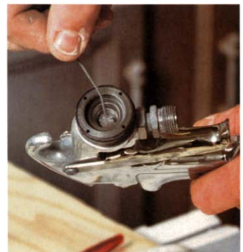
Remove the air cap and fluid nozzle. The inside of the gun is best cleaned with a skinny brush soaked in lacquer thinner.
