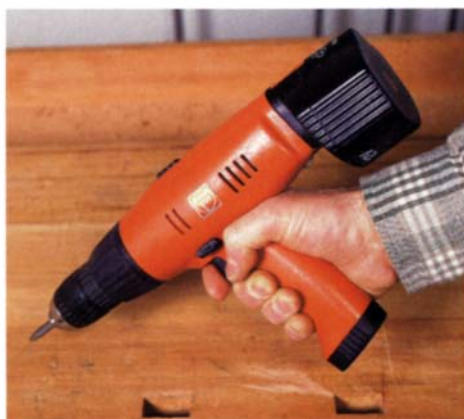
Fein drill gets into tight quarters. The battery on this 12-volt drill can be attached either to the base of the handle (right) or to the back of the motor (left).
