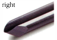
Spindle gouge with a fingernail grind
