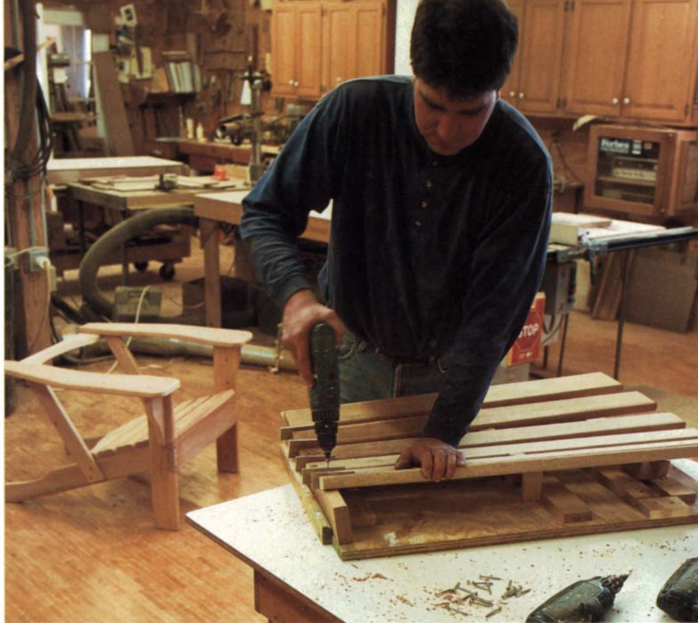
Building the back. A jig holds the bottom and upper back stretchers while the author screws on the back splats. He uses spacer blocks at the bottom and middle of the splats.
