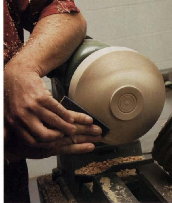
Hand-sand the profile. Keep your hands on the lower half of the bowl; the motor cover makes a good arm rest.
