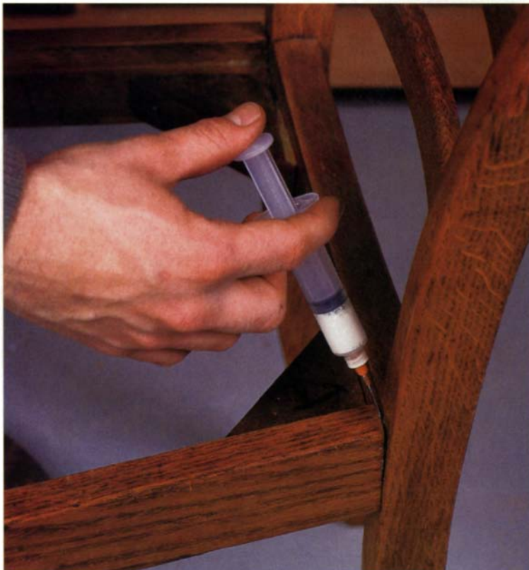
A quick fix. Chair Doctor glue injected into loose, squeaky joints first swells the wood fibers, then bonds them tightly in place.
