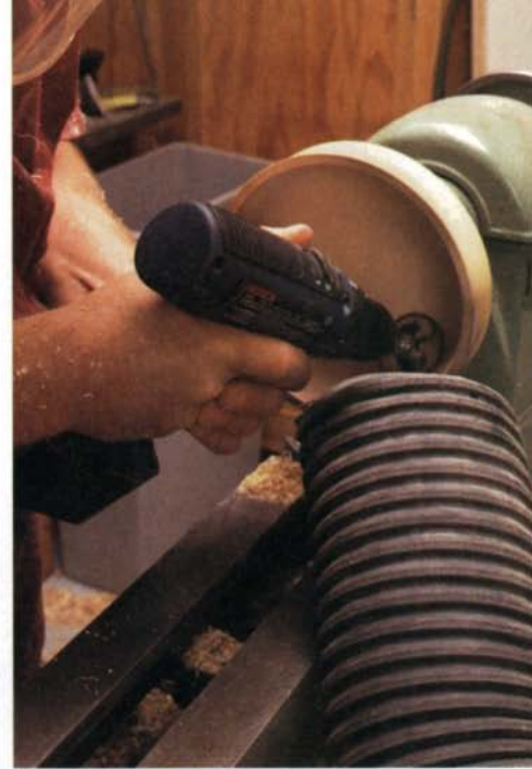
A faster way to sand. Power-sand using flexible sanding discs in a portable drill. Sand from 100 grit to 380 grit.
