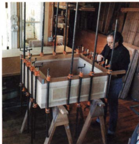
Cauling all clamps. Strips of wood, called cauls, are placed between the clamps and the face frame to prevent marring. The author uses numerous clamps when gluing the face frame to the cabinet's plywood carcass.
