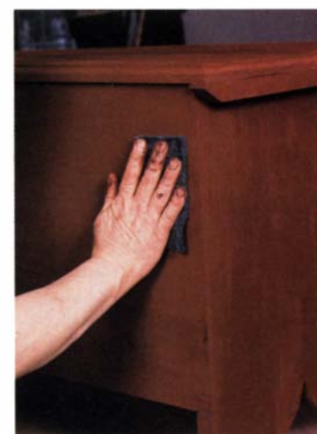
Excess paint turns to dust as it dries. A gray Scotch-Brite nylon pad knocks off any rough spots in the second coat.
