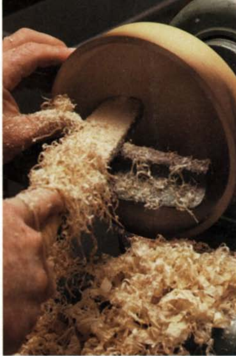
Smooth the interior. Use a scraper to clean up tool marks and tearout.
