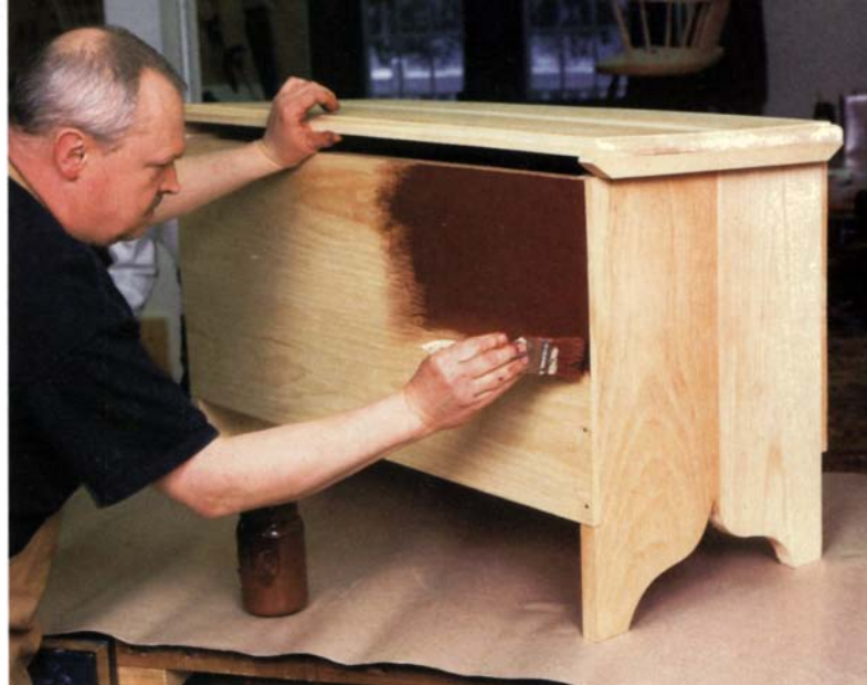
A cheap brush is all you need. A natural bristle brush—bought for $1 at the local hardware store—is used to apply all coats.
