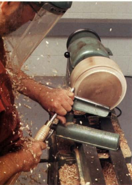
The outside profile of the bowl is shaped first. Begin by taking material off the corner. Don't worry about tool marks at this point; just rough out the shape with a 1/2-in. spindle gouge.
