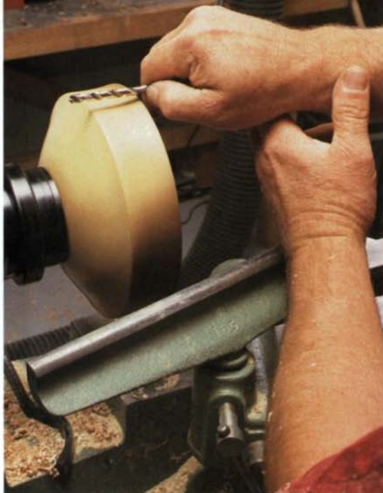
Measure the depth of the bowl. Leave about \frac{1}{2} -in. thickness in the base.
