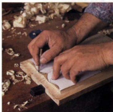
Retrace your steps. After shaping the top surface of the panel, retrace the template (above) and then chop the ends to shape (right).
