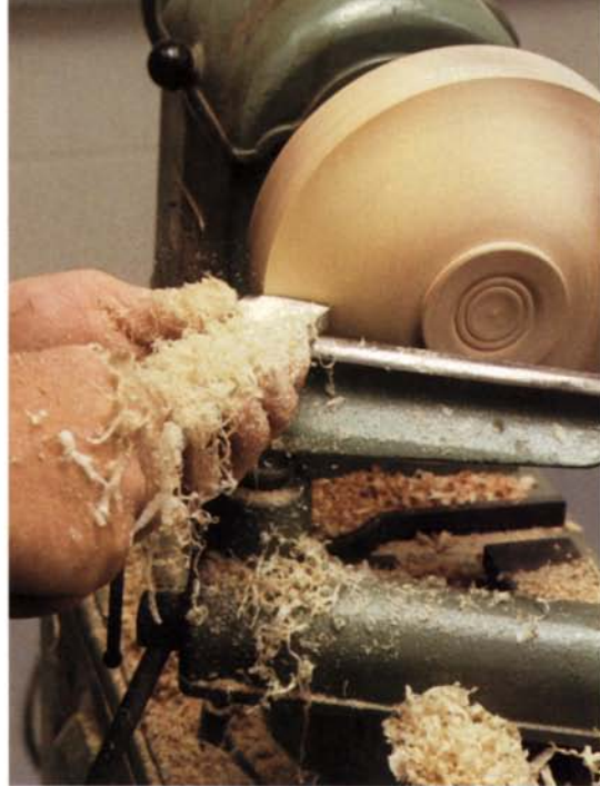
Finish shaping the profile. Working from the base of the bowl to the top, take a series of shear cuts with a gouge (left). Clean up using a scraper (right).
