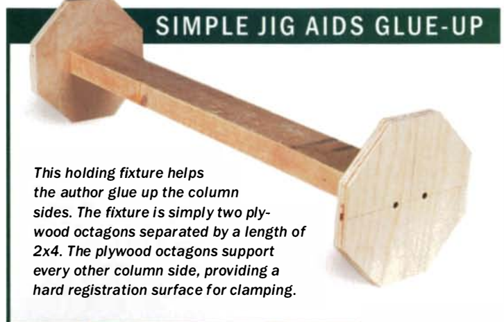
Clamp four sides. Every other side of the column is clamped to the holding fixture. The remaining sides float into position.
