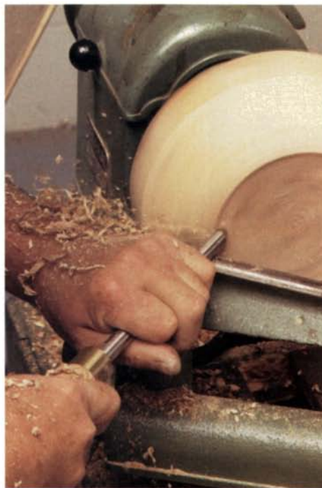
True the edge of the base. Have the gouge on its side with the flute facing the base. Squeeze the edge into the wood. When the ticking noise stops, you have a trued edge.
