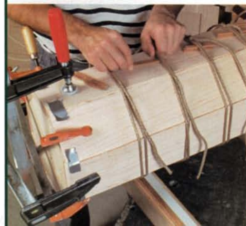
Add more clamps and tie it off. The combination of clamps and rope holds the assembly solidly together.
