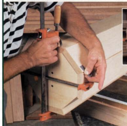
Add tape. The tape temporarily holds the non-clamped sides in place.
