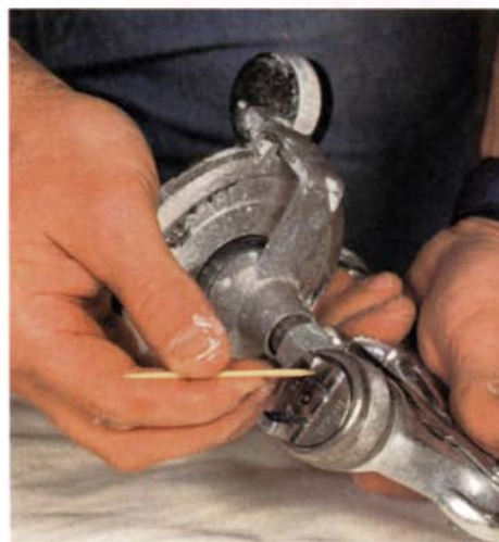
Clear the air passages. Wood toothpicks won't damage the precisely machined air-cap orifices, which can get clogged with finish.
