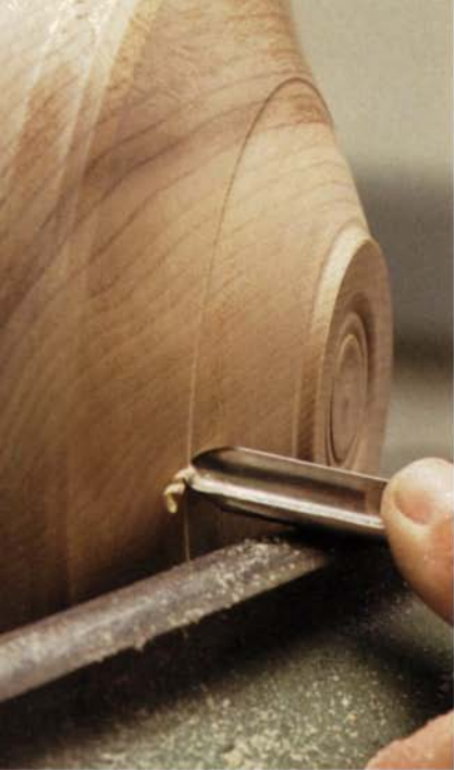
Finish shaping the profile. Working from the base of the bowl to the top, take a series of shear cuts with a gouge (left). Clean up using a scraper (right).
