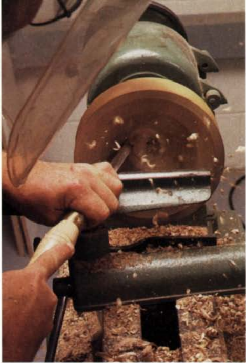
Rough out the inside. Use a deep-fluted \frac{1}{2} -in. bowl gouge held at about 45^\circ and work from the rim to the center.
