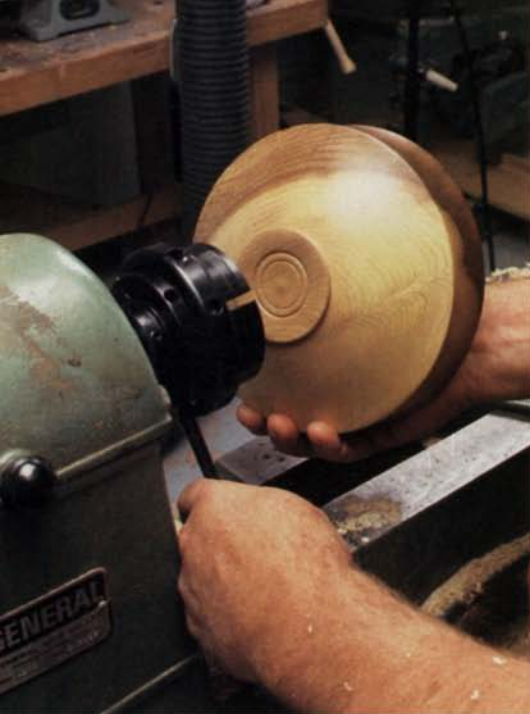
Rechuck the bowl by its foot. A four-jawed chuck with step jaws won't mar the workpiece.
