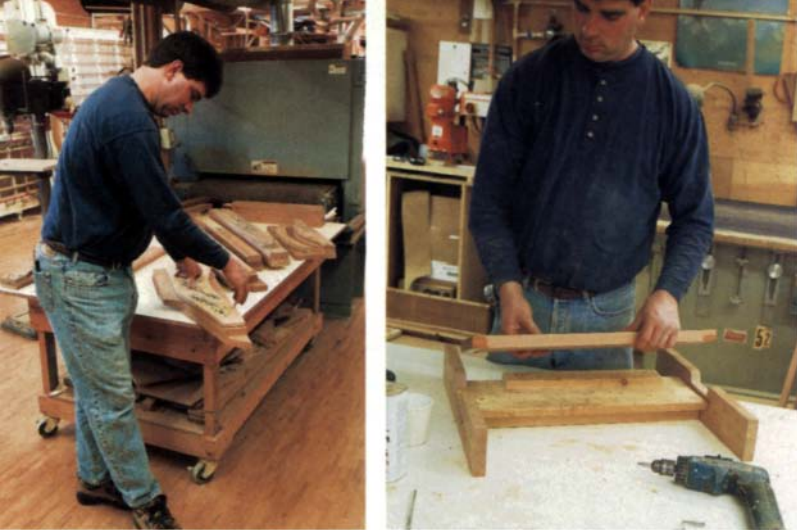
Front stretcher is let into the front legs. Both long edges of the stretcher are ripped with the saw tilted 20°—the same bevel at which the rear legs meet the front legs. A simple jig (right) holds the front legs at the proper spacing.
