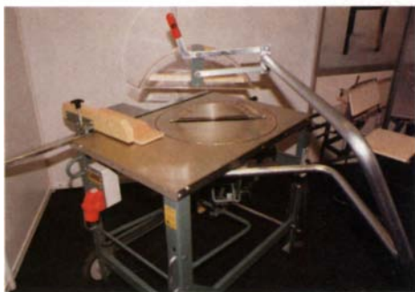
Unusual portable tablesaw from Norway —The Norsaw, which is not available in the United States, has a blade/motor housing that tilts and rotates.
