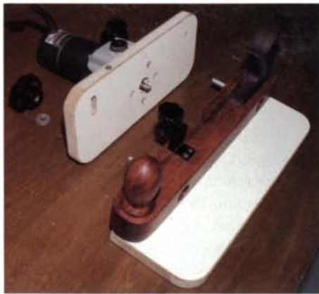
Easy design and assembly from odd materials. Trimmer is mounted in a fence and attached to a base at 90°.
