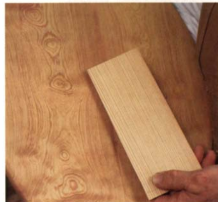
Curly pine is rare. Quartersawn heart pine shows tightly spaced annual rings, characteristic of old-growth timber. Much rarer is the curly heart pine behind it.
