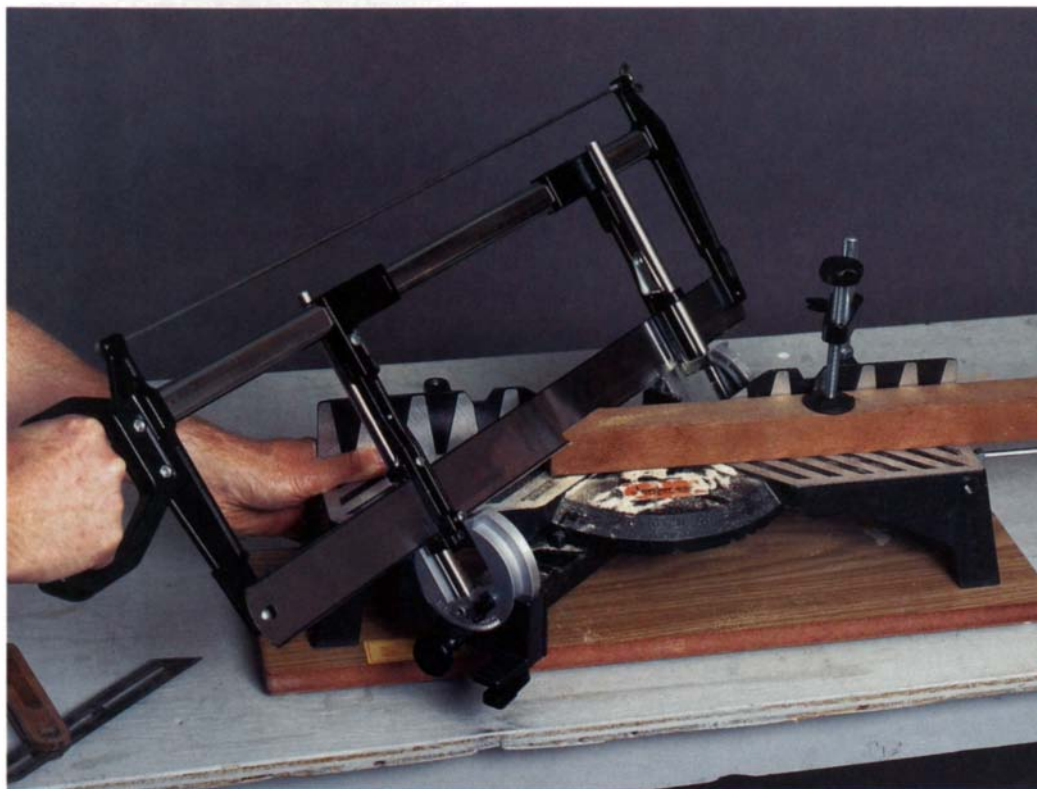
Jorgensen hand-powered compound miter saw —The fine-tooth blade on this saw cuts slowly but leaves a smooth surface. It comes with one hold-down.
