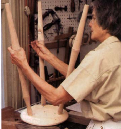
Dry-fit the legs to measure the stretchers. Stretchers are cut to fit; it doesn't matter whether all the stretchers are the same size.
