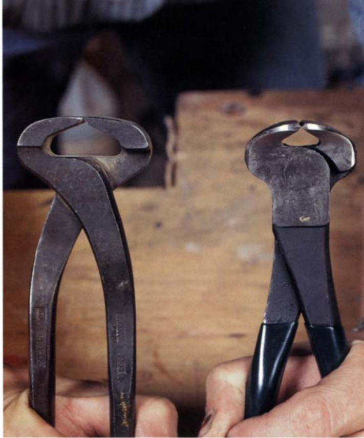
Pincers ground flat, like those on the left, will grab nails set almost flush to the surface.
