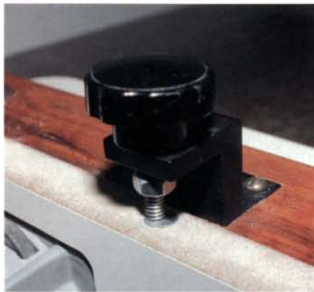
Adjusting knob sets cutting height. A roofing nail makes a resilient contact point, reducing wear on the fence.
