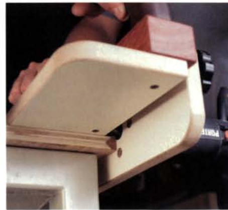
Gap between base and fence avoids obstacles. Trimmer won't hang up on glue squeeze-out or oversized edge trim.
