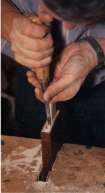
A broken tenon can be rebuilt by drilling out what's left and gluing in a new piece. Veneer can be used to build up the tenon to the correct thickness.
