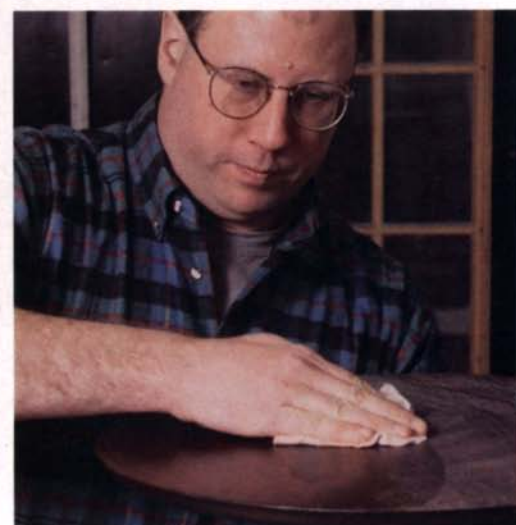
Don't use tack rags to wipe off dust. They can leave chemical residues that will show up as blemishes under a waterborne finish. Use a rag dampened with water.
