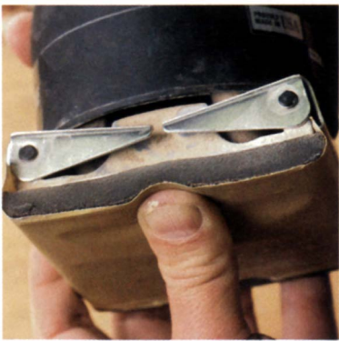
Soft pads let the sandpaper deflect. Soft backings on sanding tools won't support the sandpaper and make it cut more slowly.
