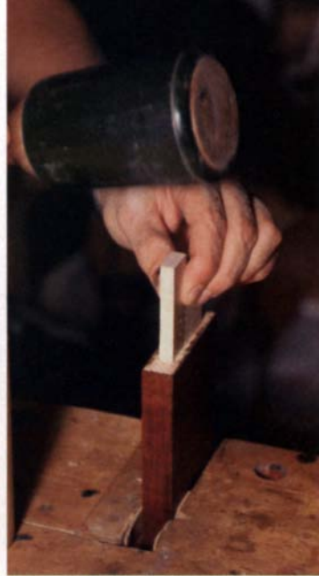
A broken tenon can be rebuilt by drilling out what's left and gluing in a new piece. Veneer can be used to build up the tenon to the correct thickness.
