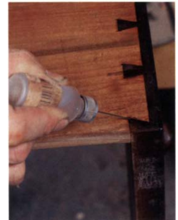
Alcohol crystallizes hide glue. The author wicks denatured alcohol into a dovetail joint, weakening the bond.
