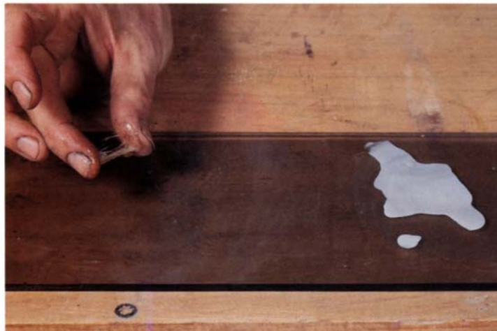
A simple test identifies glue. Water turns PVA glue white and makes hide glue sticky. Knowing which type was used makes taking furniture apart much easier.
