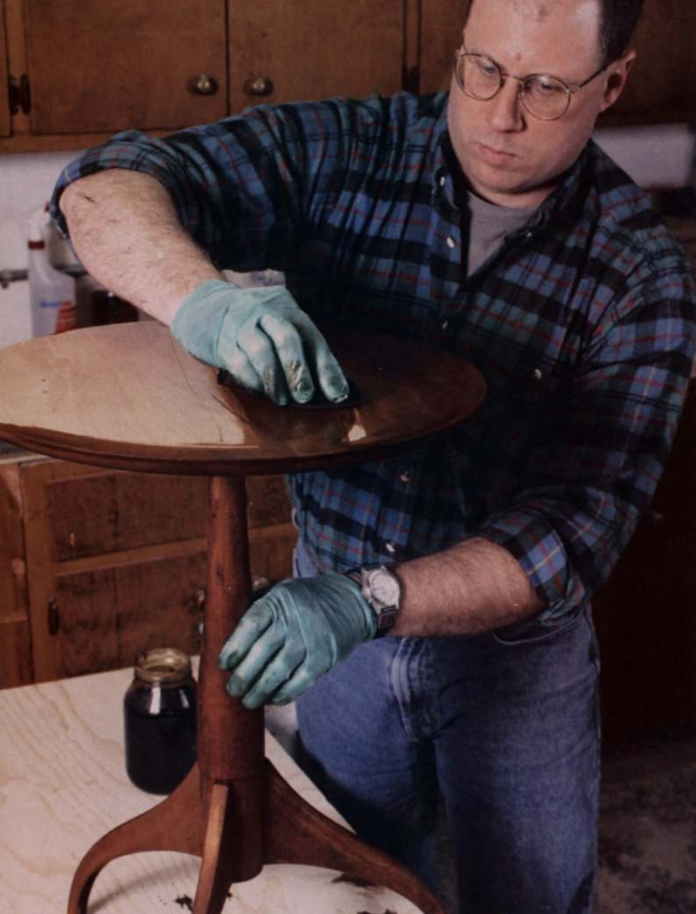
Waterborne dyes are rubbed on with a rag. Flood the workpiece when applying stains and dyes. Work quickly, and wipe off any excess to avoid lap marks.
