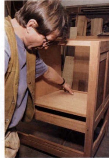
The case is built. With the two end assemblies connected and the case divided into its three main sections, the carcass is ready for doors and drawers (left). The case includes two hidden compartments (below).
