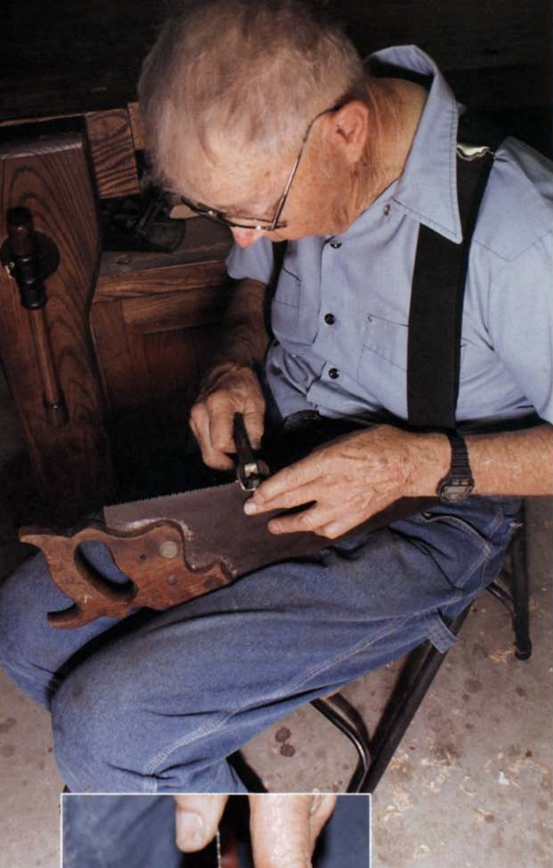
It's easier to move the saw up your lap than to move the set down the saw (above). Only the top part of the tooth should be bent (left).
