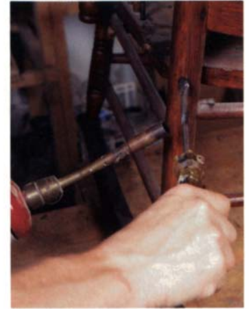
Heat a frozen screw by torching the shank of a screwdriver held in the slot of the head. Once the screw is cool, it's easy to remove.
