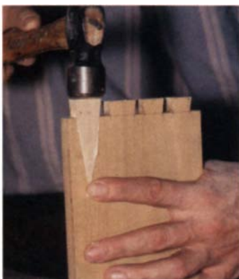
Adding a new tail—To replace a broken tail, define the angle of the saw cut into the piece by following that of the original joint. The long V-shaped cut allows plenty of glue surface for a good grab.
