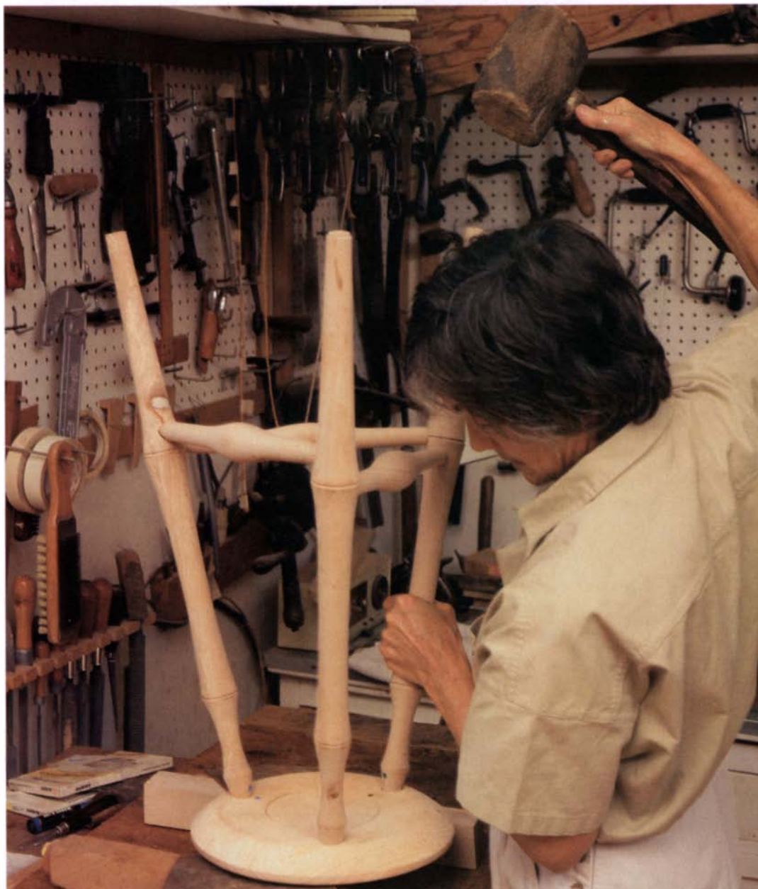
Colored tabs make a quick visual index of one part of the stool to another. The author supports the seat on scrap blocks when pounding legs in place.
