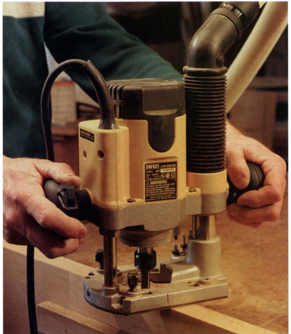
DeWalt 621 variable-speed plunge router —This 2-hp router comes equipped with a built-in dust port. Most of the tool's controls are built into the handles.
