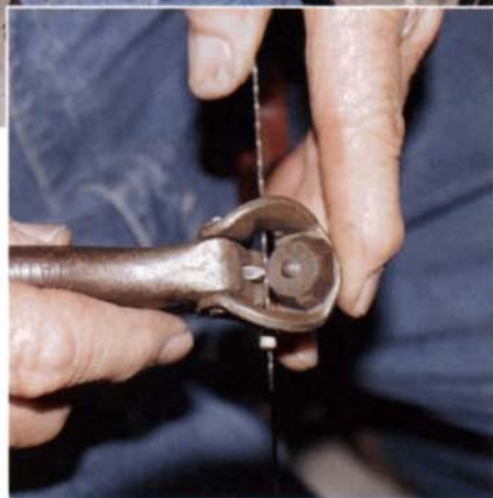
It's easier to move the saw up your lap than to move the set down the saw (above). Only the top part of the tooth should be bent (left).
