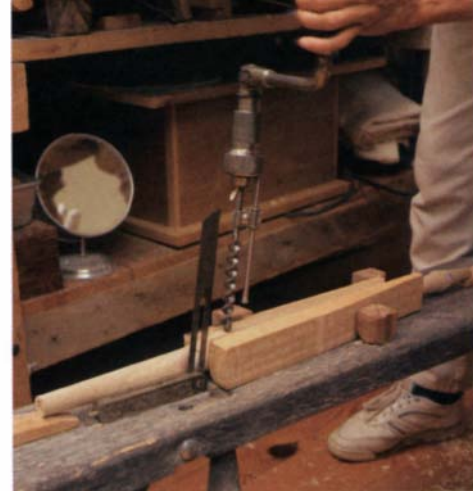
Wedges and dogs hold the legs in place when boring holes for the stretchers. Three dogs hold the workpiece firmly at a comfortable height off the floor.
