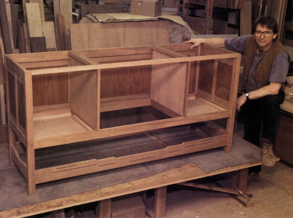
The case is built. With the two end assemblies connected and the case divided into its three main sections, the carcass is ready for doors and drawers (left). The case includes two hidden compartments (below).
