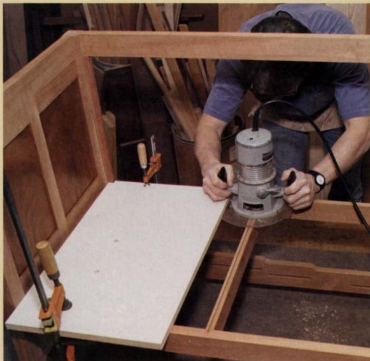
Divider rails are grooved for splines. Splines connect the rails to plywood dividers. The same spacer used to rout the dovetails for the divider rails is used here.
