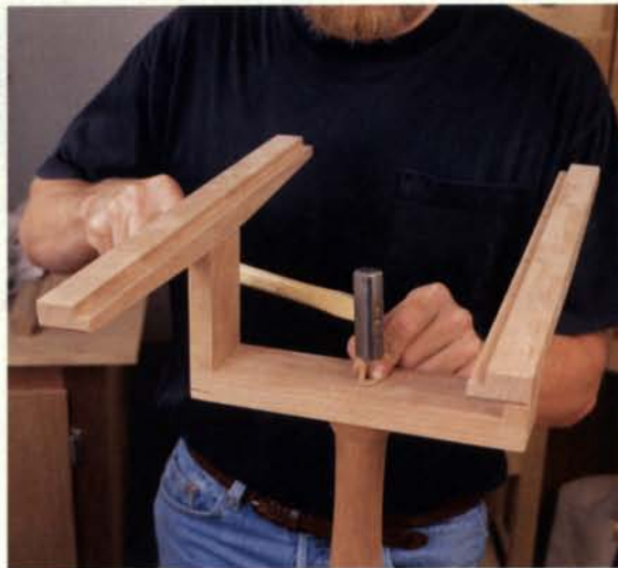
Glue and insert a wedge in the slotted tenon to secure the yoke to the pedestal. Orient the wedge perpendicular to the crosspiece's grain to prevent splitting.
