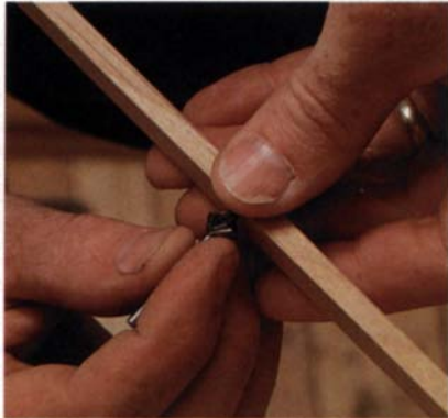
Clean up both sides of the escutcheon-pin shank holes by hand-turning a small countersink.
