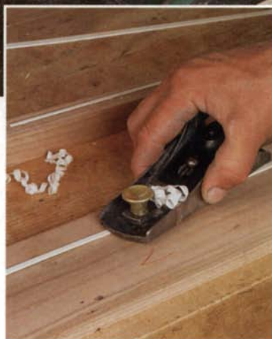
Rip strips of inlay on the tablesaw. Because the inlay stock is so thin, take it off on the waste side of the blade (above). Slice strips to 1/4 in. or so with a knife and straightedge. Plane to width with a block plane (right), beveling slightly to match the groove. Check the fit frequently.
