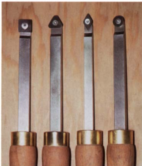
Scraper tips are held with a screw. They can be turned to expose a new cutting edge.
