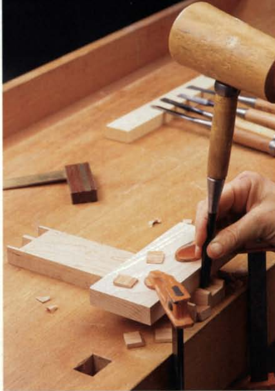
A guide block improves accuracy—When chopping the through dovetails in the crosspiece, the author uses a block of wood to guide his chisel. The crosspiece forms the bottom of the U-shaped yoke.
