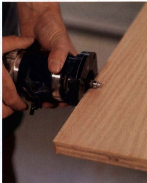
Run the router in a climb cut (from right to left) to prevent tearout. It leaves a rough edge, so follow with a block plane.
