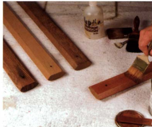
Glazes make a leg look old. The author used glazes on three legs of a table (above) to match a leg that had darkened from iron reacting with tannin. He applied a tan base color and then defined the pores and grain patterns with darker glazes.
