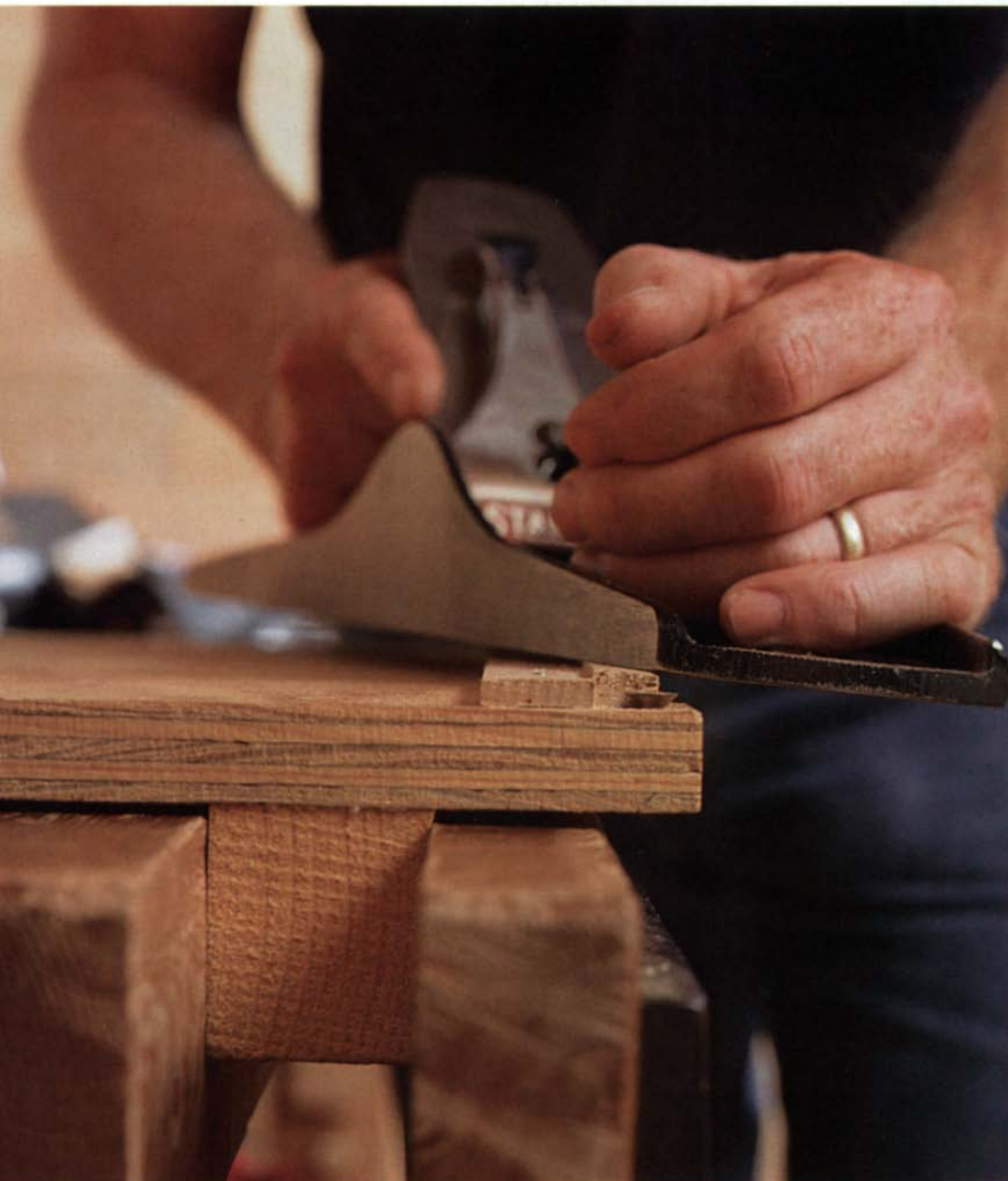
Chamfering the beveled strips relieves any sharp edges.
