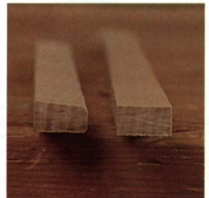
The strip on the left is ready to install. The bevel and chamfers, though small, are obvious when compared to the rectangular strip on the right.
