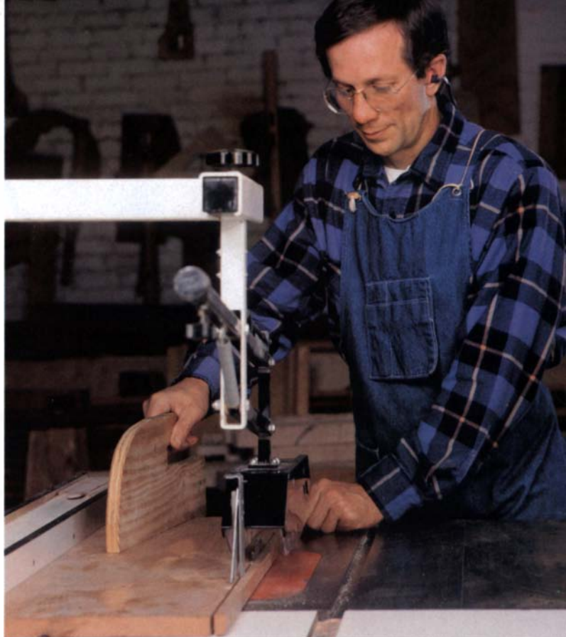
Large push stick keeps stock against fence and holds it on the table. Note that the author is not standing in line with the blade.
