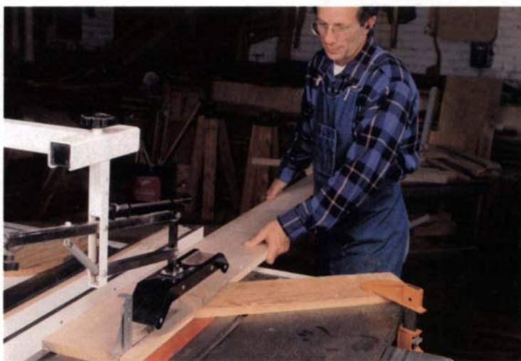
A featherboard holds the stock against the fence, reducing the chance of kickback. Mount featherboard in front of the blade.
