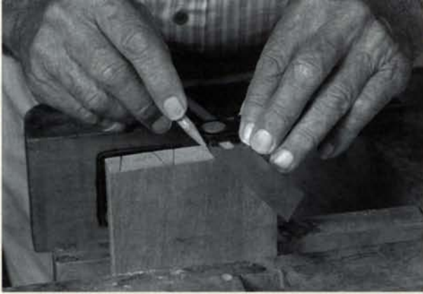
Use a bevel gauge to extend pin and half-pin marks across the end of the board. A 1:6 ratio is about the right angle for most hardwoods.
