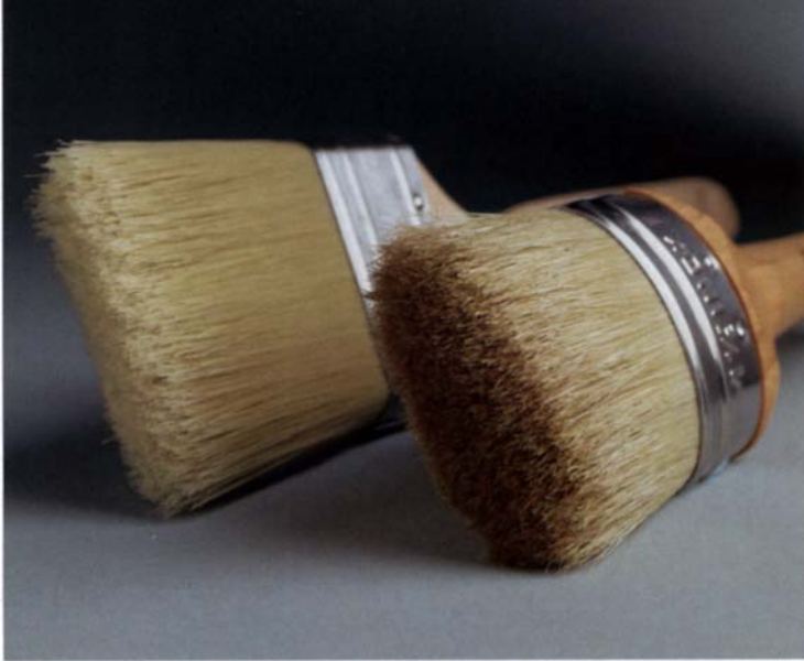
Same width, more bristles. The oval chisel-edge brush (right) will hold more finish than the flat chisel-edge brush. This allows varnish to be applied in long, smooth strokes.
