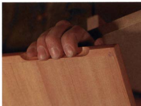
Finger pulls are deeper than standard edging. So make the bottom edging thick enough to accommodate them.
