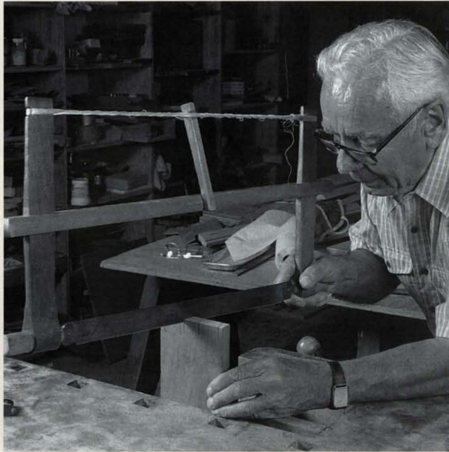
Cut to the gauged baseline. Split the line with the sawblade on the waste side.
