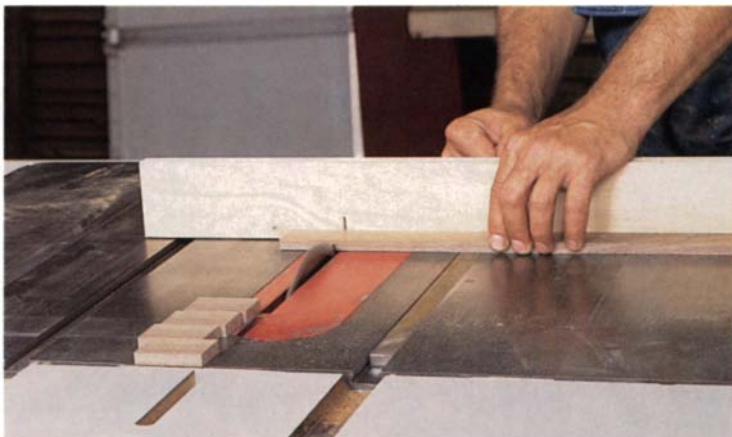
Miter-gauge fence prevents kickback by pushing offcuts away from the blade and providing more support to the stock.
