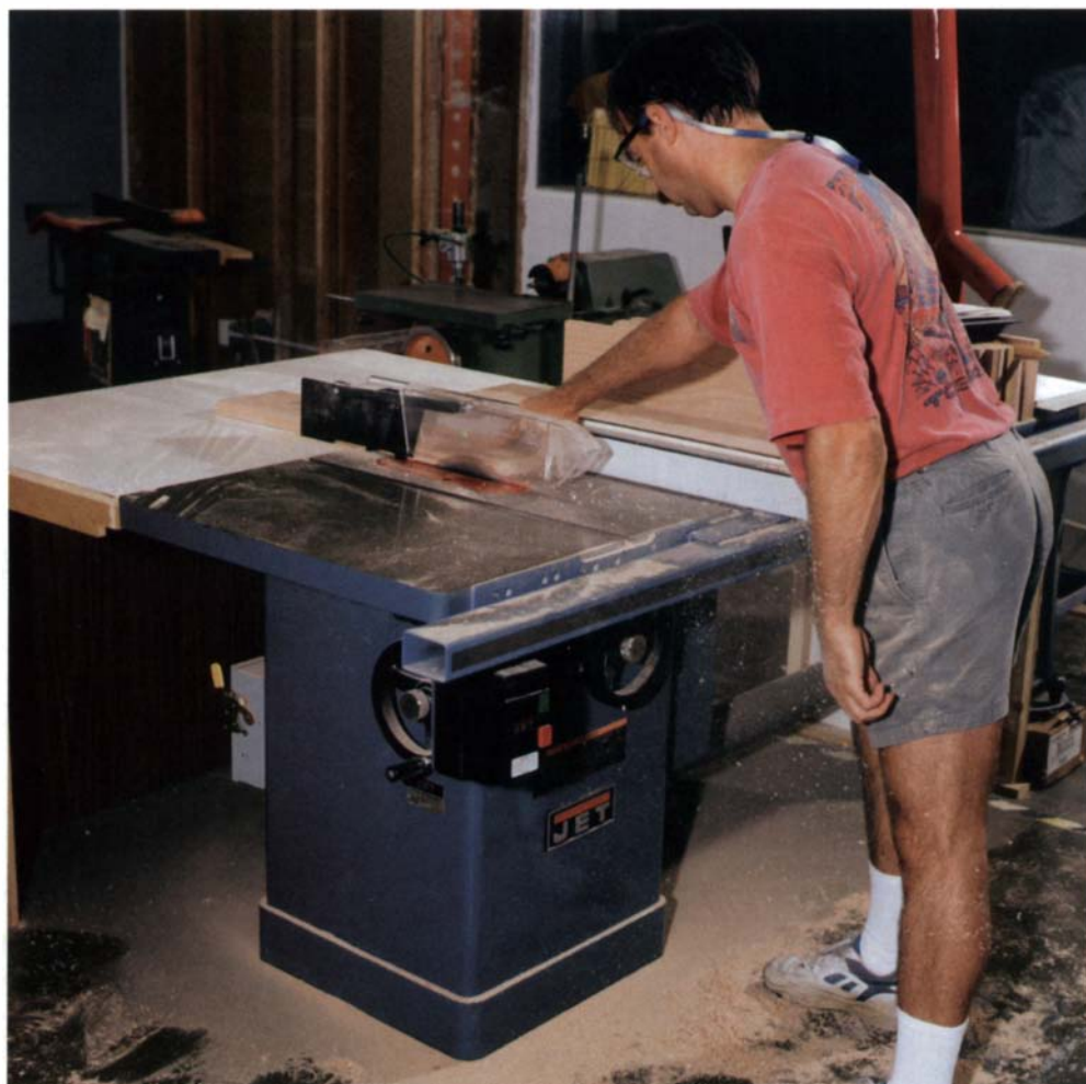
The Jet tablesaw has a large cast-iron top, magnetic switch and a choice of rip fences.
