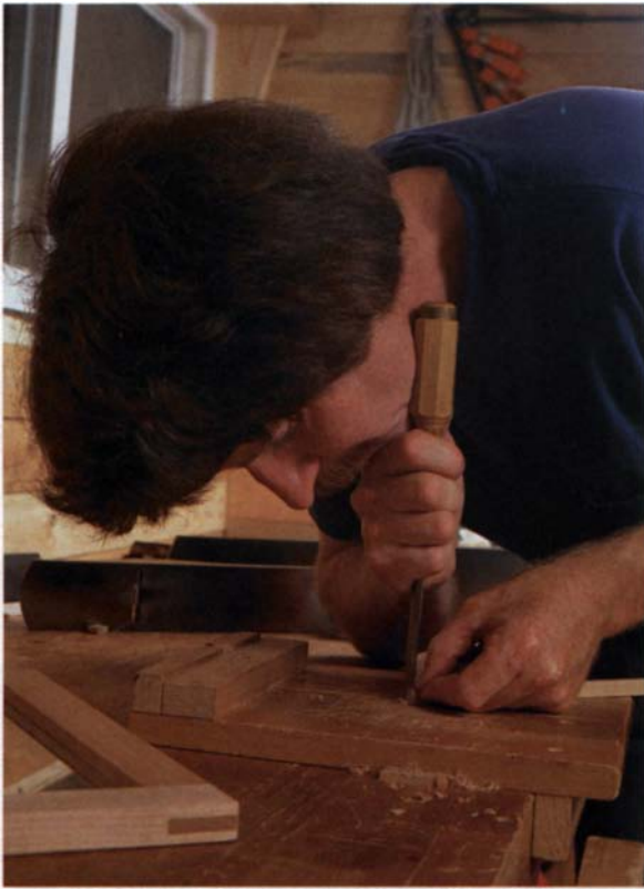
Use a chisel to pare the ends of the strips to fit after cutting them a little long with a backsaw.
