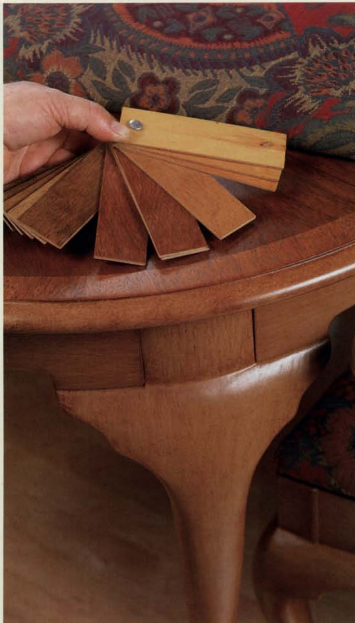
Stain sticks aid color choices—Guided by a fan of stain sticks, the author chose a glazing stain for this tabletop. The samples also helped the customer come up with a color that makes the veneer band look natural and blend with the chair fabric.
