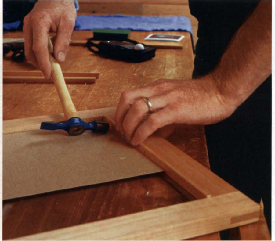
Protect the glass with cardboard, and carefully use a light hammer when setting the escutcheon pins.
