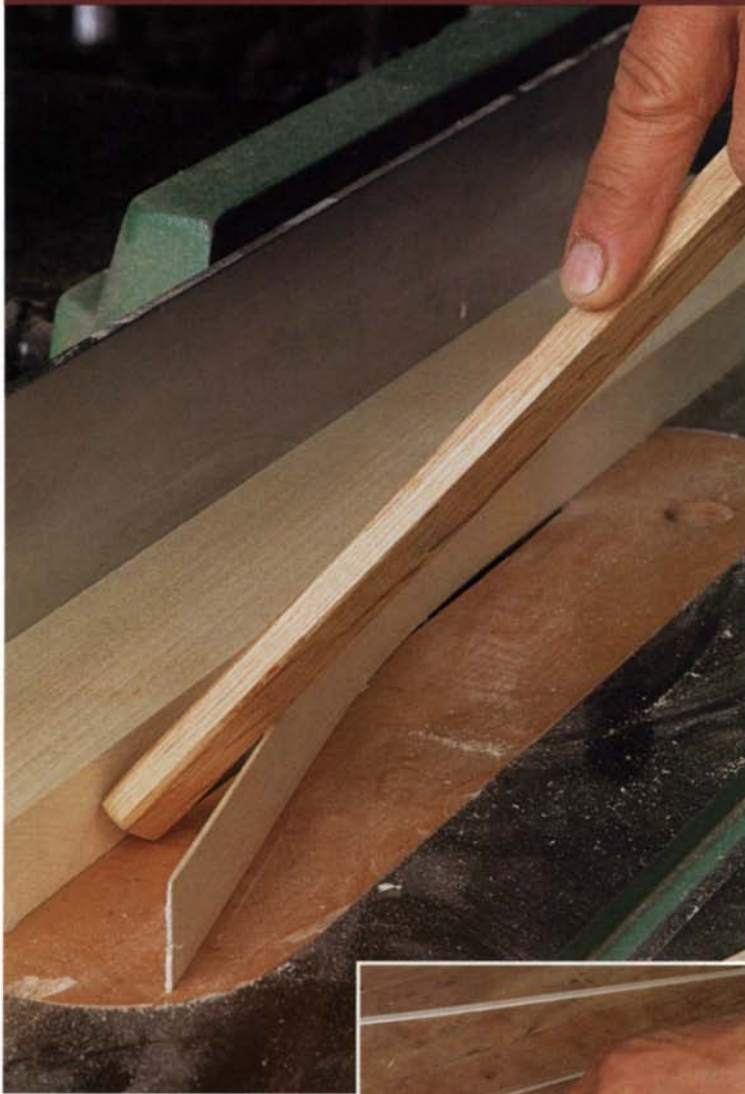
Rip strips of inlay on the tablesaw. Because the inlay stock is so thin, take it off on the waste side of the blade (above). Slice strips to 1/4 in. or so with a knife and straightedge. Plane to width with a block plane (right), beveling slightly to match the groove. Check the fit frequently.
