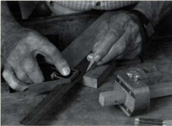
Extend the pin marks down to the baseline using a combination or try square.
