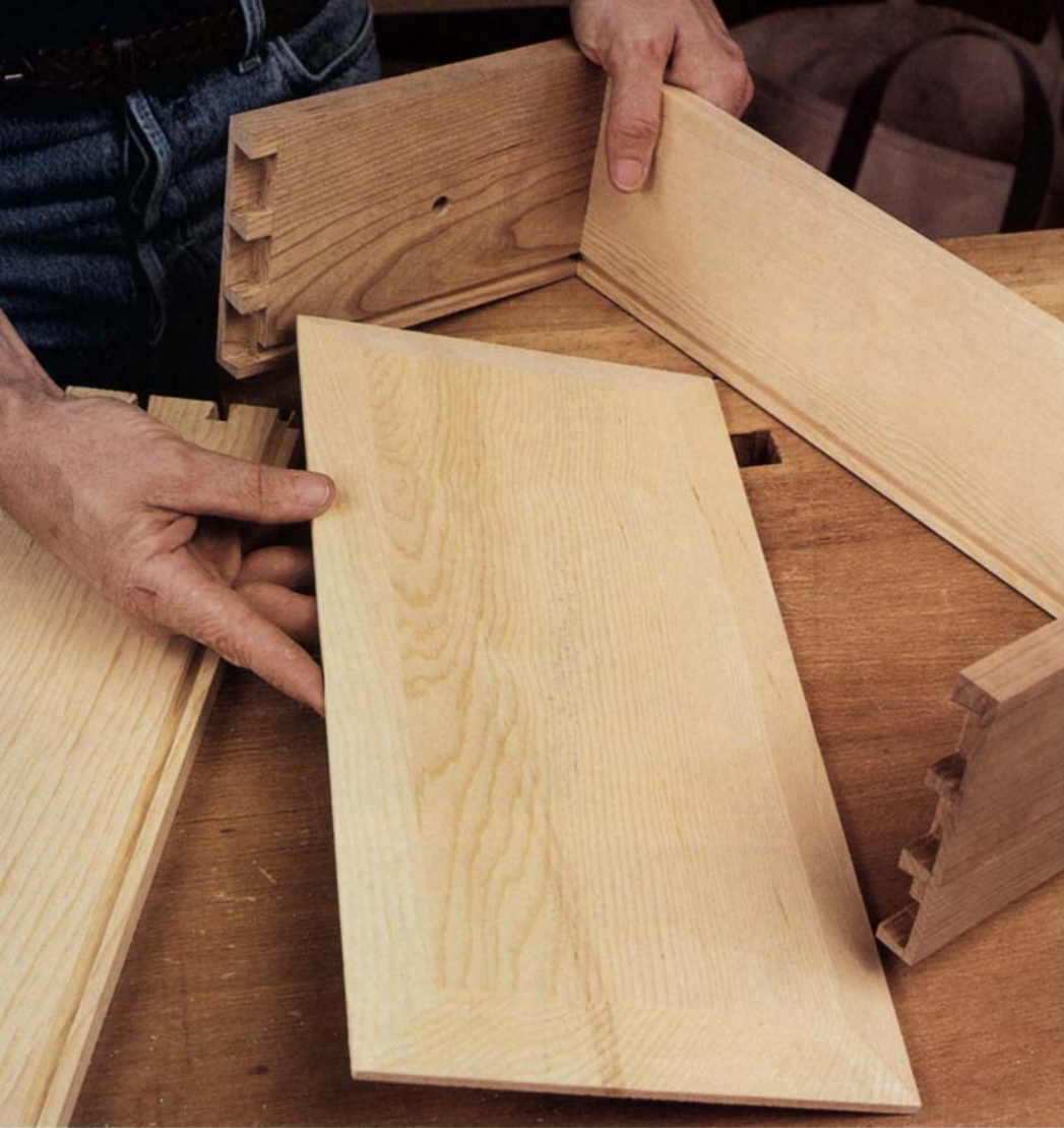
Assemble the drawer with the bevel down. The pine bottom floats in grooves in the pine sides and in the cherry drawer fronts.
