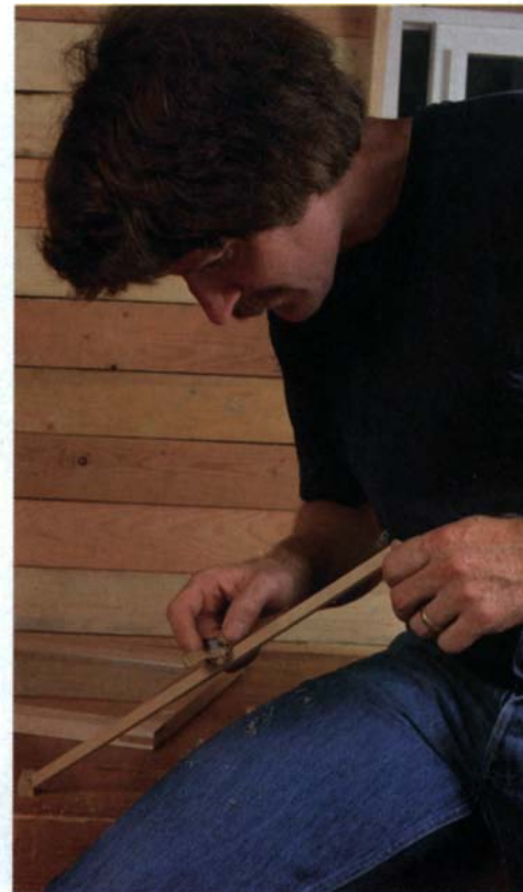
Chamfering the beveled strips relieves any sharp edges.
