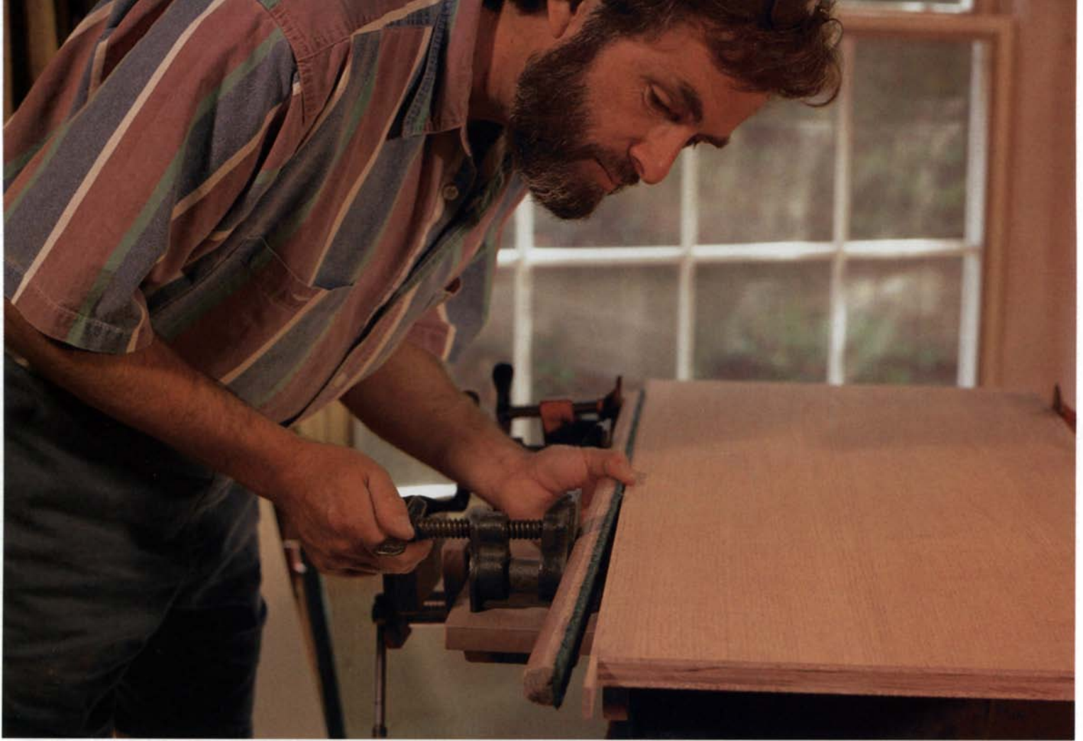
A lightly bowed caul, faced with felt, needs only a few clamps to apply even pressure on plywood edging.
