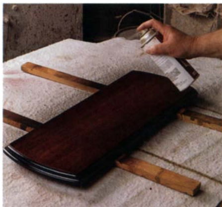
Toner used as a shading stain —To simulate a table with a faded center, the author shades the edge of this mahogany top with a dark toner. After he rings the top with light, even coats, he can refine the look and color by spraying other toner bands.
