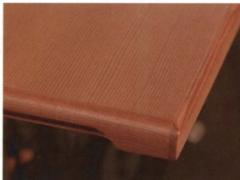
Finish the edges of a door with a \frac{3}{16} -in. roundover bit. Run the sides by the top and bottom to cover the end grain.
