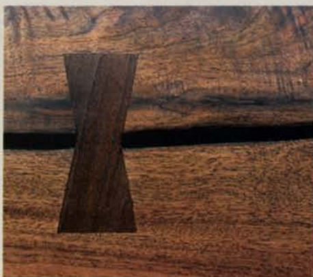
Butterfly keys save boards, preventing checks from spreading and providing a decorative element as well.
