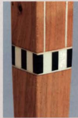
Cuff inlay, which is a band encircling a leg near the floor, is the traditional termination for string inlay.
