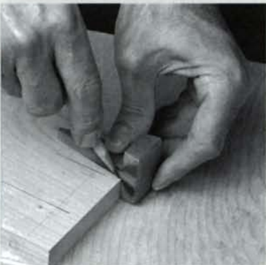
Mark the angles of the pin sockets with a dovetail gauge or a bevel square. Transfer these lines across the end grain. Now tape the two tail boards together, so you can cut pin sockets on both at the same time.
