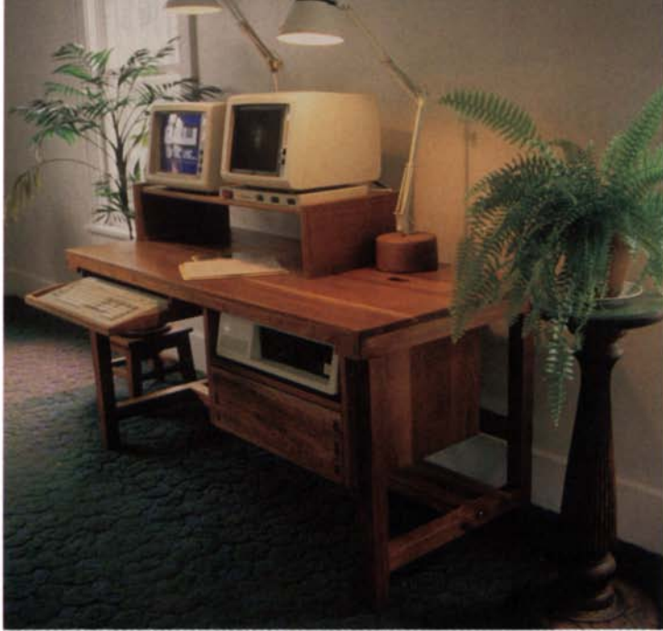
This computer workstation, built from cherry wood by Hugh Foster, features a retractable keyboard drawer, a raised shelf for two monitors, a drawer for floppy discs and two mechanical-arm lamps on wooden bases that can be moved to give light where needed.
