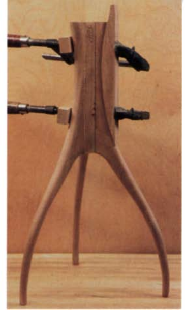
These three photos show the fixture and clamping arrangements used for assembling two legs with a filler block (left); two filler blocks with a leg (center); and the final pedestal glue-up (right). A scrap piece, left over from the bandsawing of the legs, is used as a caul.
