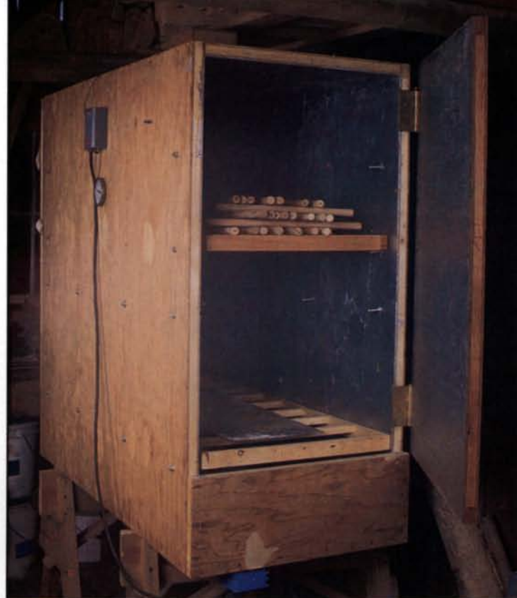
A piece of sheet metal on the bottom rack of this kiln deflects the direct heat from the electric baseboard heater below.
