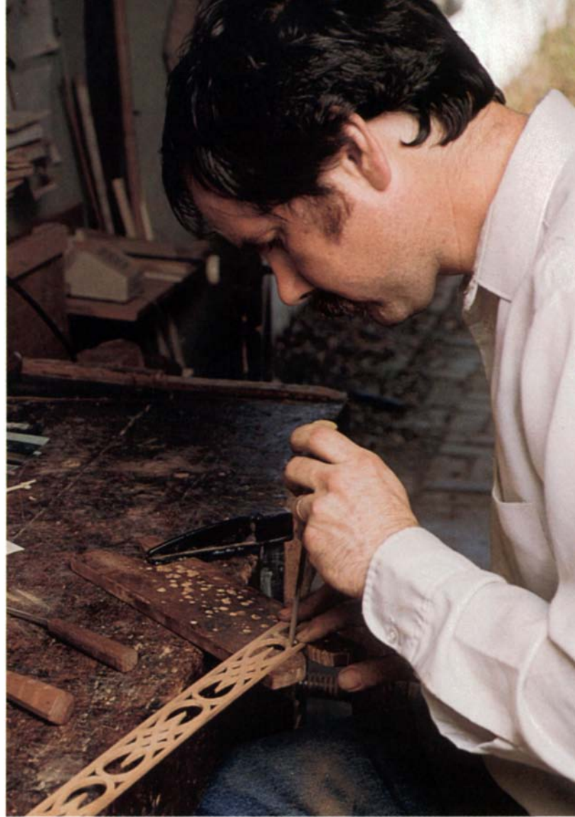
The author supports the fret on a bird's-mouth fixture clamped to the workbench while smoothing out the roughsawn edges of the design with small files and chisels.
