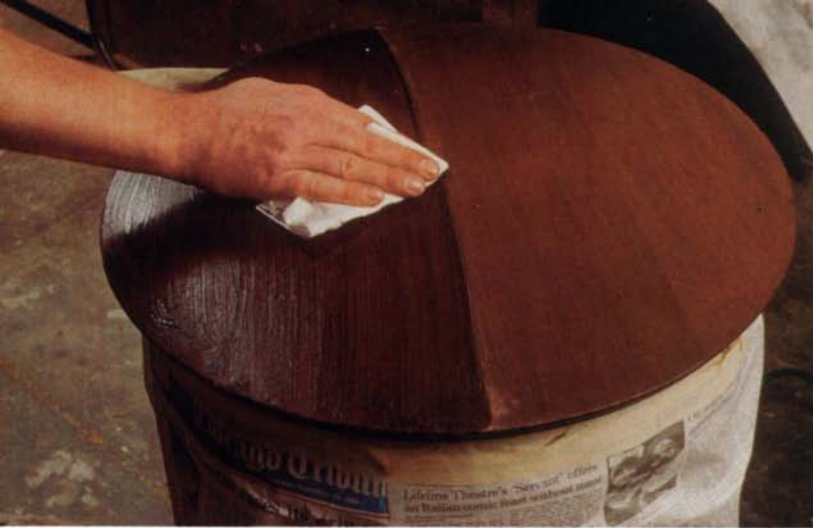
Glazing is done by thoroughly sanding the first coat of varnish and then wiping with an oil-based stain (above, left). Remove any heavy build-up before spraying additional coats of varnish. The subtle tone change obtainable is evident in the photo above, right.
