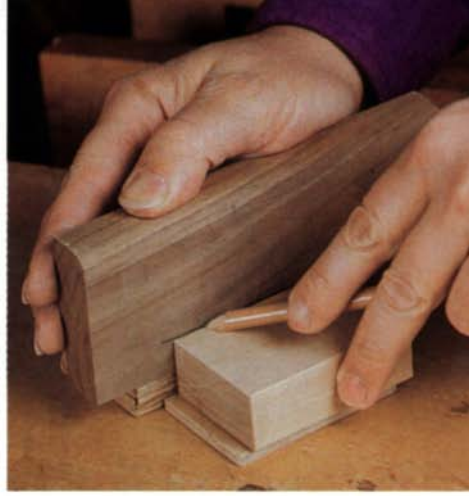
Used in conjunction with 1-2-3 blocks, plywood spacers allow fractional distances to be marked. Shown here, distances between spacer sizes can be marked by shimming the workpiece and subtracting that distance from the marking-block stack.
