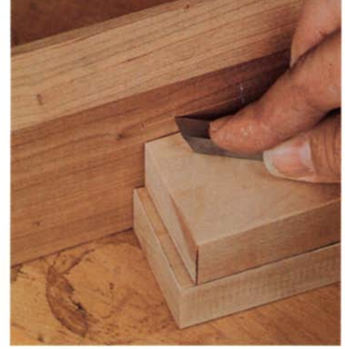
Another method for marking fractional distances uses square-steel tool bits—cutters commonly used on the metal lathe. By grinding the tip to a bevel and using it on top of 1-2-3 blocks, the tool bit serves as both a spacer and a marking knife.
