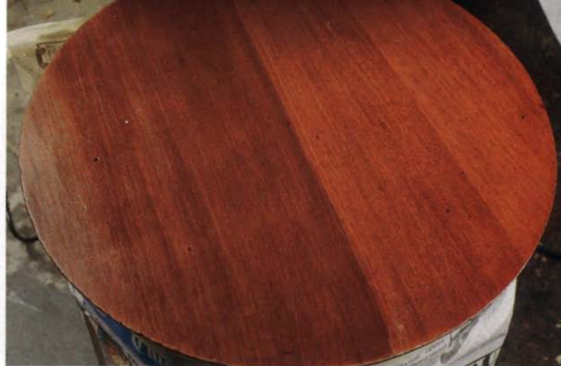
Glazing is done by thoroughly sanding the first coat of varnish and then wiping with an oil-based stain (above, left). Remove any heavy build-up before spraying additional coats of varnish. The subtle tone change obtainable is evident in the photo above, right.
