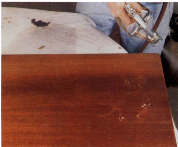
Spraying varnish requires a minimum investment in equipment, is easy to do and yields extremely good results.
