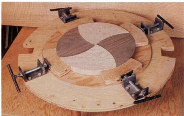
This gluing fixture applies uniform pressure in a radial direction. The wood cauls can be modified to accommodate various size discs.
