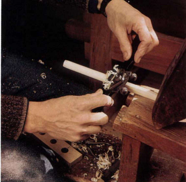
Langsner uses a shaving horse to hold a rung as he shapes and sizes it with a spokeshave. The small block with the three holes is his fitting gauge. The sides of the first hole are colored, so when a tenon is rotated in the hole, the color shows where the tenon needs to be shaved more.
