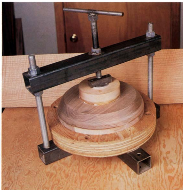
A versatile shop-built press clamps the top of the pot to its bottom during glue-up. Its external profile is later refined on the lathe.
