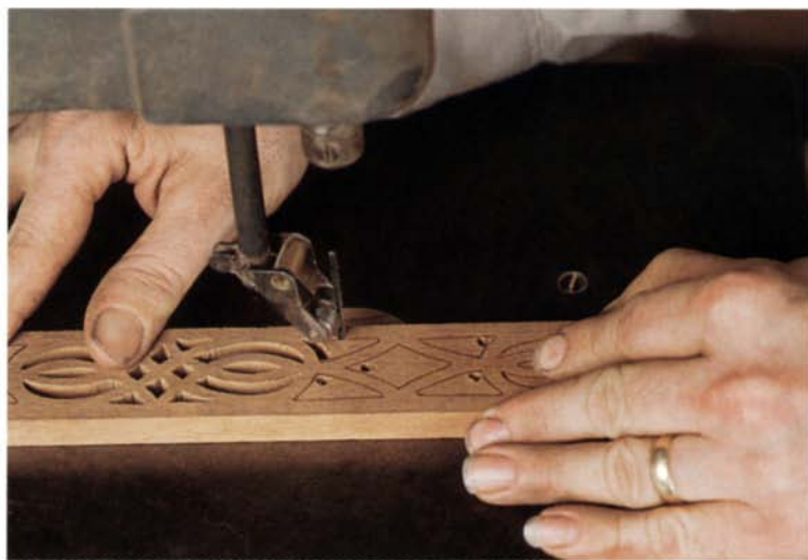
It's important to cut away the line completely to preserve the delicacy of the fret design. By replacing the saw's upper blade guide with a roller blade support from an old sabersaw, the blade need not be attached at the top. This makes it easy to raise the guide and insert the blade into the next opening to be sawn.
