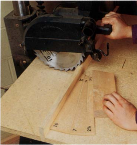
Eze-Angleguide lets you cut any angle without resetting your radial-arm saw.
