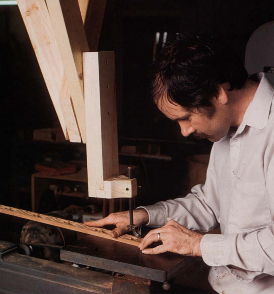
The 22-in. throat of Pine's scroll saw limited the length of stock he could easily cut. To overcome this limitation, he attached a 2x4 frame to the ceiling to hold the roller blade support, removed the saw's arm and positioned the saw table directly below the upper guide.
