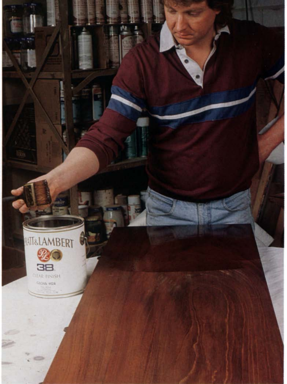
Brushing varnish can yield good results. To avoid air bubbles in the finish, don't scrape the brush on the side of the can, but allow excess to run off, as shown by the author.
