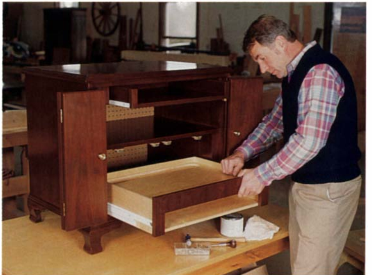
Frank Klausz does the final drawer adjustment on a computer cabinet he designed for an executive office. The mabogany cabinet has bi-fold doors that conceal a pull-out keyboard and a two-tier printer drawer that has one slot at the front for loading paper, and another slot at the rear for paper to feed up to the printer.
