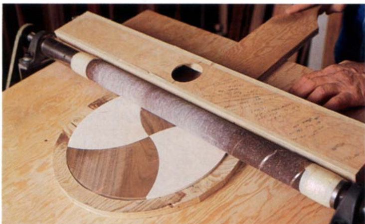
This shop-built thickness sander flattens the segmented disc so it can be mounted and shaped on a lathe. The sander is similar to the one in 'FWW on Making and Modifying Machines,' p. 38.
