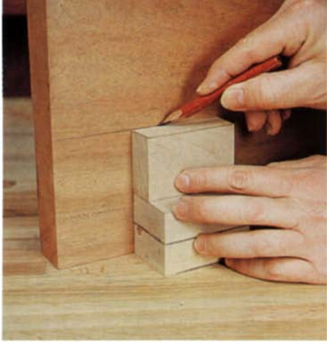
1-2-3 blocks are a handy alternative to measuring with a ruler or tape measure. Here, a stack of blocks that's 4 in. high is held against a board, on edge on the workbench. The line is marked as the stack is slid along the board.
