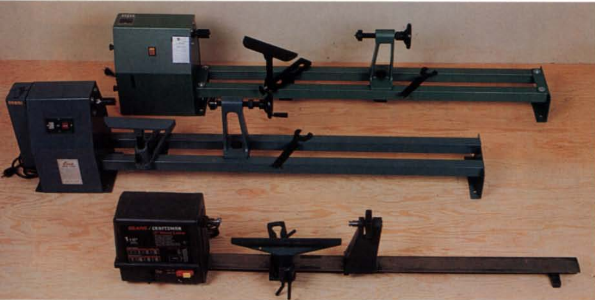
The Grizzly G1025 (top) and Enco 199-9055 (bottom) look-alike lathes are Taiwan imports. The motors for these, and the smallest Sears lathe (bottom), are mounted compactly in the headstock housing.
