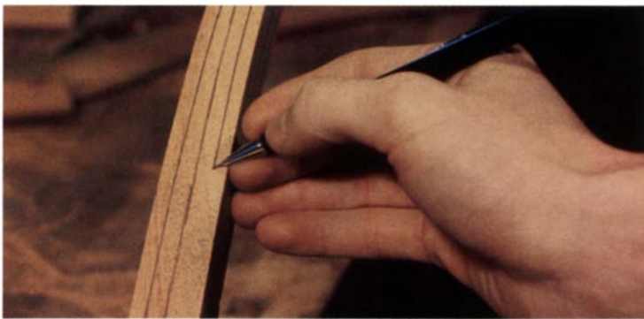
The author freehands penciled guidelines along the leg's edge before shaping with planes, rasps and files.
