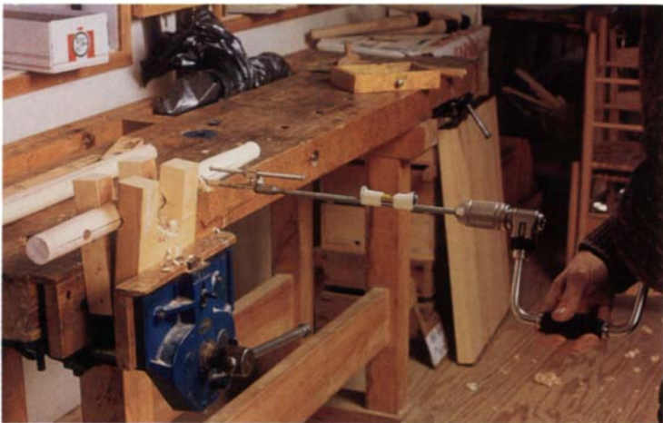
The notched blocks hold the post so all the mortises in one side can be bored without having to loosen the vise to move the post. A builder's line-level taped to the bit extension aligns the bit and a depth-stop clamped to the bit controls depth.
