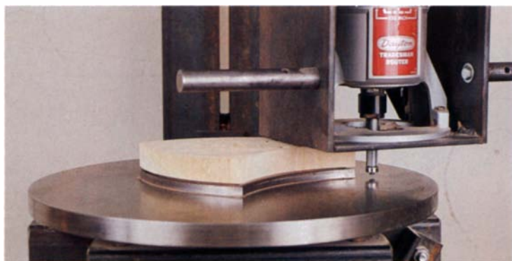
Mongold uses a shop-built radial-arm router to shape segments. The segments, rough-cut with a bandsaw, are firmly positioned on steel templates and held in place by a vacuum chuck. A flush trim router bit guided by a pilot bearing does the final shaping.
