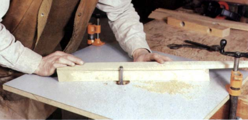
The curves on the outside of the legs are roughed out on the bandsaw and then cleaned up with a straight bit and template on the router table. Note that the template curves in two planes to accommodate the curve routed during the first pass. Always test such a setup before trying an actual leg.
