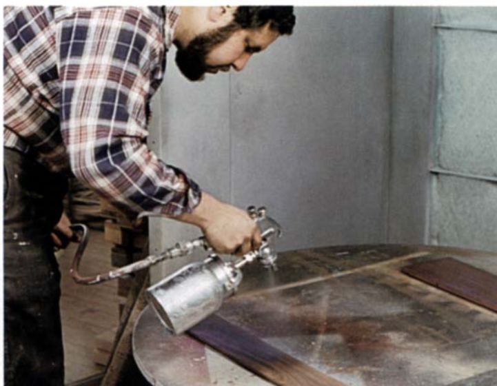
Hydrocote's milky-white color belies the fact that it dries to be as transparent as nitrocellulose lacquer. Since Hydrocote is nontoxic, the author sprays a sample without a respirator on.
