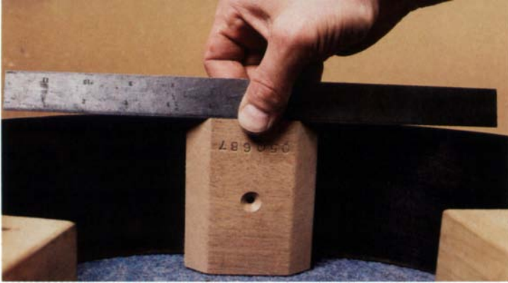
Checking the relationship of the high end of the beel block to the tapered sides. Also see figure 1, for measurements.
