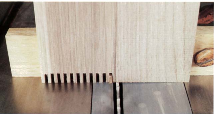
The first half of the joint begins with a finger, so the mating piece must begin with a slot. The initial finger on the first piece becomes a stop for cutting the first slot on the mating piece. After the slot is cut, the sequence is the same as described above.
