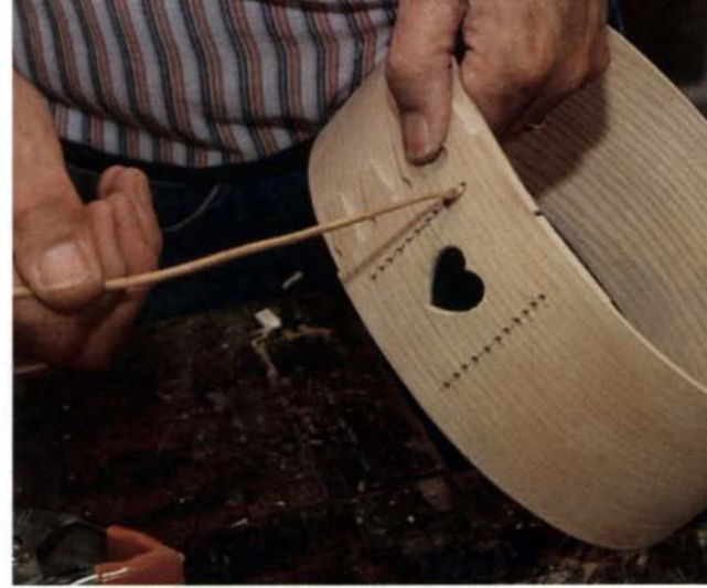
Each loop of birch-root lacing is pierced with an awl to allow the lacing coming from the inside of the box to be passed through it. Note that the lacing has been sharpened to ease its passage through the holes.
