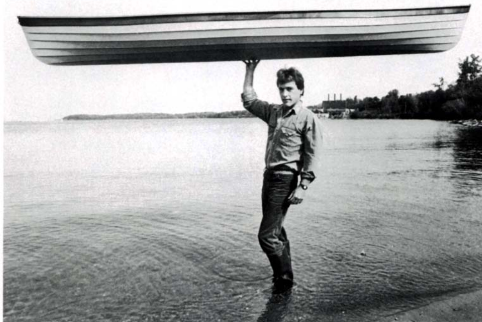
Tom Hill's ultra-light lapstrake canoes are a wilderness backpacker's dream. At 11 ft., 6 in., this monocoque canoe weighs only 25 lbs.
