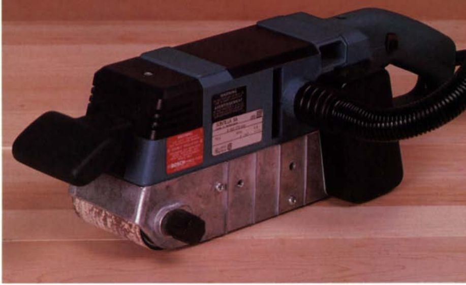
Held rigidly in its stand and fitted with its angle guide, the Elu 4023, above, can be used as a small stationary sander. Fitted with its optional air-vac attachment—a hose connecting from the sander's dust port to a vacuum cleaner—the Bosch 3270D, left, undoubtedly becomes the cleanest-to-use belt sander on the market.
