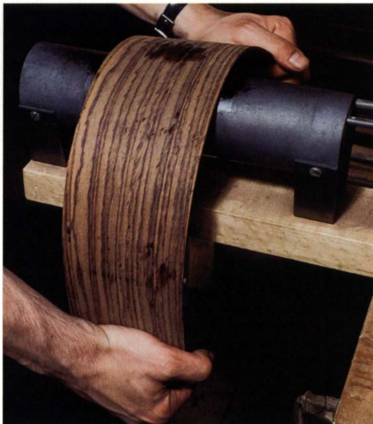
Guitarmakers shape the sides to conform to the guitar mold by bending the dampened wood over a heated pipe, moving the wood constantly to avoid kinks and scorching. With a little practice, the mold can be matched exactly.
