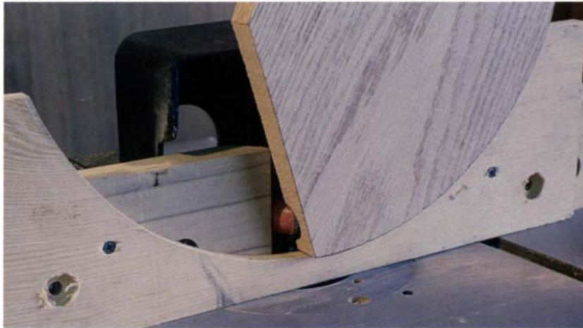
A shopmade high fence supports the workpiece while it is rotated past the cutter, shaping a relief into the radiused face.
