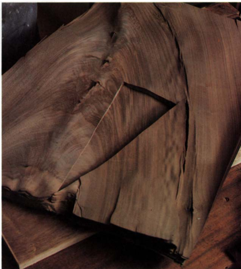
The 16 wedges needed for the tabletop's pattern are cut at one time on the bandsaw from walnut crotch veneer.
