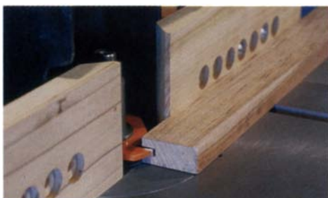
A narrow straight cutter cuts a \frac{1}{4} -in. groove in the edge of a board. Both halves of the split fence are aligned with each other to support the stock before, during and after the cut.
