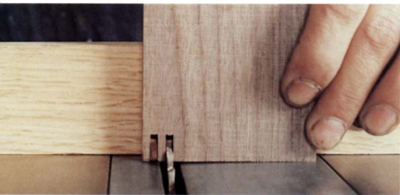
Before the next slot is cut, the board is moved so the previous slot fits over the spline. The process is repeated until fingers and slots are cut across the width of the board.
