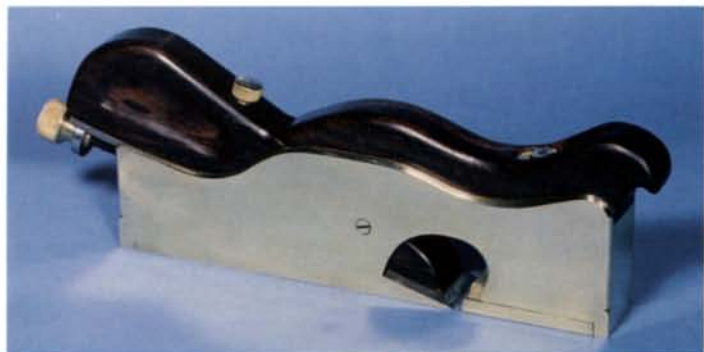
Ian Wilkie's brass shoulder plane with rosewood in-fill weighs a little more than 3\frac{1}{2} lbs. It was made to fit a Record iron.
