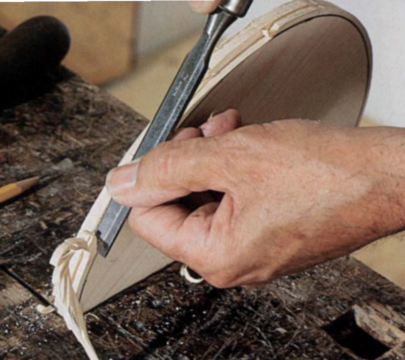
To cut the rabbet in the bottom, the author first marks the back of the rabbet by tracing along the body from inside the box. He then marks the bottom of the rabbet by drawing a line on the outside edge using his hand as a marking gauge. He saws on this line around the box's edge with a dovetail saw, then pares along the kerf, working down to the first line.
