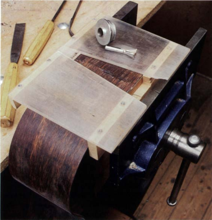
To rout the dovetail socket for the neck, the author uses a standard dovetail bit with a plastic template and a guide bushing.
