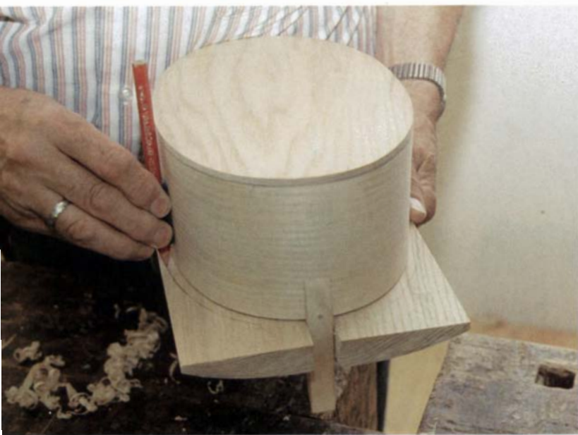
With the lid of the box notched to fit over the clasps, the lid's profile is traced from the body. The pencil is wrapped in tape, thus creating space for an overhang around the box.
