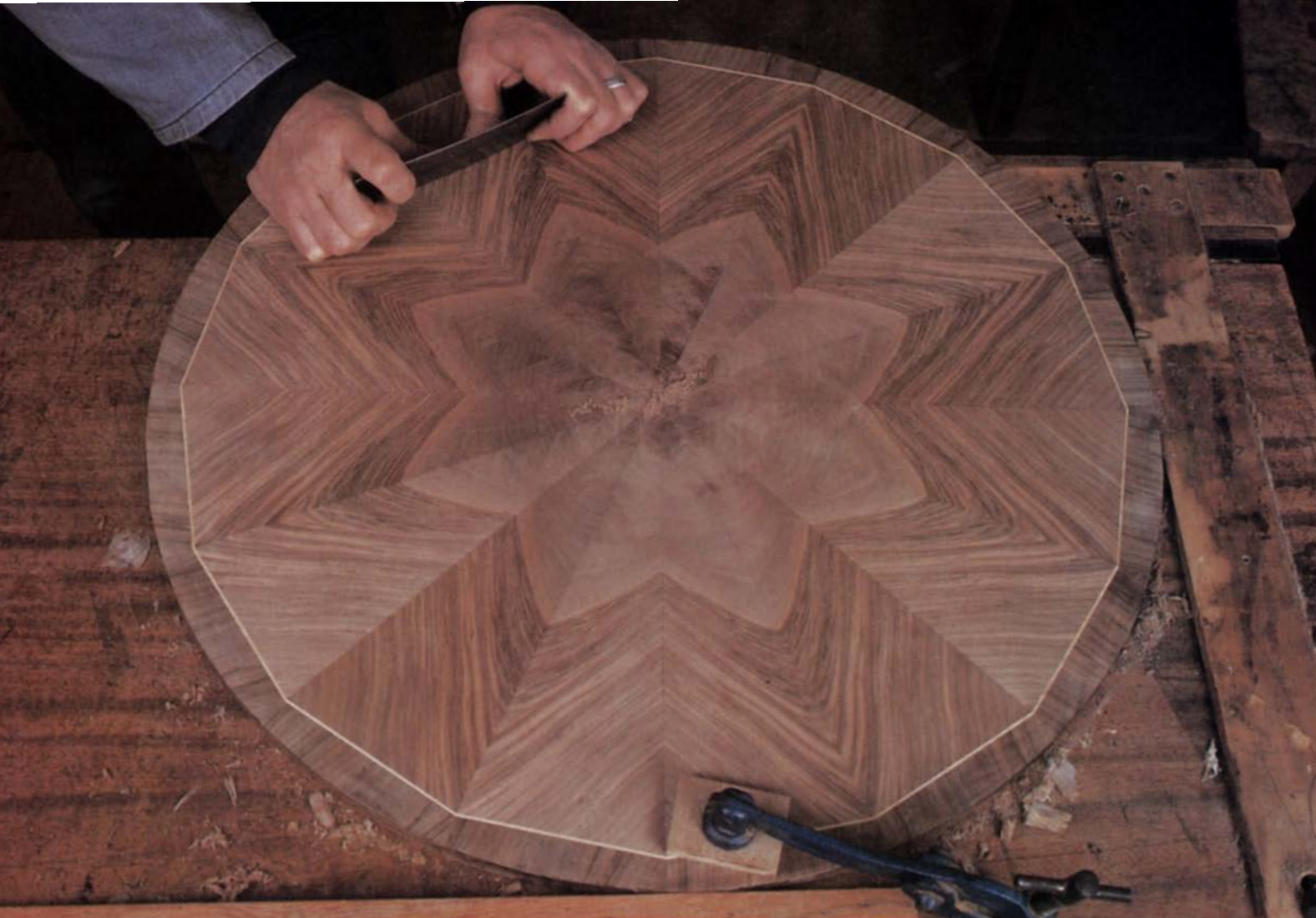
The author created the radiating pattern on his tabletop by cutting wedge-shaped pieces from consecutive leaves of a walnut flitch and hammer veneering them to the plywood top. The underside is also veneered to prevent warping.
