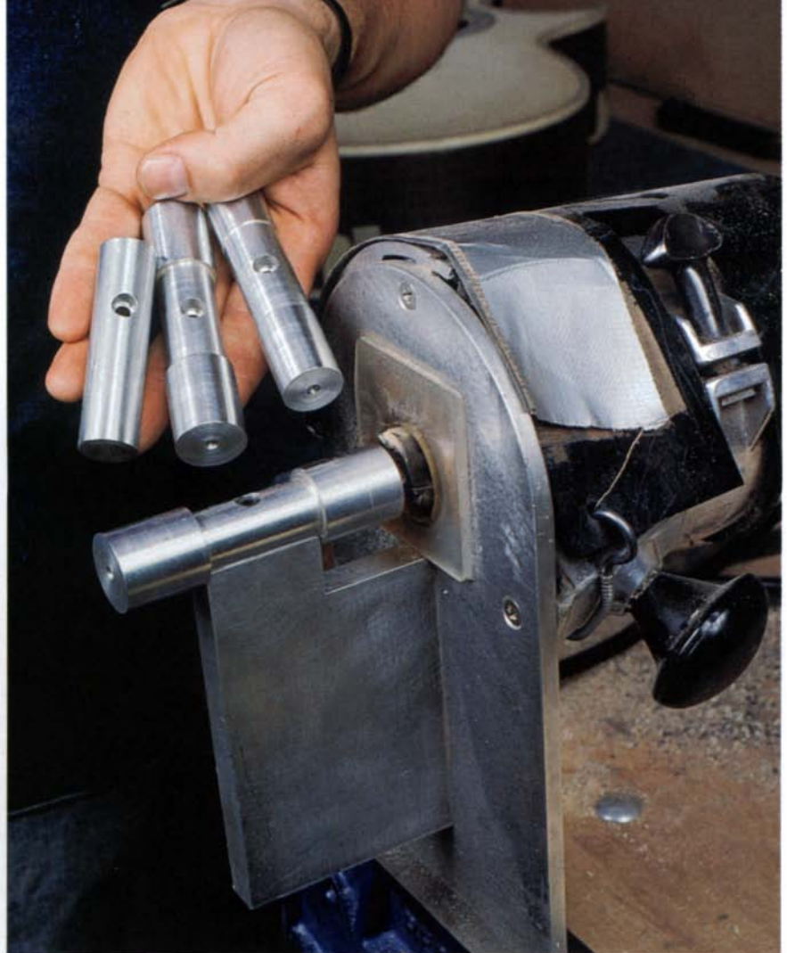
To rout the different-size grooves around the edges of the guitar for inlaying binding and purfling strips, Laskin made this router jig. The side of the guitar bears on the turned aluminum rod as the instrument is moved through the cutter, while the front or the back of the instrument is pressed against the router base. Various rods control the width of the cuts; the depth is controlled by the router's own depth-setting adjustment. The tapered top edge of the small pad in the center of the base allows clearance for the curved back of the guitar. A duct-tape shield directs dust down and away from the operator.
