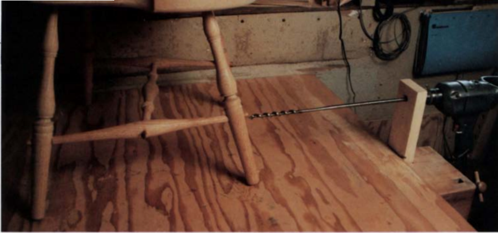
For boring rung holes, Campbell uses a 2x4 with a hole bored through it as a guide for his drill. Demonstrated here on a Windsor chair, the technique works on stools too. To avoid splintering, the auger bit (extended by a pipe welded to it) is retracted when the pilot screw breaks through. The holes are then finished by boring from the other side.
