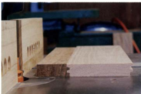
The glue-joint cutter will produce the joint shown by simply flipping the stock over for every other pass. This joint has about 2\frac{1}{2} times more glue surface than a simple butt joint.
