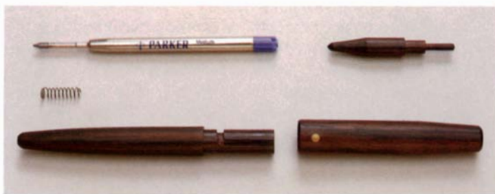
Tired of plastic pens breaking, the author made a two-piece rosewood housing for his ballpoint refills. The tiny trigger on the top makes the pen retractable. A boxwood pin fits into the top locks into a groove in the barrel to hold the pieces together.
