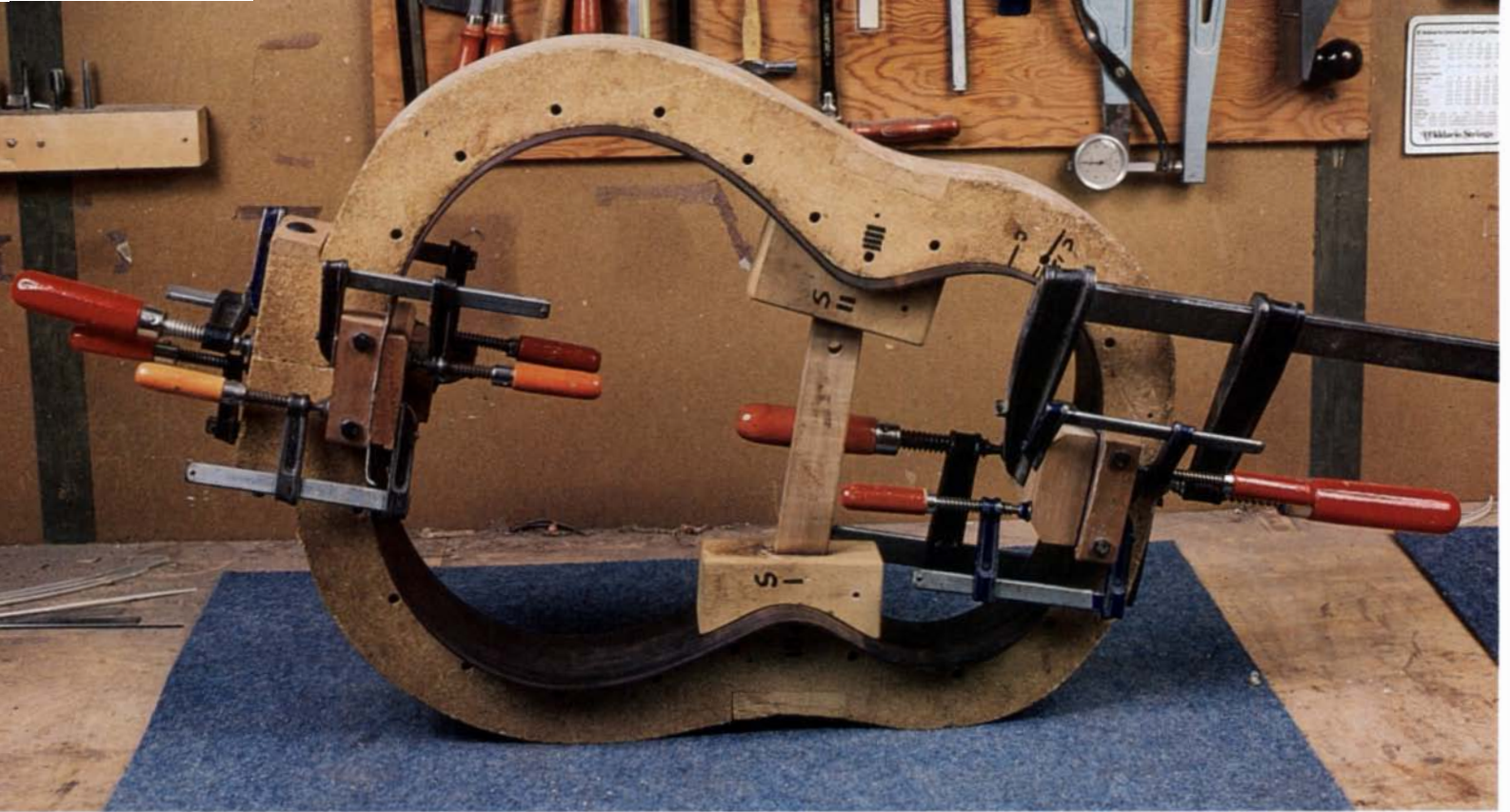
Guitar sides and blocks are clamped and glued in the mold. Shaped blocks at the waist, wedged apart by a stick, hold the pre-bent sides tight in place. Next the body will be tapered, as shown below, the neck block dovetailed, and linings added, as shown on p. 63.
