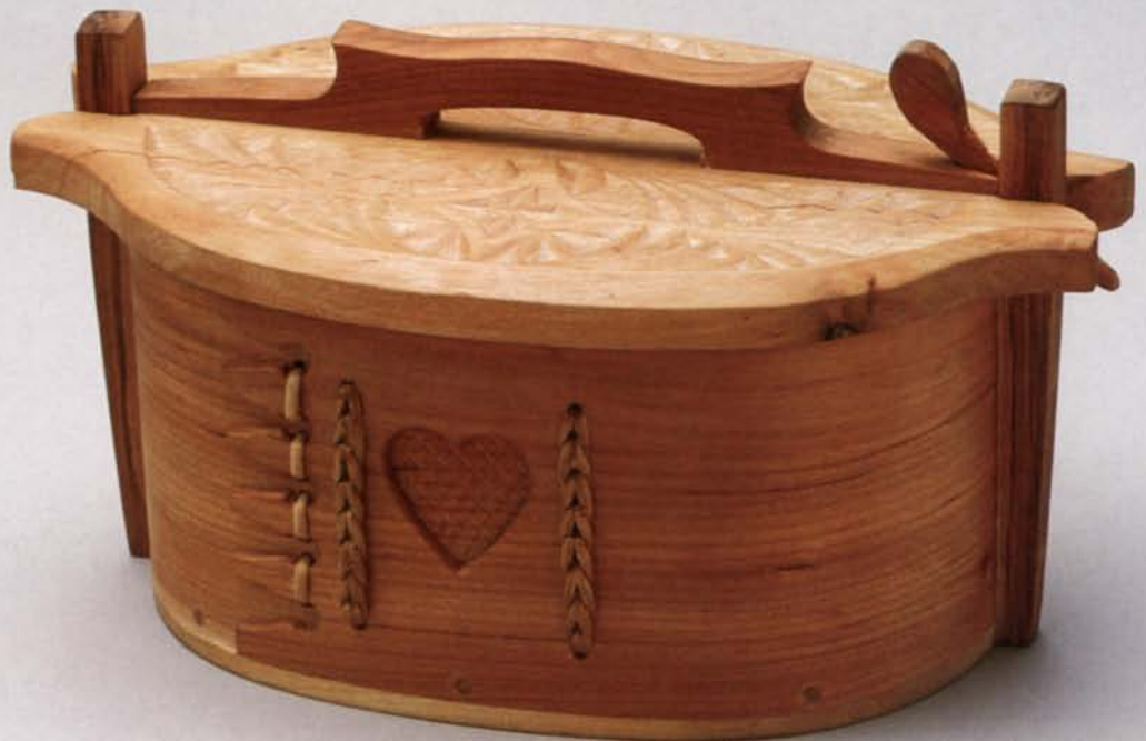
The outlines of the decorative fingers and the heart are drilled out and then finished with a sturdy woodworking knife. The box's body is suspended from a board clamped to the workbench.
