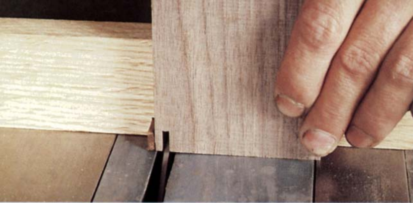
The finger-joint jig locates the spline one sawkerf from the blade so each cut leaves a finger equal to the blade width.
