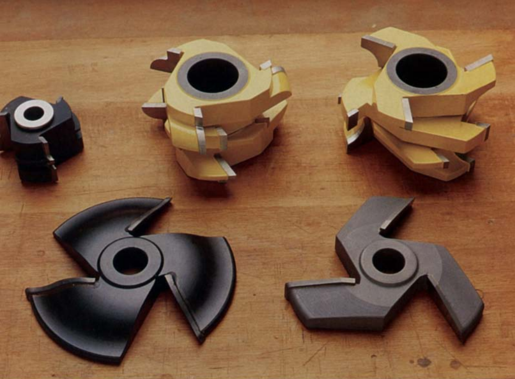
Specialty cuts range from interlocking patterns to wide beveled fields. Above, clockwise from top left: a carbide-tipped glue-joint cutter from Delta; a set of Tantung-tipped cope-and-pattern cutters from Freeborn; and two styles of panel raisers—one from DML that cuts a flat field and a second from F.S. Tool that creates a gently curved field.
