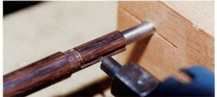
Cutting the groove for the locking pin is simple with this router arrangement. The pen barrel is pushed onto a guide rod, which fits snugly inside the barrel, as the bit cuts the groove. Twisting the barrel creates the final skewed section of the groove.
