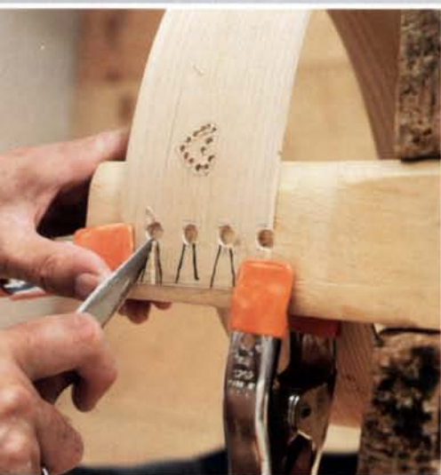
The outlines of the decorative fingers and the heart are drilled out and then finished with a sturdy woodworking knife. The box's body is suspended from a board clamped to the workbench.
