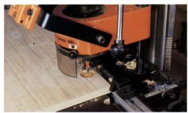
A low-cost drill-press attachment does double duty by boring three screw holes simultaneously and then pressing the hinge in place on the cabinet door.
