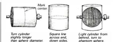
This approach leaves tiny defects that can be filled and sanded where the centers have dented each side. Reduce these defects by using a small spur center and a ball-bearing center.
