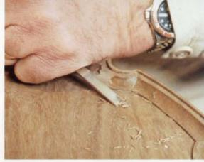
14. I've switched to a flat chisel here for paring away the gouge marks. Note the size of the chips and try to match them with your own tools. You must work in thousandths-of-an-inch—if you can't produce chips of this size, your chisel is dull. Check frequently with a small straightedge to be sure you don't go too deep.
