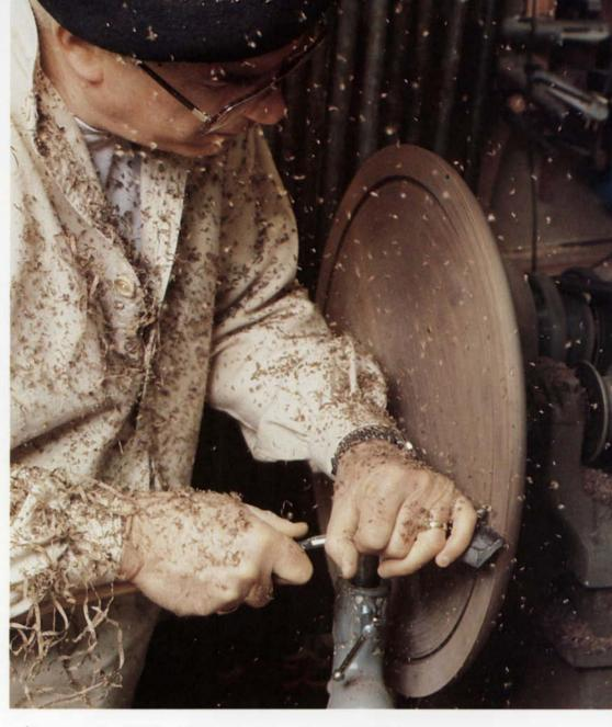
**4.** I turn the cove with a carbide-tipped scraper (soldered up for me by my favorite local machine shop) that has a profile like a flat little fingernail. This narrow profile allows me to fine-tune the shape of the cove until it exactly matches the profile of the gouge I'll use for the carving, as shown in the next step.
