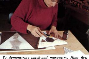
To demonstrate patch-pad marquetry, Hunt first transfers a crest design to posterboard with carbon paper, top left. Veneer segments for the individual marquetry components are then taped into "windows" cut in the posterboard, above left. Each poster-
