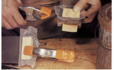
A loose tenon can be built out to fit its mortise by gluing on a piece of veneer or a strip of wood. Clamp the piece down with a wooden block protected from glue squeeze out by wax paper.
