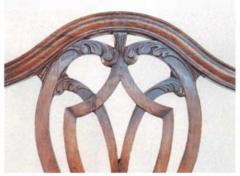
Weak cross grain on the crest rail of this old chair is prone to breakage, especially when it's mortised to accept the tenon of the chair back.
