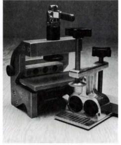
Doweling jigs for use with portable drills.
