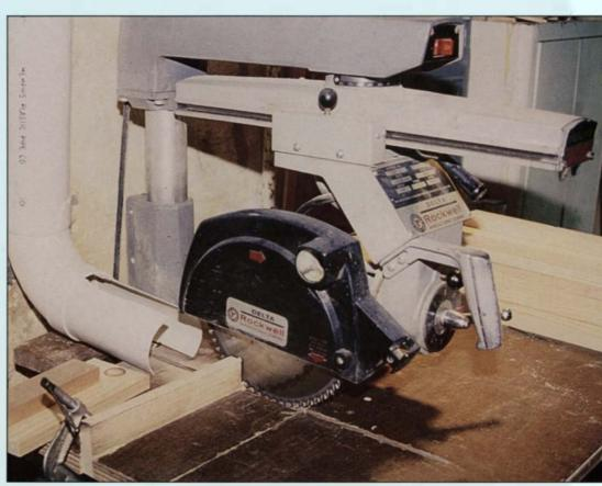
A plastic pipe pulls dust away from a radial-arm saw. More elaborate boods can be made from solid wood, plywood, plastic sheet or sheet metal.
