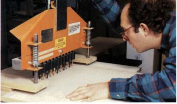
The author uses 12 of the 18 drills on his line-boring drill-press attachment to quickly bore rows of system holes on cabinet sides. The drill press's ingenious band drive rotates alternating drills clockwise and counterclockwise, thereby eliminating the need for elaborate gearing to drive the multiple spindles.
