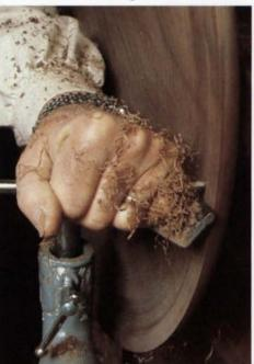
**5.** Check the profile of the cove by stopping the lathe and pressing the gouge—in this case a \(^8\)-in., #5 sweep—into the cove at the same angle as when you will be carving. The fit shown here is just right and matches the original table. Piecrusts superficially look alike, but each carver makes the cove to match his particular tools.
