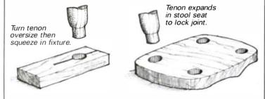
I make Windsor stools with legs that have tenons turned at the top to fit blind holes bored in the stool seat. These leg joints take a lot of stress, so I take pains to ensure the leg joint is tight. First, I turn the tenon slightly oversize, so its diameter is about ½4 in. too big for the hole. Then, before assembly, I compress the tenon with the fixture shown in the sketch, so it
