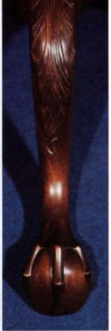
Because of the large diameter of Pine's mahogany interpretation of a Philadelphia-style tripod, the author dished the top with a router instead of on the lathe. Hand tools then leveled the surface and carved the piecrust design. The ball on the shaft can be left plain or be carved. In either case, it should be turned to the diam-
