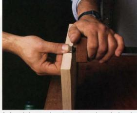
2. Stand the panel up in a vise and mark the edge that fits in the groove with a marking gauge. Set a marking gauge to the width of the groove and slide the gauge along the panel's back.
