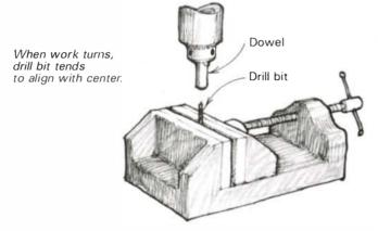
When you need to drill a longitudinal hole in a small dowel such as Jeris Chamey's box hinge (FWW #62), try this. Chuck the dowel in the drill press and hold the drill bit in the drill-press vise. When you lower the dowel on the bit, it will self-center and provide a quite accurately centered hole.
