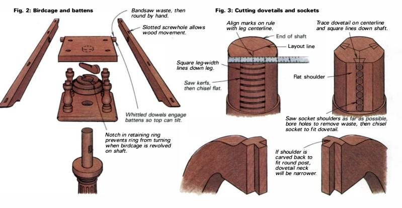
tabletop to revolve properly, the wedge should bottom out in its slot while just removing all slop from the ring and birdcage. The bottom of the slot must line up exactly with the top surface of the ring. If the slot is too high, the tabletop will rattle around; if the ring is too thick, the wedge will bind things up and the top won't turn at all. When you have things just right, trim the wedge to length and shape its ends.
