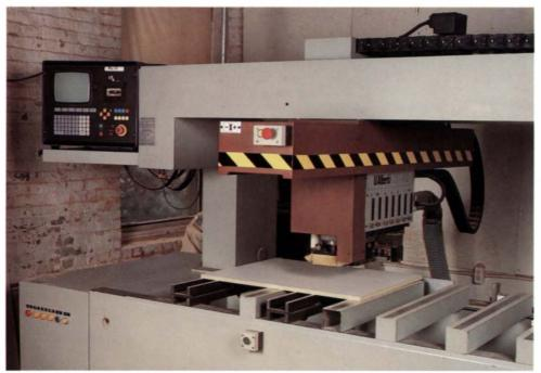
The key to automated 32mm production is the CNC milling machine. Its computer memory stores the complex patterns that allow the machine to perform hundreds of different boring and routing operations on cabinet parts.
