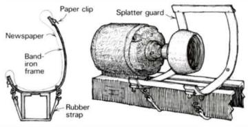
We welded together pieces of ½-in. by 1½-in. band iron for the shield's frame. The piece of band iron welded to the bottom serves as an index to locate the shield between the lathe's ways. We riveted a No. 2 Boston paper clip to each corner to hold a sheet of newspaper spread inside the shield. Finally, we attached two rubber tie-down straps to the rear of the shield. These straps are pulled under the lathe bed and hooked into rings on the front of the saddle to cinch the shield down.
