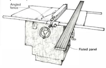
To cut the fluted panels, fix the angled fence on the rip fence and set the blade depth at about  $\frac{1}{8}$  in. It will take four passes, raising the blade  $\frac{1}{8}$  in. each pass, to cut the flute to its final depth of  $\frac{1}{8}$  in. After one flute has been completed, move the rip fence over, lower the blade and start another.
