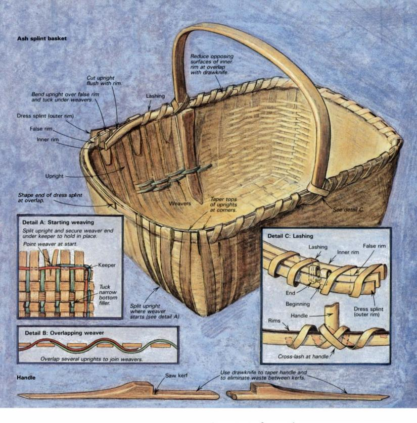
the top weaver and under the false rim. When you come to the handle, cross the lashing over its outside (see detail A, above). Stop lashing at the starting point. Coming from the inside of the basket, tuck the lash under the inner rim and bring it up between the inner rim and the false rim. Loop it over the top of the false rim and dress splint rim and pull it taut.
