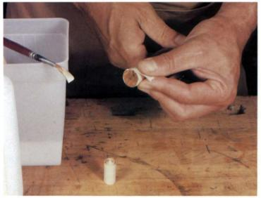
After being pulled tight to squeeze out excess glue, the curled plane shaving will hold its shape without clamps.
