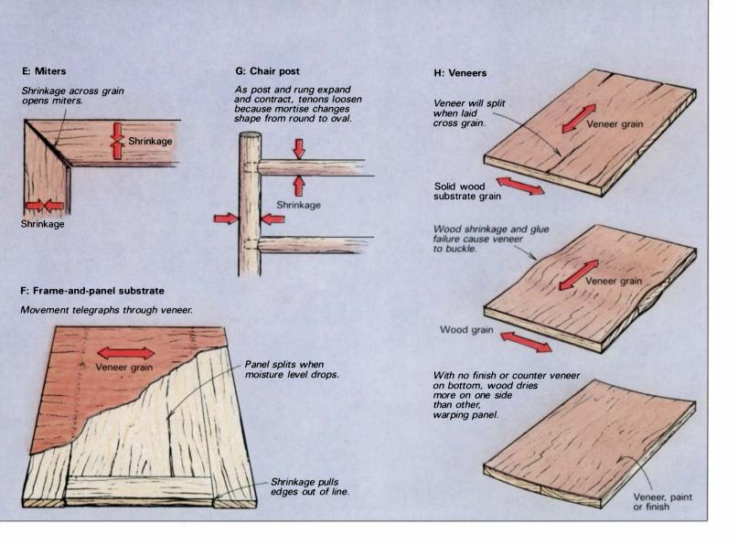
ture-related movements against the holding power of the glue. This wouldn't be such a problem if the shrinkage during dry periods and swelling during the damper months occurred uniformly in all directions. But, the movement is in one direction only: across the grain. There's virtually no movement along the grain. When boards are joined at right angles, the contrary shrinkage and expansion stresses the glue joint and causes it to eventually fail.
