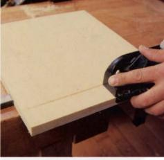
3. A rabbet plane cuts the perimeter of the raised field. The scrap clamped to the edge of the piece prevents tearout when planing across the grain.
