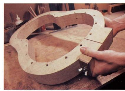
To ensure symmetry and uniformity, guitars are usually built in a mold. Laskin's mold can be loosened at the bottom so the sides can be slipped out without damage.
