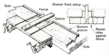
To rout the male dovetails, I use a tall fence on my router table with the router attached to the back of the fence and the bit running parallel to the table. I recommend cutting one side of the dovetail on all the pieces, then resetting the fence and cutting the other side with the same face against the table as before. The principle of always working relative to one face will ensure that all dovetails will be the same size.
