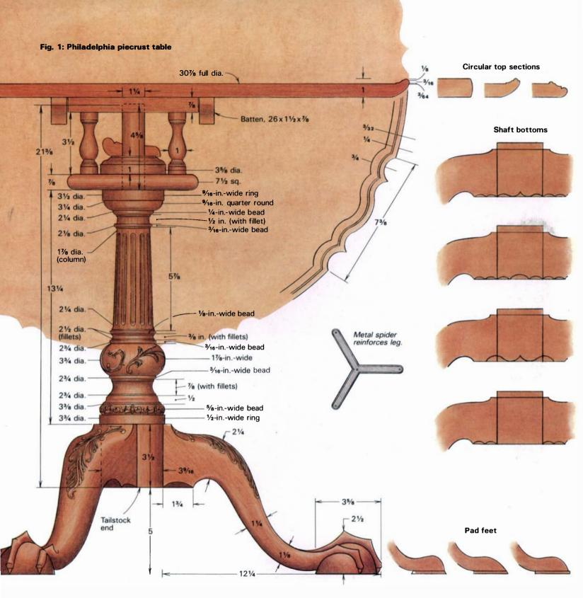
in turning the area of the shaft where the legs will join. This section must be perfectly cylindrical—any taper will affect the stance of the legs. Turn both ends of the shaft and the ledge where the birdcage will rest flat and square to the axis of the shaft. Wait until the legs are fitted to the shaft before doing any carving or fluting. This will decrease the likelihood of damaging fine details while driving legs into and out of their sockets.
