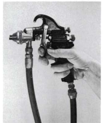
Morris demonstrates the proper relative distance from and angle to the surface being sprayed. Hand-holding the guitar allows more sensitive positioning in relation to the light. He's using a full-size DeVilbiss type JGA gun, siphon-fed from a quart cup, which is suitable for spraying large objects without the need for frequent refills. DeVilbiss type EGA gun, top right, is right for objects the size of a guitar and smaller. Its cup can be replaced with a small mayonnaise jar, permitting quick color changes. The Binks model 18 gun, right, has a pressure-fed hose instead of a cup. The hose supplies lacquer under 10 PSI from a 2-gal. holding tank. Such a system is light, versatile (it can even be used upside down) and good for production work. At top, an edge-grain section of a piece of lacquered rose wood at x28 magnification shows its enormous pores and the filler (white at upper right) under the finish. The lacquer film tapers in thickness toward the corner because the film shrinks as it dries.
