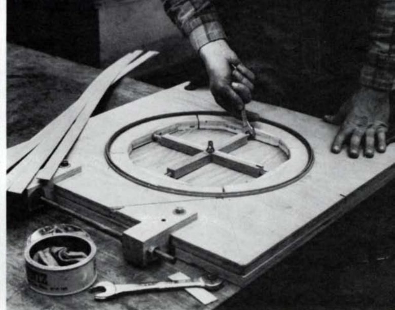
Mattson uses a dielectric glue drier, left, to speed laminating the spokes, 16 of which are required in this design. At right, he applies clamping pressure to the laminates that will form the rim of the lamp.
