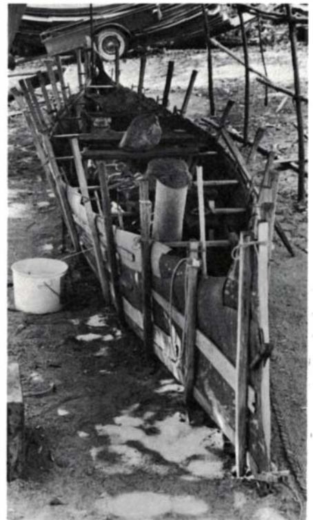
Kanawa Museum curator Rick Nash is building this 20-ft. birchbark in the traditional way—between stakes and a form weighted to the ground with rocks.
