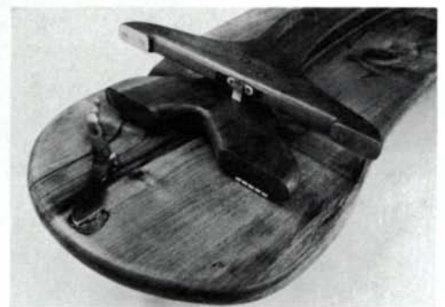
Unusual function and flawed materials can be inspiring design parameters. This cherry table, made to fit over an upholstered armchair, includes homemade brass hardware (at left and above) that allows the legs to fold for storage. A router produced the flat surface of the tabletop, leaving a decorative and functional scalloped rim (at top) and salvaging a thin, warped, otherwise useless plank.
