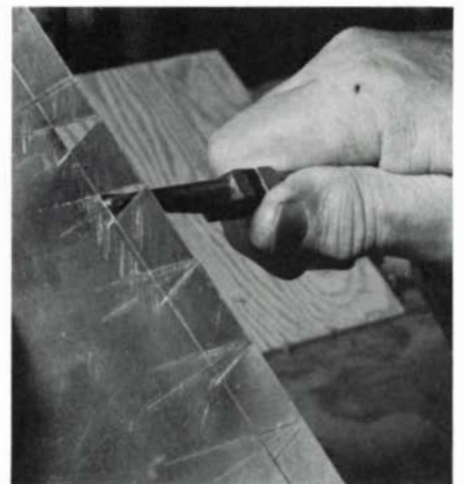
C. Breaking out the waste.
