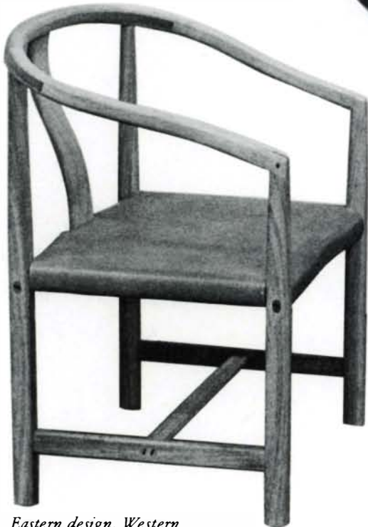
Eastern design, Western joinery mark this chair by Sat Rattan Singh Khalsa. Made of teak and iroko, it has a cowhide seat, and its rails are brought through the posts with wedged tenons. Instead of the traditional keyed scarf joint to connect the arms and back rail, Khalsa used long, open mortise-and-tenon joints.
