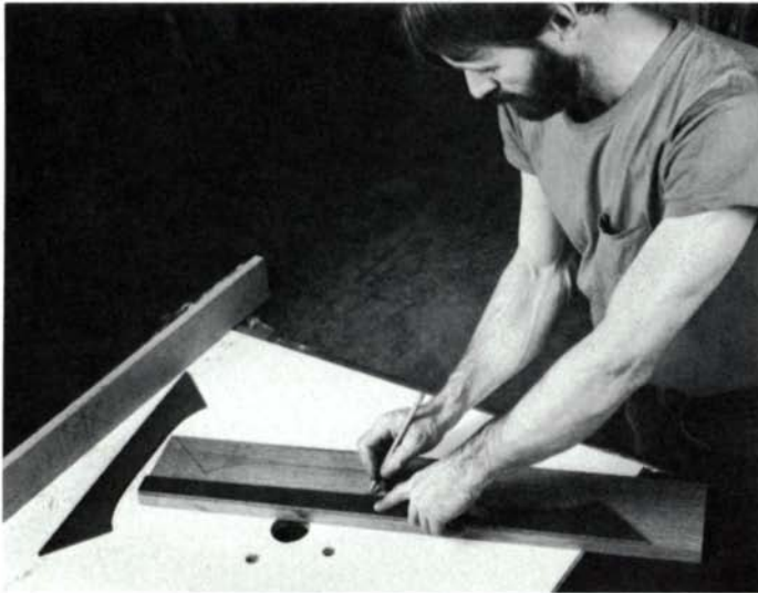
A. Author traces interior curve and taper of half a leg from Masonite pattern. Only one apron pattern is needed, since the line between the curves can be lengthened or shortened as required. Straight side of the pattern must be registered along a jointed edge of the stock.
