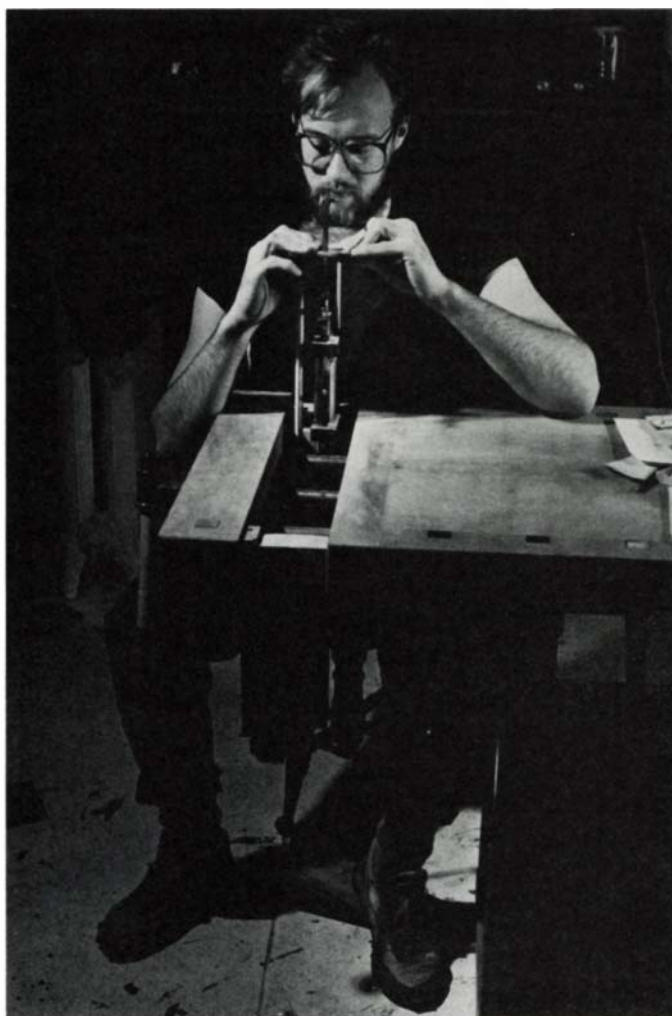
Foot-powered jigsaw designed especially for cutting delicate mother-of-pearl and abalone is mounted in the bench vise. A drawing of Parker's jigsaw appears on the following page.
