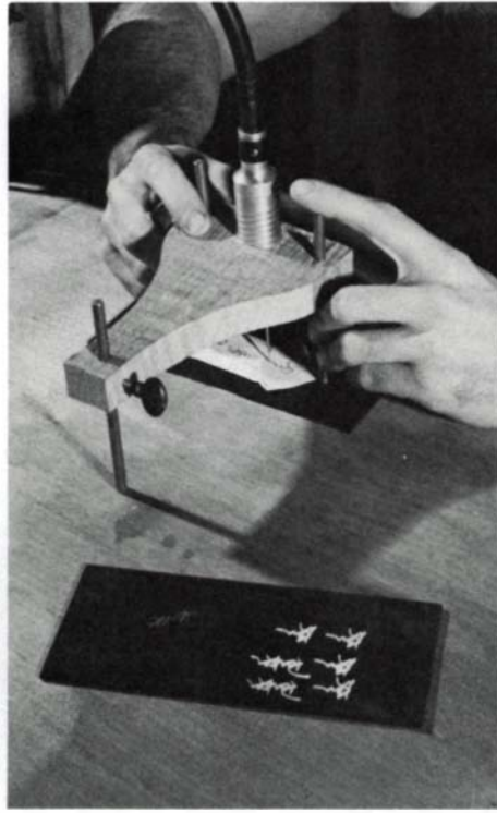
Parker's design allows a comfortable working posture, sensitive control of the stroke and a good view of the work. Thin, narrow sawtable, left, allows work to be held down securely between fingers and thumbs. Center, Parker cuts the mortise for his mother-of-pearl signature (0.030 in. wide) using a Foredom mounted in a simple, adjustable-leg tripod.
