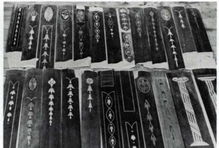
Jason French's work includes banding, left, and face veneers for square-tapered legs, right. Note that these are samples and that the leg veneers would run the entire length of the leg, including the border line, which is sawn.
