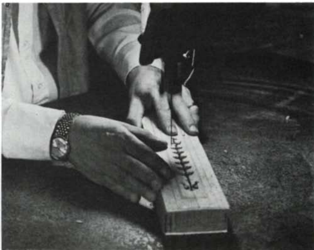
Jason French saws a sandwich of 16 veneers for fan inlay parts. The dotted line is pounce, a powdered asphaltum applied through perforations in the master pattern.
