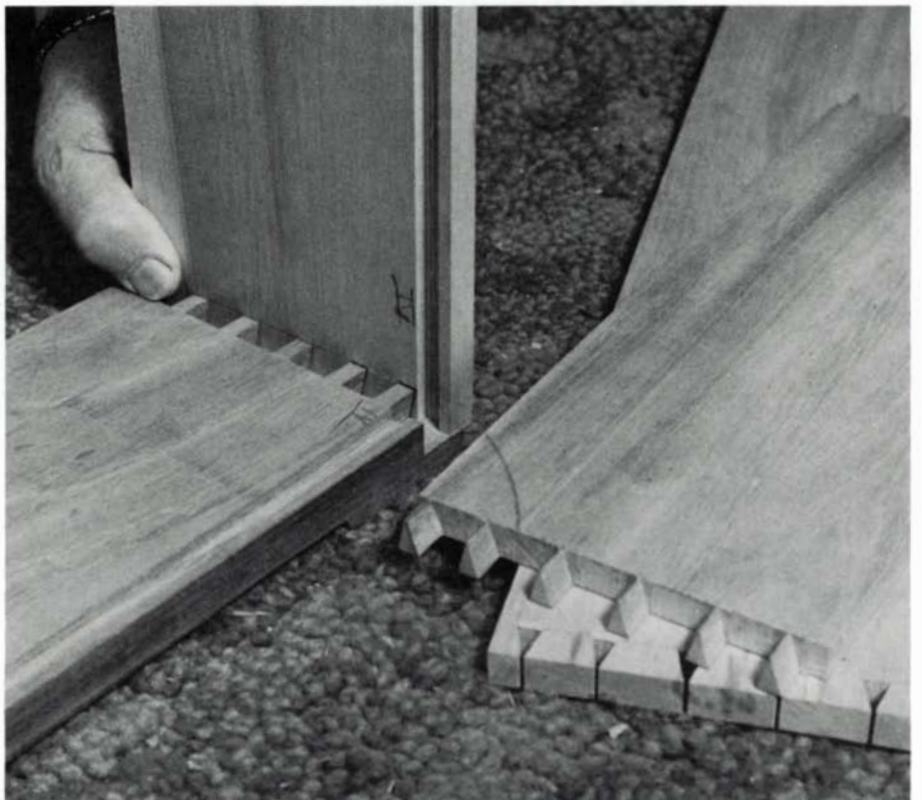
L. The completed joint.
