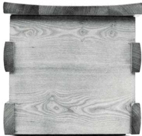
Ash chest, top and above, 60 in. by 20 in. by 16 in., is one of Peters' favorite pieces. 'I didn't want this chest to be a clever piece peppered with dovetails. It's going into a medieval house, and I just wanted the chunkiness, the shape. The corners are mitered with a spline.'
