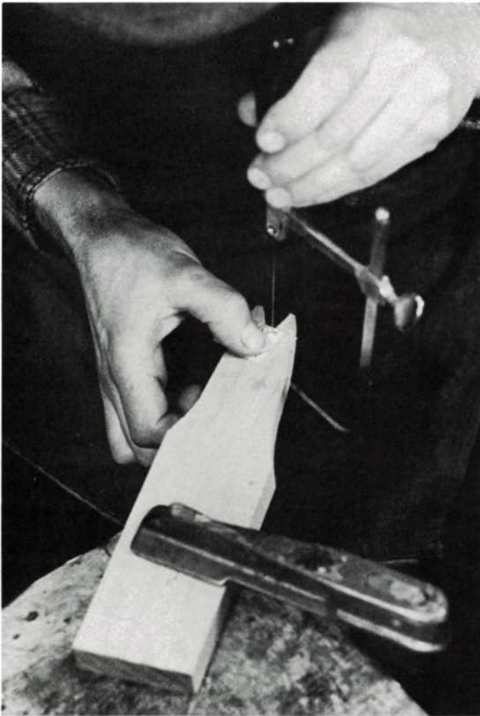
Very fragile and brittle, pearl must be sawn with a studied technique and special care. Left, with jeweler's saw and bird's mouth (the V-notched board clamped to his bench), Newman cuts a mythical sea beast from a mother-of-pearl chip. Top right, Dremel equipped with a tiny end mill routs the recess for the pearl inlay. It must fit easily, but with no gaps. Center, Newman uses an engraver's block to hold the stock when incising detail into the pearl. Engraver's blocks are necessary for good results, since engraving requires moving the work into the tool rather than the other way around, as is the case with carving wood. Engraved gouges filled with epoxy/aniline dye mixture delineate details and add depth to the finished dolphin (about twice actual size), right. Newman used black dye, but other colors would work as well.
