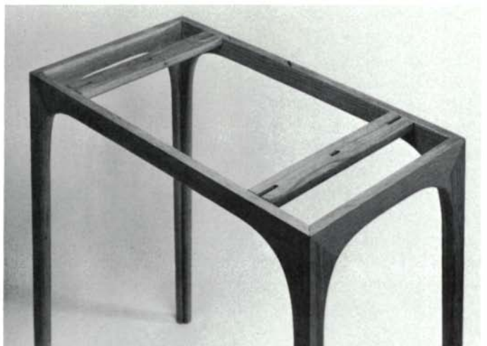
D. Tabletop support stringers are slotted for screws and mortised into the ends of the long aprons. Screw slots allow the top to expand and contract without bowing or cupping. Mortises are routed before table frame is completely assembled.
