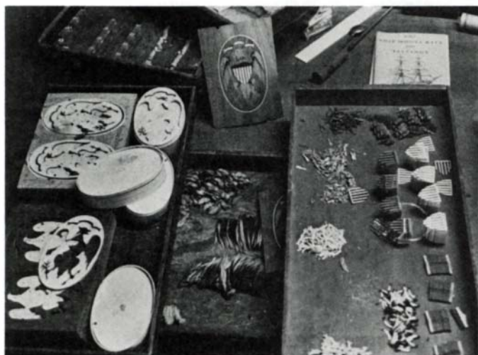
Marquetry inserts at Dover Inlay like the sunburst, top, are assembled on a light-tack tape. Above, an American eagle in all its parts.
