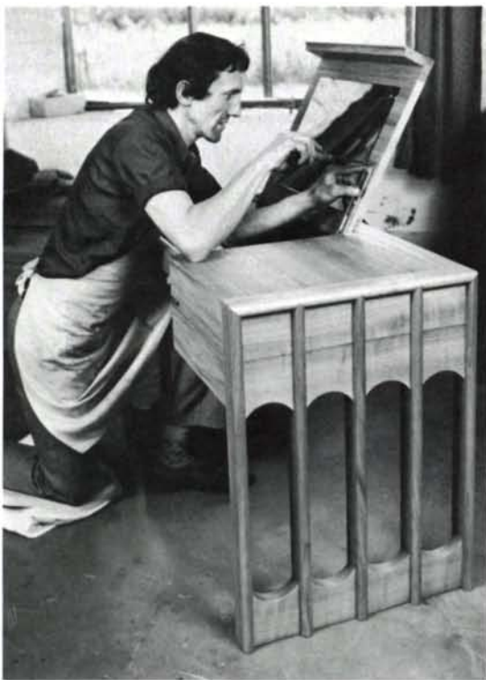
Above, small writing desk in the Chinese Gothic idiom is constructed with a mixture of solid wood and veneers. Peters felt it was risky to make the arches out of solid wood because there would have been 9 in. of grain to move. The hinged flap also is veneer construction. Says Peters, 'I know the weakness of veneers and try to have a good solid lipping wherever I can.' Photo: Council for Small Industries in Rural Areas. At right, lumber cut roughly to shape for future projects is stacked in the upper part of Peters' shop. The heat is kept on all winter. 'In effect,' says Peters, 'we do our own kiln drying.' Photo: © Robson 1980.
