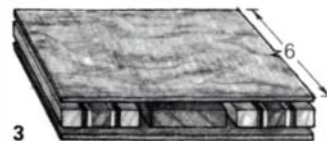
Glue components between veneers (3), and saw into strips (4).
