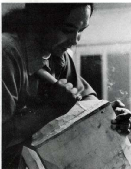
Kwakiutl Roy Hanuse recesses the fourth corner of a steamed and kerf-bent box with a specially designed hooked knife. The kerf-bending tools and traditional techniques of the Indians of the Northwest Coast are described on pp. 36-43; how Hanuse made this box, also shown on the cover, is detailed in a photo-essay, pp. 44-45. Photo: Ulli Steltzer.
