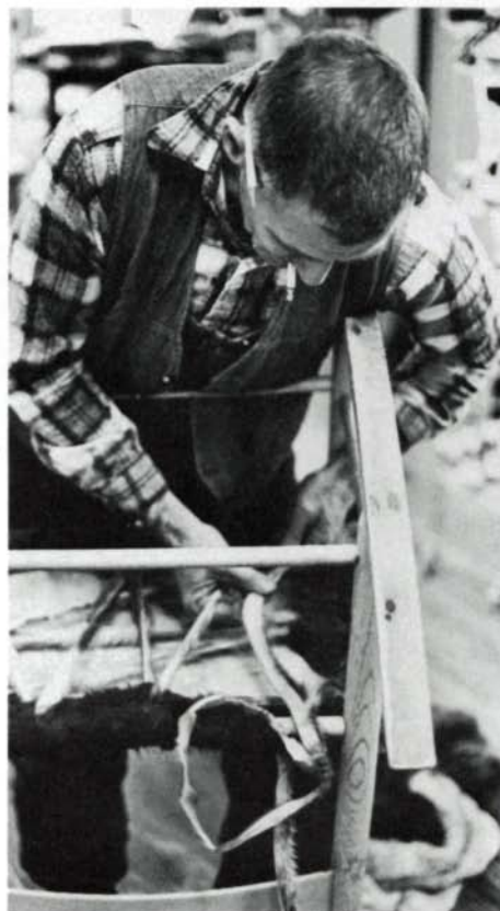
From cured hide to durable seat: a lacing thong is cut from the hide in a continuous half-inch strip (top center). The seat is positioned by fitting the hide around the front posts (top right), then it's laced from side to side (left) and trimmed around the back posts (above). Lacing continues from front to back until the seat is tight.
