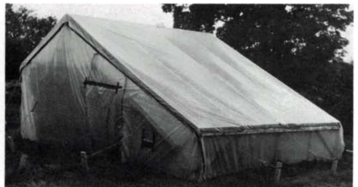
The Oxford kiln with rafters and polyethylene tent yet to be mounted, left, and in operation, right, is light enough to be carried by two or three people from one stack to another. It was designed for use in energy-poor countries.
