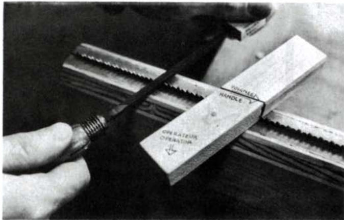
Crosscut-saw filing is aided by a bearing guide on the saw and a tilting guide on the file. Maintain consistent pressure for an equal number of strokes in each gullet, with a tooth set toward you always closest to the saw handle.
