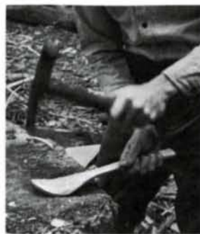
From log to finished utensil. Dustin begins by splitting a white oak crotch with froe and club, top. After rough-shaping with a hatchet, the spoon blank, left, still retains the basic shape of the branch. Next the bowl of the spoon is hollowed with a sculptor's adze, a gouge and a hook knife. Finished spoons, below, are of various woods, including mountain laurel, lilac, apple, butternut, walnut, cherry and cherry dogwood. Right, Dustin's mummified fruit-skin pots, baked in an oven and sealed with oil and beeswax.
