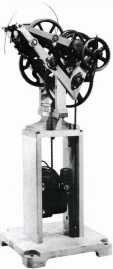
Clock #1, by William Bellows, is driven by the weight of its electric motor. It's 66 in. high.
