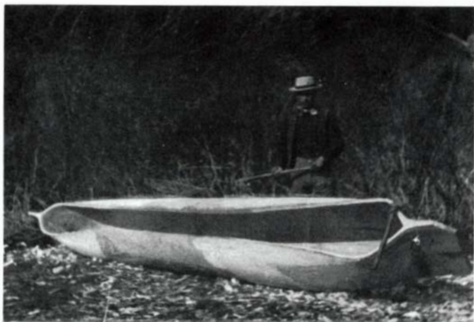
A medium-sized canoe, hollowed out but not yet filled with boiling water for spreading to final shape. Photo was taken in 1902 by C.F. Newcombe, courtesy British Columbia Provincial Museum, Victoria.
