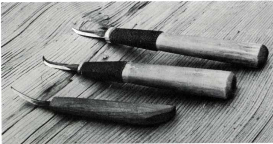
From left: double-curved knife, hooked blade, and slightly curved knife. Right, double-curved knife smooths an eye socket.
