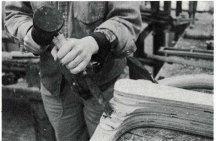
When side has been shaped and four layers added to start the seat, gouge and Surform remove the stair-steps.
