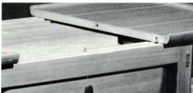
Patternmaker's locating pins, left, index cutting board and center leaf. Male pin, below, is set into center of front rail and a notch is cut into sliding leaves to conceal it. Button magnet at center of leaf edge keeps movable parts together. Bullet catches concealed in the ways control the extension of leaves.
