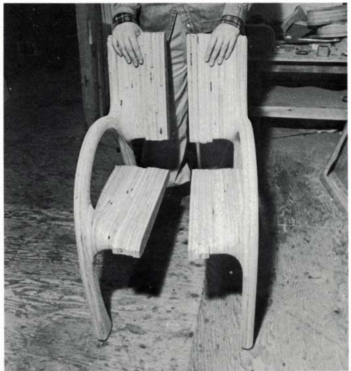
A wedge-shaped section will join the two halves, with dowels for reinforcement because the seat is supported only at the front.
