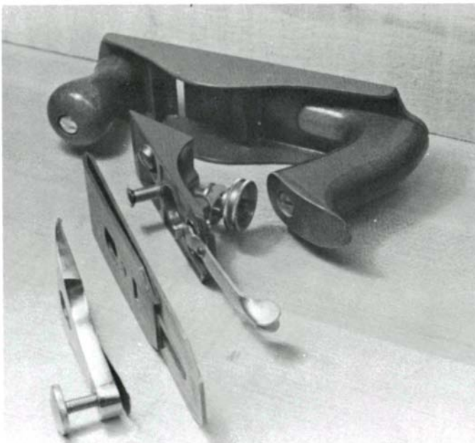
A partially disassembled smooth plane. The all-important adjustable frog is between the iron and the plane body. In a block plane, there is no frog; the iron rests on the plane body and a moveable toe plate adjusts the blade opening.
