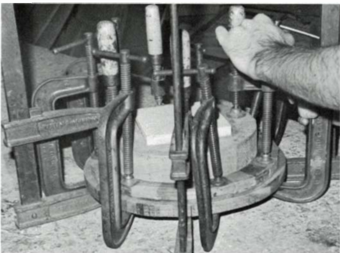
Checked ring is touched with sander to make sure it's flat; then it's glued between the two-inch teak base block and the one-inch walnut board that will form the top rim.
