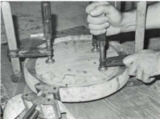
Tourniquet clamp holds glued segments together while two plywood disks protected by waxed paper are clamped to hold checkered ring flat between them.
