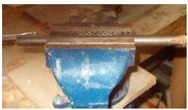
Here are a couple of shots of the receiving platform ground to about the half way part of the rod and about 7/8" long.
