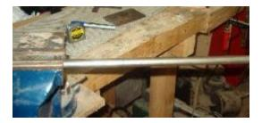
Next I mounted a piece of 5/8" cold rolled steel rod and measured to cut off about 10".
