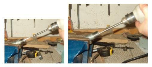
Insert the set screws and assemble tightly the extension to an elbow to the 2" nipple to an elbow to the 4" nipple. You do not want these to rotate under use so tighten hard. Some thin CA trickled into the joints can not hurt.
