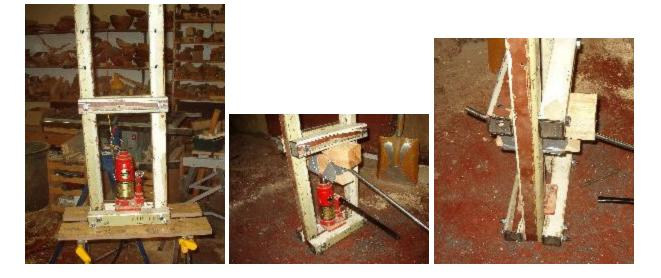
In goes the steel and the jack is slowly raised for the first bend. Some careful positioning and the second bend is accomplished. Then I checked it with my sketch and realized a bit of tweaking was needed. I decided to bend it a bit at the point where the arrow directs.
