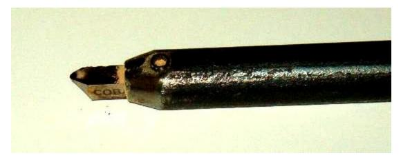
As you can see I have drilled and tapped for a set screw about 1/2" behind the tip. I find this sufficient to hold the tip in place although you might want to put another set screw about 1/2" behind the first. Out of habit I use 6mm x 1 set screws but 1/4" x 20 would work as well. I have also ground the end of the shaft back to give a bit more clearance for the cuts. The tip is ground to about 45 degrees and is usually more rounded than I have it
