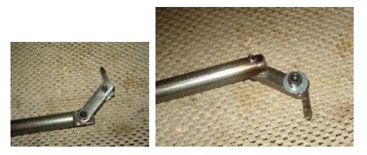
Finally, here it is mounted in a home made arm brace, ready to be used. Any hollowing tool with the cutting tip so far from the angle of rotation will have a lot of torque so an arm brace helps to give control.
