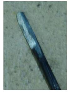
Now to the grinder. I want a hook with an inside bevel for the particular cuts I am about to make. An outside bevel is usual and the one I use the most. As you look at the nail with edge up ward, for an outside bevel grind it on the left, for an inside grind it on the right. Here it is ground on the right. I first grind the edges straight, then the sides flat, then the bevel to about 45 degrees.
