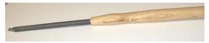
This is a shot of my 1/4" Oland Tool. Note that this is a working tool and nothing was done to make it fancy for sale. I turned a handle about 14" long and drilled a 5/8 hole about 2 1/2" deep into it. The shaft is cold rolled steel with about 10" extended from the handle. The tip is a 1/4" x 2 1/2" HSS cutting tool, standard in the metal lathe industry.
