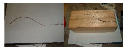
The sketch was transferred to a block of maple and cut out on the bandsaw
