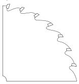
For cutting with (parallel to) the grain. Requires fewer and larger teeth than crosscut blades. Cut is relatively rough. Blade shown is carbidetipped.
