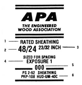
This grade mark can vary a bit, but in general includes (1) the panel grade designation, (2) the span rating, (3) the thickness, (4) the exposure durability classification, (5) the lumber mill that produced the panel (shown as a number) and (6) the applicable product standard.
