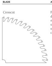
For cutting across the grain or at a diagonal. Has more teeth than rip or combination blades, resulting in a smoother cut with a minimum of splintering. Blade shown is carbide-tipped.
