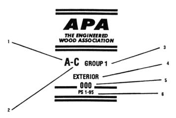
The grade mark for plywood, identified by the face and back veneer grades, includes (1) the grade of the face veneer, (2) the grade of the back veneer, (3) the species group number, (4) the exposure durability classification, (5) the lumber mill that produced the panel (shown as a number) and (6) the applicable product standard.
