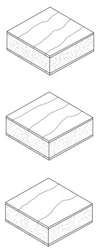
Particleboard Core: A particleboard core with hardwood veneer on each face
