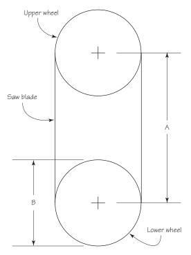
Note: Before measuring dimension A, locate the adjustable upper (tension) wheel so that it is midway between the fully up and fully down positions.
