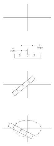
1. Draw a horizontal line slightly longer than the length of the ellipse, then draw a vertical line slightly longer than the ellipse width. Make sure the lines are perpendicular to each other.
