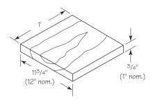
Several formulas are used to calculate board feet, but the one most often used is as follows:
