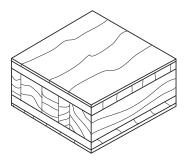
Lumber Core: Made from three, five or seven plies of edge-glued solid lumber; may be either hardwood or softwood; species mixing not allowed. Grades available are Clear, Sound and Regular. A Regular grade clearedge version is available with edge strips at least 1<sup>1</sup>/2" wide to facilitate edge molding and shaping
