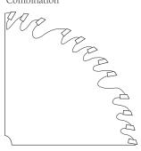
For both crosscutting and ripping. The number and size of the teeth are a compromise between the crosscut and rip blade designs. Eliminates having to constantly change from rip blade to crosscut blade. A good general-purpose blade for all cuts, but it doesn't rip as well as a rip blade or crosscut as well as a crosscut blade. Blade shown is carbide-tipped.
