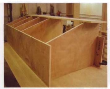
Begin with the corner units. You'll notice that they are not symmetrical. This is because the units on the long wall are 12" (305mm) deep, but the units on the short walls where the clothes rods go are 16" (406mm) deep to accommodate hanging garments. This doesn't pose any problems in construction but it is an important aspect of the design. The shelves are fixed into place with screws. Note: It is a lot easier to edge-band the shelves before assembling the corner units.
