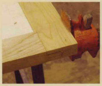
Once the glue has cured, you can sand the face of the door frame and its edges. I don't sand the panel once it has been enclosed in the frame, as it is harder to sand evenly. Depending on the overall style and look you're going for, you can rout the outside edges of the door on a router table or with a hand-held router.
