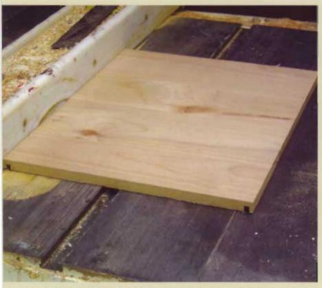
I cut a dado into each side panel near the ends, where the front and back panels will attach.
