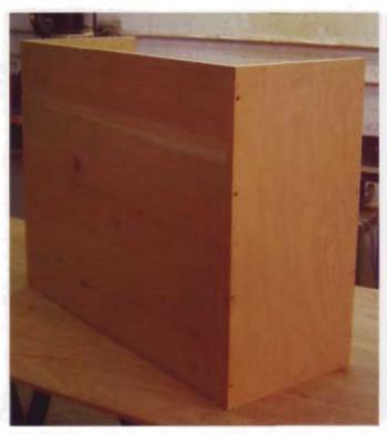
Build the single drawer box and install the cabinet side runners in it. I positioned the front corner of the runners 1/2" (13mm) above the cabinet bottom.
