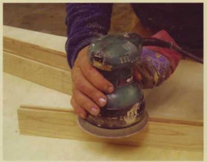
Prior to assembly, I recommend making sure the inside faces of the stiles and rails have been sanded smooth. Once the door is assembled it is very difficult to sand these areas.
