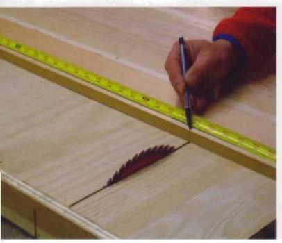
Cut the end panels first. They are the largest components and the smaller pieces can later be fabricated from their offcuts. Then cut all the other 3/4" (19mm) cherry parts.
