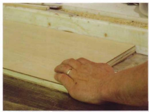
The sides, top and bottom are all grooved to hold the 1/4" (6mm) oak plywood back. I used a router table and a straight-cutting bit.
