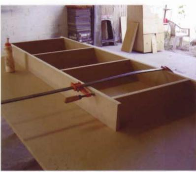
The cabinet boxes sit on a single base. It measures 4<sup>1</sup>/<sub>2</sub>" (114mm) high and spans almost the entire footprint of the niche. I set the sides in about 1" (25mm), just in case the front and back of the base needs to be trimmed for a precise fit. Position the center supports evenly across the interior of the base.
