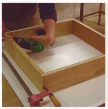
I built the base for the tall drawer cabinet from scrap plywood.
