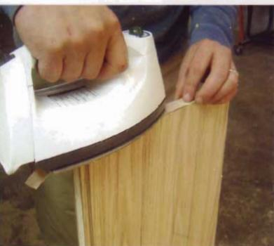
Once the groove has been cut, edge-band the parts. This sequence is important because the edge-banding covers up the groove that shows through on the ends of the plywood.
