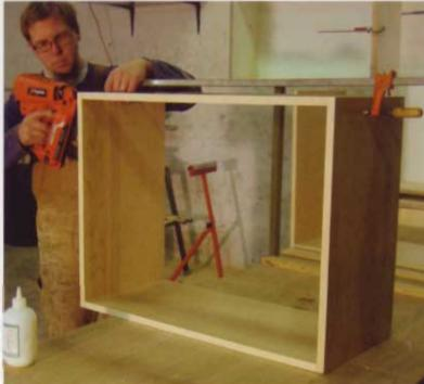
The layout of some of these cabinets allows a few shortcuts in their construction. You'll notice that the sides of cabinets B,C,E and F are not exposed. This means you can save some time by just nailing or screwing the cases together.
