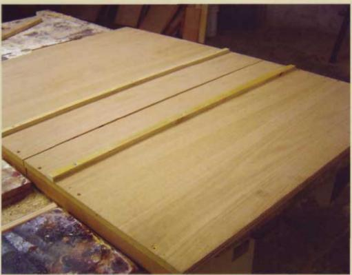
You'll want to start by milling two strips of hardwood that fit into the grooves on the table-saw top—they should move easily from front to back, but they should have very little side to side movement. The strips should be about 1/16" (2mm) higher than the table-saw top.
