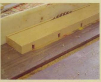
The depth of the dadoes should equal half the height of the block of wood. Once the notches are done, you can put a regular blade back on the table saw and rip the block of wood into 1/4" (6mm) strips.
