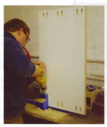
I used pocket screws to hold the bottom in place. I chose pocket screws because I wanted the exposed screw heads on the bottom right side of the piece to be concealed. Fastcap self-stick screw head covers would've helped, but pocket screws are equally quick and look even better.
