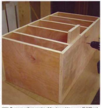
To assure uniform spacing of the shoe cubbies, use a 5" (127mm) spacer. The highest shelf is slightly shorter.
