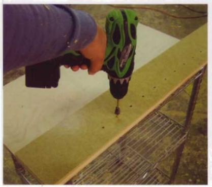
The cabinet parts require some work prior to assembly. You can do the edge-banding now or later, but I find it easier to drill the shelf-peg holes early on in the process.
