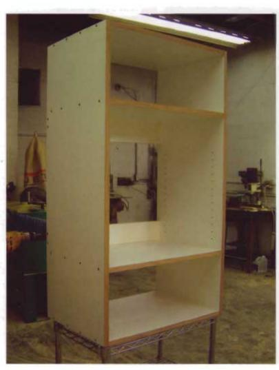
The back wall stretchers provide a place to screw the cabinet into the studs in the wall. I placed them inside the portion of cabinet that will be hidden by the doors. Doing so makes for a less cluttered look when the cabinet is installed.
