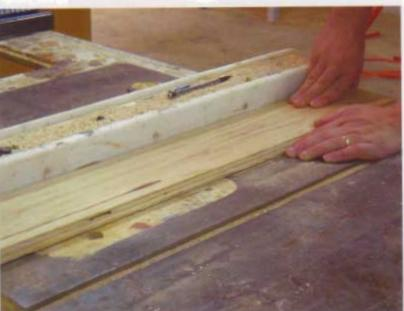
The tower is composed of two end panels connected with stretchers. The stretchers are ripped from 3/4" (19mm) cherry plywood and edge-banded on their long edges.
