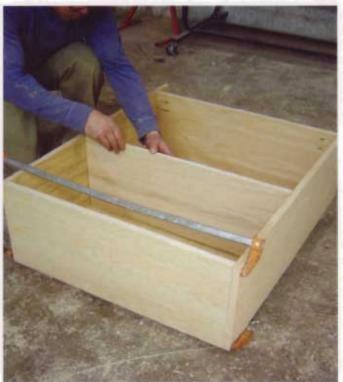
The center shelf is installed with pocket screws. Measure up 21<sup>1</sup>/<sub>4</sub>" (540mm) from the bottom edge of the side panels and align the top side of the shelf accordingly.
