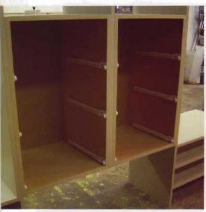
I used three-quarter extension drawer slides for this project. Install the cabinet-side slides in the cabinets first.
