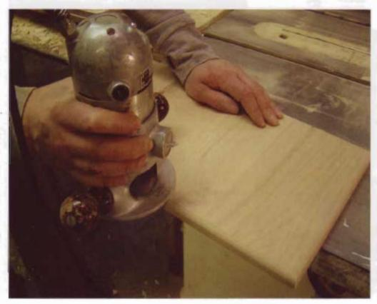
I detailed the front edges of the MDF drawer fronts using a 3/e" (10mm) roundover bit. This detail looks nice and eliminates the chipping that often occurs on edges left at 90°. Drawer fronts can be a high-wear area.
