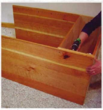
The shoe cubbies above the single drawer unit are made with two short end panels attached to the sides of the drawer box. I ran screws front the inside and the outside the box for maximum holding power.
