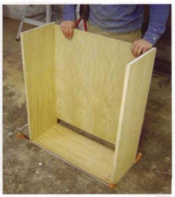
The back should slide in easily without excess force. Test-fit prior to applying the glue.
