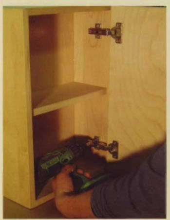
With the mounting plate clicked onto the hinge cup, position the door at its correct height for mounting. I leave a <sup>1</sup>/<sub>a</sub>" (3mm) gap between the door and front of the cabinet (I just eyeball it, but you could tape a spacer to the edge of the door and then press it tightly into place). Using a pen, or fine marker, mark the locations of the mounting plate holes on the inside of the cabinet. A few screws will secure the door.
