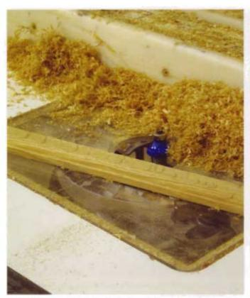
I made a matched pair of edged-panel drawer fronts for this piece. I created the molding profile with a <sup>1</sup>/<sub>4</sub>" (6mm) roundover bit. The bottom edge of the cutter was raised to 1 <sup>1</sup>/<sub>16</sub>" (27mm) below the top of the router table. For more details on this construction method, see Beyond the Basic Box.
