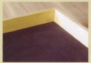
A jewelry drawer starts out like any regular drawer, built in the usual manner. The velvet bottom is made by wrapping a 1/4"-thick (6mm) piece of plywood with velvet. I use a spray adhesive on the underside of the false bottom to secure the velvet.
