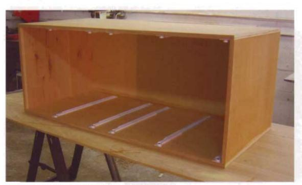
The drawer slides separate into two halves: the cabinet side runner and the drawer rail. In addition, the parts are assigned to either the right of left side of the drawer. The cabinet side runners screw directly onto the inside face of the cabinet sides. To locate the positions of the cabinet side runners, refer to the drawing on page 31.
