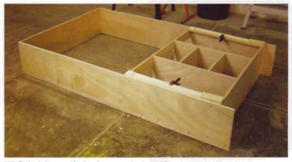
The header has several functions: it serves as a place to mount the overhead lights, it provides a place to securely fasten the crown molding and it helps to create a more built-in look.
