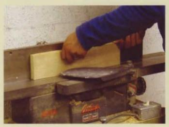
Once you have an accurate measurement for the finished door, you can start to make a list of the parts you'll need. A frame and panel door is usually comprised of five parts: a center panel, generally 1/4" (6mm) thick, and a solid wood frame, which consists of two vertical stiles and two horizontal rails. I usually mill an extra frame part or two because it doesn't take much extra time, and it will be well worth it if you make a mistake later on and need a replacement.
