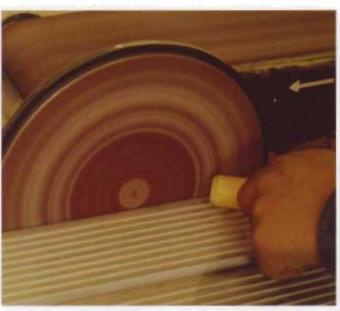
I recommend sanding the exposed ends of the dowels on a disc sander. This creates a more finished look and also prevents the ends from splintering in the future.
