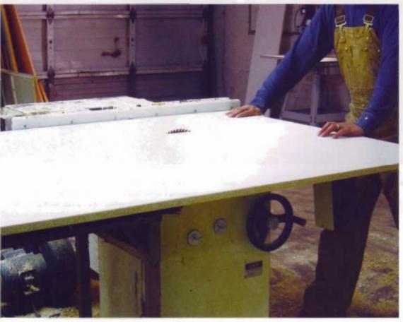
Build the smaller, wall-hung cabinet first. I cut the parts to size using my table saw and a blade specifically meant for cutting melamine. While most any combination blade will provide acceptable results, melamine-specific blades tend to produce the smallest amount of tear-out.
