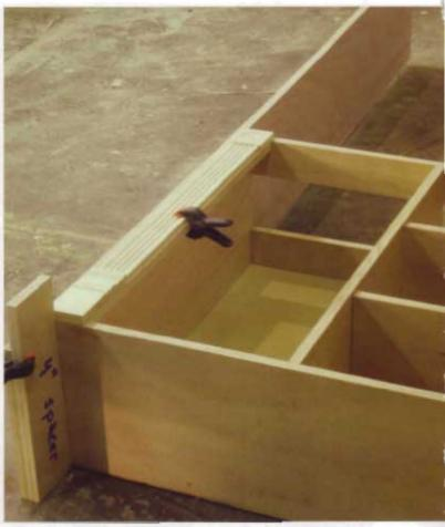
The end panels are screwed directly to the cabinet. The screw heads won't show if you screw from the outside because other cabinets will cover them later. Use a 4" (102mm) spacer to postion the end panels accurately.
