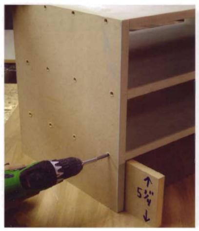
Painting the parts of the shoe cubbles prior to assembly is a must—the tight corners and small spaces are really tough to finish otherwise. When the paint was dry, I used a 51/4" (133mm) spacer to align the shelves consistenty. After the assembly is complete, sand the joints and touch them up as needed.
