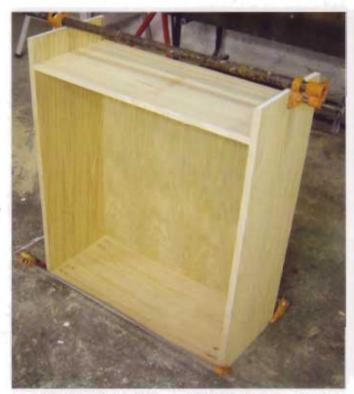
The bottom is sandwiched between the sides, just like the top. To position it correctly, measure down 3" (76mm) from the bottom edge of the sides and make a couple of small marks in pencil.
