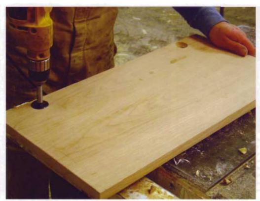
I made the doors from some scrap cherry plywood. (You can use the species of wood you desire.) Use a 13/6" (35mm) Forstner bit to drill the hinge holes 4" (102mm) from the top and bottom edges of the doors, and 13/16" (21mm) in from the edges.
