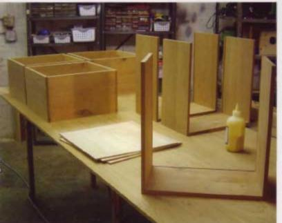
These fairly simple drawers are built with 1/2" (13mm) material that's glued and nailed at the corners. The bottoms fit into a groove I ripped near the bottom edge of the drawer stock.
