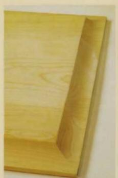
If you'd like to make a true raised-panel door, the same process applies. Instead of the plywood center panel, though, you'll need to glue up a solid wood panel about <sup>5</sup>/a" (16mm) thick. Once it has been squared up and sanded, you can run it across your router table equipped with a panel raising bit.
