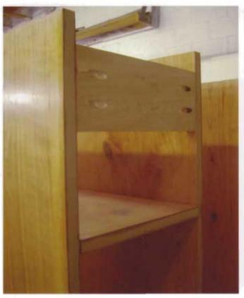
The third stretcher is placed at the top of the tower, on the back side. During the installation, you'll screw the tower to the wall through this stretcher.
