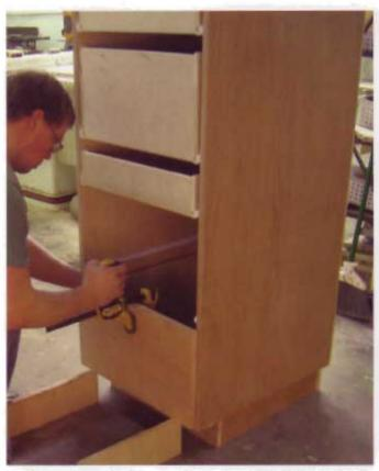
These drawer fronts are simple to make, but a bit tricky to attach. Starting with the tall drawer cabinet, you'll need a pair of 4<sup>1</sup>/<sub>2</sub>" wide (114mm) shims, which will hold the bottom drawer front at the correct height. By removing the second drawer, I had enough space to get a quick clamp in place to hold the drawer front onto the drawer. I secured it from the inside with two 1" (25mm) screws.
