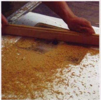
Since this was a pretty elegant project, I decided to tile the top with 12" × 12" (305mm × 305mm) limestone. That meant installing a 1<sup>3</sup>/<sub>4</sub>"-wide (44mm) trim strip for the front edge, because the tiles are <sup>1</sup>/<sub>4</sub>" (6mm) thick. If you're doing a standard wooden top, make the trim strip 1<sup>1</sup>/<sub>2</sub>" (44mm) wide. I routed the top and bottom edges of the strip on the router table.
