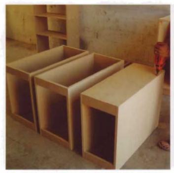
Since this project allows for some "quick and dirty" construction techniques, you can simply screw and glue the backs directly onto the cabinet boxes.
