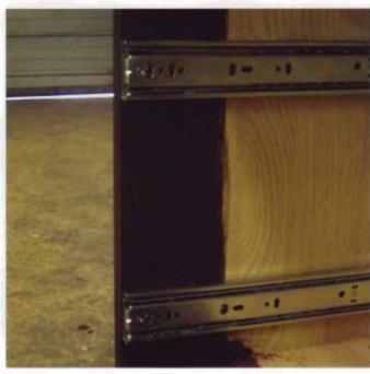
These aren't deep drawers, so full extension slides were a necessity. For details on drawer slide installation, see the Shared Master Bedroom Closet project. I constructed the drawers using rabbet-and-dado joinery- this is detailed in Beyond the Basic Box.
