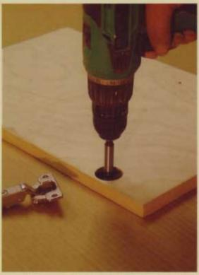
The hinges come in two parts: the hinge cup and the mounting plate. Start by drilling a hole in the door to hold the hinge cup. You'll need a 35mm or 13/e" Forstner bit. To locate the center of the hole for the hinge cup, make a pencil mark 7/a" (22mm) from the edge of the door.
