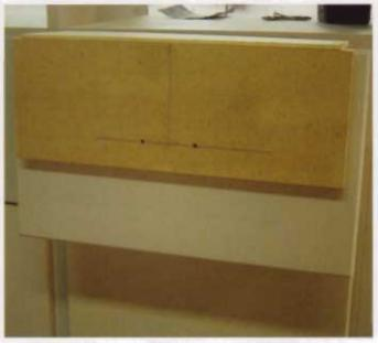
Because the holes for the chosen drawer pulls required unique spacing, I made my own alignment guide and I used it for all six drawers.
