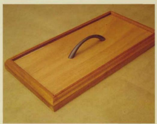
Miter joints allow the profile to wrap seamlessly around the panels.
