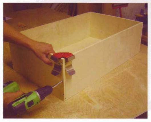
I kept it simple and glued and nailed the drawers together. Then I varnished them. For details on the drawer installation, see Installing Drawers with Accuride-style slides on page 50.
