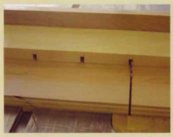
Using a miter gauge or a table-saw sled, I cut a series of dados across the piece of wood. The dadoes should be spaced equidistant from one another and should be as wide as the finished dividers will be [about 1/4" (6mm) wide].
