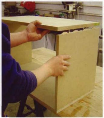
After a test-fit to make sure the slots are properly aligned, I glued up the assemblies and applied even clamping pressure. The test-fit may seem like a waste of time, but it's not. If you discover a discrepancy in the fit, you'll save a lot of time, stress and mess if you catch it before there's glue all over the place.
