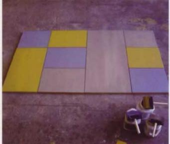
Making the doors and drawer fronts for this project couldn't be simpler. No edge-banding is required, and all you need to do is cut out MDF rectangles. To help develop the color scheme for this project, I laid out the doors and drawer fronts in their actual configuration. For me this was much easier and more direct than trying to work on paper.
