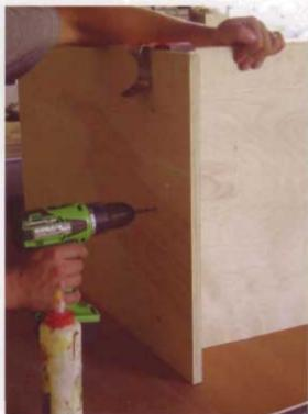
The dresser is essentially a four-sided box, with the back glued and nailed on. A separate top cap will finish it off and hide the exposed plywood edges which would otherwise be visible from above. Begin the dresser by cutting the sides and bottom to size. The bottom is glued and screwed into place; the sides overlap it. You'll notice that I inset the bottom 4<sup>1</sup>/<sub>2</sub>" (114mm) from the bottom edge of the sides. The toe kick will be installed in this space.
