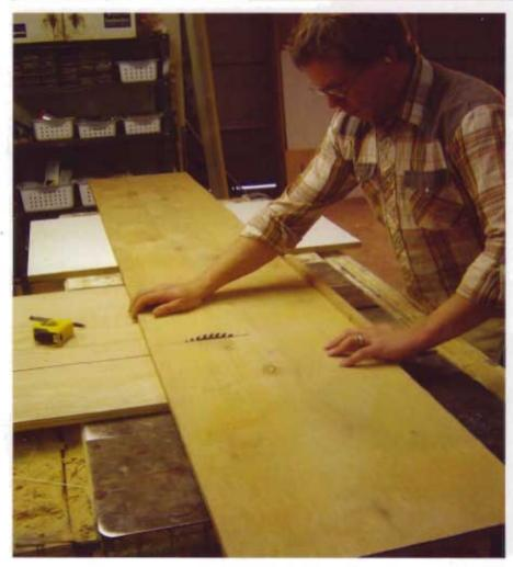
Begin by cutting out the parts for the dresser units. I used MDF because it takes paint well and requires no edge-banding, a detail which saves a considerable amount of time. You'll notice that some of the material I used is veneered with alder. I used it only because I got a good deal on it and was able to position those components in such a way that they wouldn't be visible after installation. It's also a good idea to cut out the three end panels at this time, since you're set up for it.
