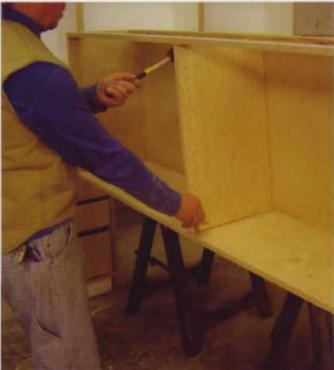
Nail the partition in cabinet G through the top, bottom and back. If it is too snug, use a rubber mallet to ease it into place.
