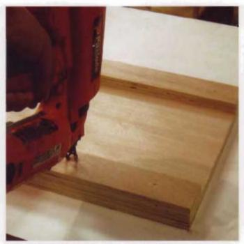
This countertop begins with a 48" × 12" (1219mm × 305mm) blank. I built up the edges with <sup>3</sup>/4"-thick (19mm) strips of plywood to give it a more substantial look.
