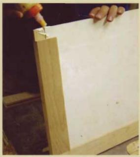
After test-fitting the parts, you can glue up the door.
