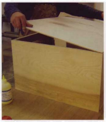
These cabinets can have the backs screwed directly on to the cabinet cases.
