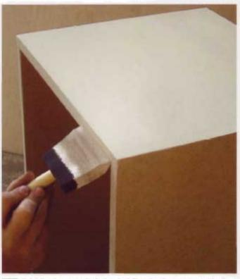
Paint the dresser units before installing the drawers to avoid getting paint on the drawers and sliders. The only parts that need paint are the tops and the front edges, as the drawers will hide the insides and the end panels will conceal the outsides.
