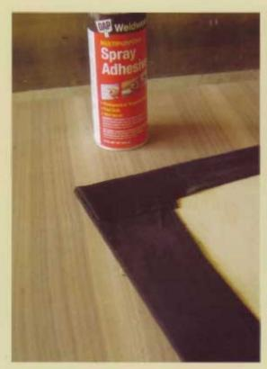
This false bottom is then dropped into the drawernote that you must size it 1/a" (3mm) smaller than the drawer's interior.
