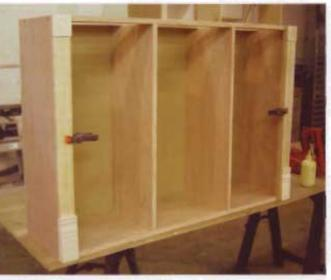
Rip and crosscut the parts for the base cabinet, then assemble it with screws. The screw heads won't show, since end panels will cover the sides of the cabinet. We dressed up the cabinets with some trim from a local home center. The trim consists of a length of fluted molding, a rosette and a plinth. The parts are glued and nailed to the cabinet, and the nail holes are later filled with a stainable putty. Screw the two vertical partitions from the top, bottom and back.
