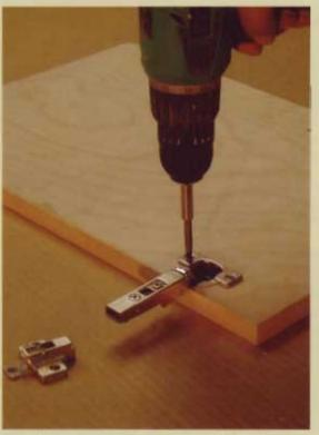
Be sure to place the marks far enough from the top and bottom of the door so that the hinges will close without hitting the top and bottom of the cabinet itself—3" (76mm) should do it. For doors longer than 36" (914mm), I recommend three or more hinges. You can secure the hinge cup with two 5/a" (16mm) self-tapping screws.
