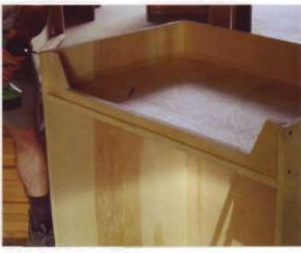
The toe kick is screwed and glued into place.
