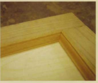
To add another interesting detail, you can make a small molding on your router table and apply it to the edge of the panel where it meets the stiles and rails.
