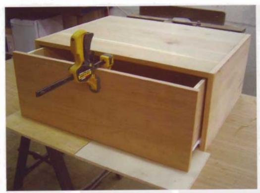
For the single drawer box, place a 1/2" (13mm) shim beneath the drawer front to set it at the proper height.
