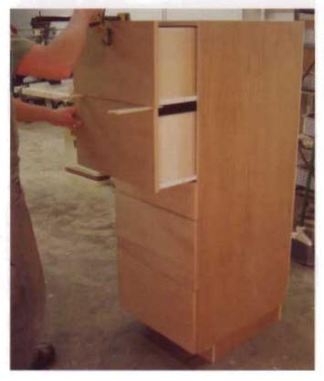
The cabinet top won't allow enough room to get a clamp in place for the top drawer front, so you'll have to pull it out along with the drawer below it. Work carefully and you shouldn't have a problem keeping the parts aligned.
