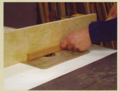
For most applications, I use moldings that measure around 1"  $\times$   $^{1}/_{2}$ " (25mm  $\times$  13mm), but you may want to experiment with different sizes and see what looks best. I use a sacrificial fence clamped to my router table's fence so that the bit is only partially exposed. This allows me to expose only as much of the bit as I need. I suggest cutting most profiles in several passes. It's safer and usually provides a neater, crisper profile.
