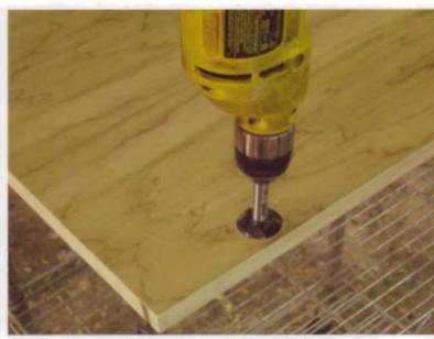
The doors are made from <sup>3</sup>/<sub>4</sub>" (19mm) plywood that has been edge-banded on all four sides. The holes for the European-style hinges are located 4" (102mm) from the top/bottom edge of the doors, and <sup>15</sup>/<sub>16</sub>" (24mm) from the side.
