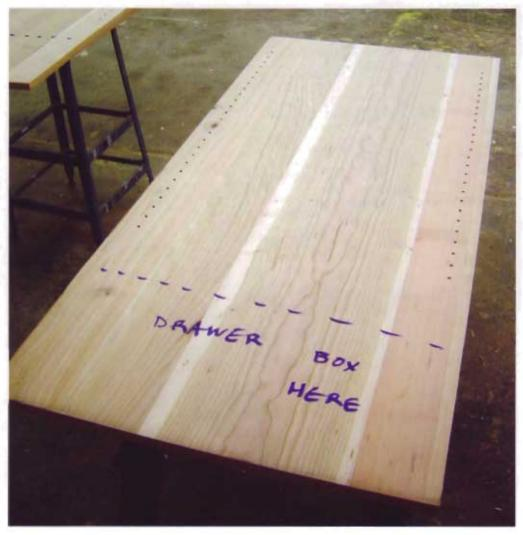
When drilling the holes for the shelf pegs, lay out the end panels in matched pairs. (I suggest labeling the back edges of the panels with a marker.) This is easy to do, and failing to do so can wreak havoc later on.
