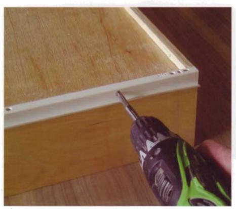
As long as you've positioned the cabinet side runners correctly, the drawers should be a cinch to install. With the drawer placed upside down on a workbench, the drawer rails can be placed on the bottom of the drawer and screwed on. The front edge of the rail should be flush with the front edge of the drawer.
