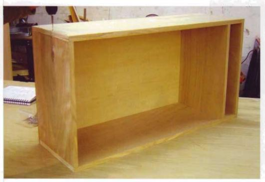
The upper cabinets come together with butt joints held together with glue and screws. The backs are glued and nailed on.
