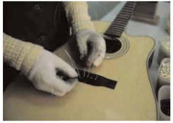
The guitar is tuned to 440 pitch, and then the necks truss rod is set and the guitar is played by the inspector to verify there is no fret buzz or other problems. If there is, electronics such as an EQ or Piezo it is tested now to check that there is even string response for all six strings.
