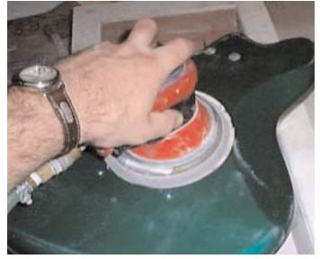
Wet sand the body in a back and forth motion with #1000 and #1500 to get the circle scratches out. The next step is I hand rub certain areas with a 3M Buffing Compound, but a car compound also works well. I do this to areas that are hard to get the buffer in on like some cutaway's or edges.
