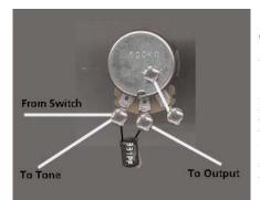
They also added a 331PF capacitor across the volume pot. This is so that the highs don't roll off when the volume is lowered.
