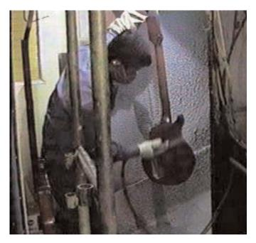
Certain colors in the factory require different spraying techniques, on many colors the bodies are first painted a base coat and when a second or third color is applied. The final color is made. Usually, to brighten up a color they would use a white base coat and on some darker colors a black base coat may be used.
