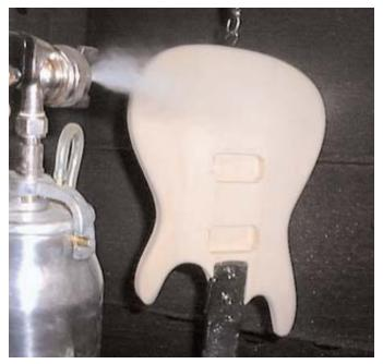
lacquer finish on a body it is sprayed at around 28PSI (Pounds per square inch) over 80% of the paint evaporates into the air. This is why it is almost illegal to spray in many places in the United States. All the finish that evaporates goes into the air and causes pollution.
