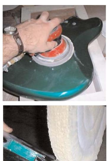
I use the buffing wheels because I have them, but you can get the same shine using a buffing compound that would be used on a car and just rubbing the scratches out. In the states I use a 3m compound and then I use a car polish called Macquires to bring the body to a high gloss.
