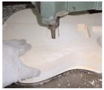
Once the basic body is shaped we need to find the center of the guitar. If the neck pocket is routed use this for the most accuracy. The reason for this is that the bodies center may be slightly different from the necks center. Put the neck on the guitar and run a straight edge down either side of the neck and draw a line. After both sides have this line, find the center of the body with these lines.
