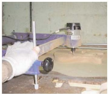
Once everything is lined up and depending on the wood I set the depth of the router bit higher then the actual final cuts. (The depth I go on each pass depends on the wood. harder wood not so deep passes but a softer wood like spruce you can go fairly deep. This is actually gutting the wood. The pin is easily adjustable. Once it is set I go back and forth until the basic arch is carved.
