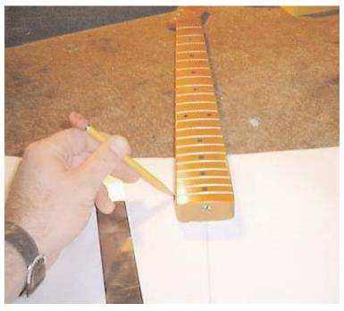
What you need is the nut, twelfth fret and the last fret. It really helps to have a slotted fretboard or a complete neck to lay down, this is the most accurate way,. If not you will need to figure it out mathematically.
