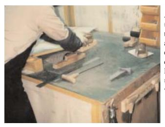
After the frets are even then use the long block with the #500 to sand out the #280 scratches on the frets. Next take the round block and hold #500 paper on it and sand back and forth the length of the fretboard to remove any scratches from the frets, this will also round the tops and sides. Be careful not to sand the tops too round you don't want to loose the top crown. Repeat this process with the #800/#1000 and #1500 paper and final polish the tops of the frets with the #0000 steel wool.
