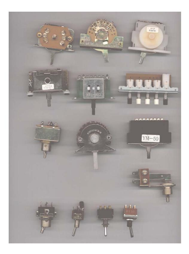
A 5-way switch works as follows. In the one, three and five position's only one pickup is one. In the two and four positions it combines both the bridge and middle or the middle and neck. When the middle pickup magnets and wires are reversed, the two pickups will work as a humbucker in Parallel Wiring.
