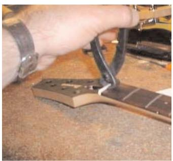
Then use a hammer and a short metal piece to pop the nut out. Lay the flat edge of the metal bar against the nut and give it a sharp tap with the hammer. The nut should come loose then lift the nut out of the slot. For Fender® style nuts that are bone, or graphite these can be tricky. The best way I have found to remove these nuts is to use a pair of end nippers that remove the frets to wiggle the nut until it becomes loose and then remove it.
