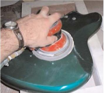
I use a palm sander with #800 dry on it and sand the area flat until all the shinny spots are gone, and the seam lines disappears. Then I use #1000 and #1500 wet, then buff the area. If you don't have a palm sander just use the #800 wet with a flat block to sand out the seams then follow the #1000 and #1500 paper and buff.
