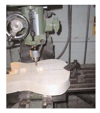
Continue milling each line to the proper depth.
