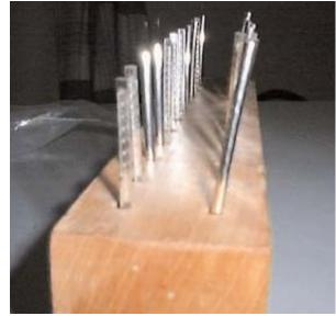
Now to install the frets I first use a rubber mallet to set the frets in the slots and then a drill press with the proper radius arbor to set the frets in. I made my own wooden presses a while back on my pin router but since I purchased the brass ones from Stew Mac, I have been using them.
