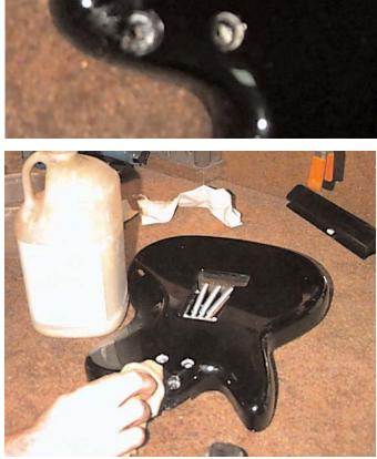
On more complicated cracks you will need to repair the crack as well as refinish the area of the crack. For this type of repair remove all the parts off the body. Close the crack the same way as before using super glue until the cracks are completely closed up. Next you will need to break the finish area that will be repainted because paint does not stick to a buffed finish. I recommend using Scotch Bright ® pads to rough up the finish in the area that will be repainted.
