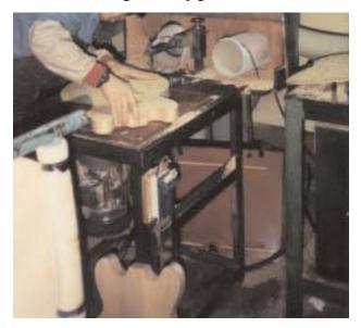
The back of the necks are shaped on a shaper table with a jig and the final shaping is done manually on a belt sander.
