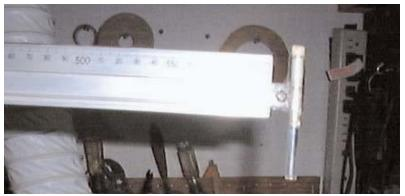
This was designed by Fritz Katoh and is used for checking the neck set angle on acoustic guitars. This is basically a straight edge with a handmade gauge on the end. When laid across the frets the guage tells what the neck angle is set at. Many people use the same type of jig but with a fixed shim of say 14mm and use this when they are actually setting the neck before gluing.
