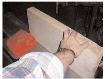
Next open the wood flipping up the two sides that will be joined. Glue is applied to both sides and then use a rubber, nylon or wooden squeegee to smooth out the glue.
