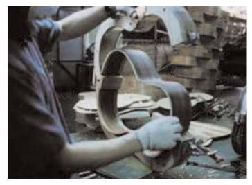
Before gluing the top on they cut the ends of the bracing. This could be done before they installed the braces but because it is much easier to keep accurate the length of the braces so they are flush with the sides of the body; this is important for the sound transfer to the top.
