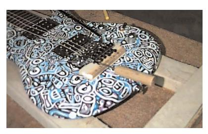
Now that the strings are off the guitar clean it up. Use the polish and a cloth for all the painted surfaces. It's good to clean around the pickups, bridge and headstock while you have the strings off.
