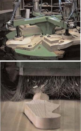
After the CNC rough shapes the necks, they still need allot of handwork. First, they are moved to an area where the headstock and heel areas are shaped and the truss rod slots are cut.
