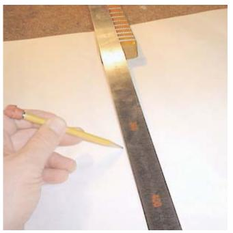
divide it by /2 then measure from the twelfth fret to the body, we will compensate for intonation later. (A 25.5-inch scale is 12.75" from the twelfth fret to the body scale location.)
