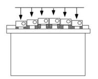
If you are adjusting the individual string saddles you will need to pay attention to the fretboard radius. This means the middle strings will need to be set higher. A good way to do this is to set the high and low strings to where you like them. Using a ruler measure the distance between the top of the fret and the bottom of the string on both the high and low strings at the 12 fret.
