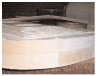
Once the step routing is finished you will see the basic shape of the arched top. From this point I use a round chisel to carve off the sharp edges.
