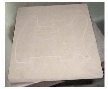
Make sure you raise the old pickguard above the new piece other wise there is no room for the bearing. Just drill out the other holes for the pots and if you have a 5way switch drill some small pilot holes where the lever will be and clean it up with a small file. I use the mill to do this for a one of a kind. To do the pickguard edge bevel (it should be at 45 degrees). We use to do the edge on the belt sander by holding the pickguard on a 45-degree angle.
