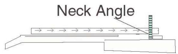
Lower the router in the wood just enough so that the bearing guide rides on the inside of the template and rout away following the template. After the first rout lower the bit and do the second depth rout. Continue until you have the proper depth, I used 18.5mm for the neck pocket on this guitar.
