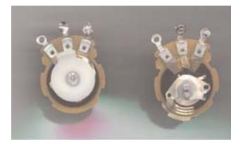
The volume of a pickup is controlled by the potentiometer. A potentiometer (pot) is a variable resistor that allows you to vary signal flowing through it.
