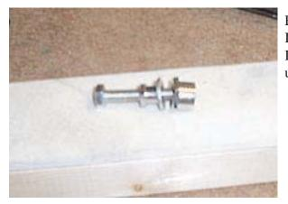
First, if there are inserts in the wood remove them. To do this I use a stud extractor that is similar to a wheel extractor. First, I use a threaded bolt that fits the studs, a nut and a washer. I use a bass machine head grommet as a spacer.
