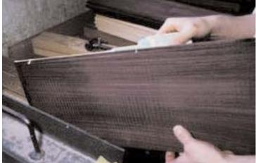
clamps are closed on the wood, weights are laid on the joint to remove any flexing. The glue sets in about 30 minutes and takes 24 hours too completely dry before any production can begin.
