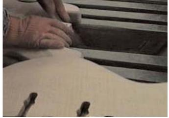
finish. The top and backs are sanded on a stroke sander with between 320 and 400, and the sides are sanded on the end drum of a belt sander.
