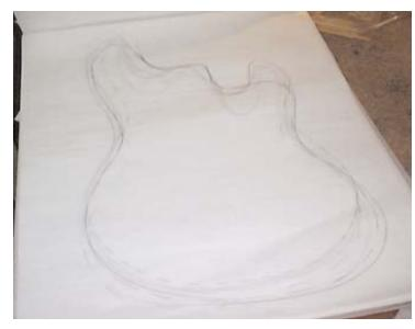
Ok your mind is fresh, look at the drawing and first figure out what does not make sense maybe the tremolo runs into the back of the guitar or the control's do not have room or the guitar does not look balanced.
