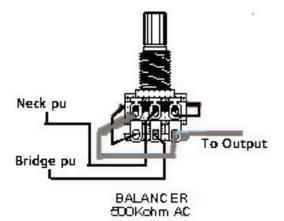
Many basses use balance pots that are stacked with two pots put together. By reversing one of the pots it will blend the two pickups together. Balance pots use different tapers for each pot this assures a smooth transition between pickups. The standard tapers are A and C.
