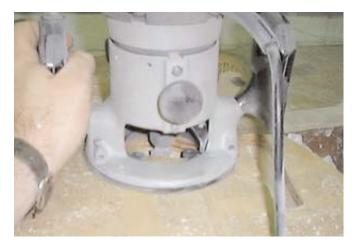
After the neck pocket is routed lay the neck in the neck pocket it should fit snug. Check the centerline to confirm it is lined up with the rest of the body routs. It's good to lay a long ruler down both sides of the neck and draw a line on the body. Hold the ruler against the sides of the neck from around the 15th fret tightly against the neck and draw the line make sure you hold both sides the same.
