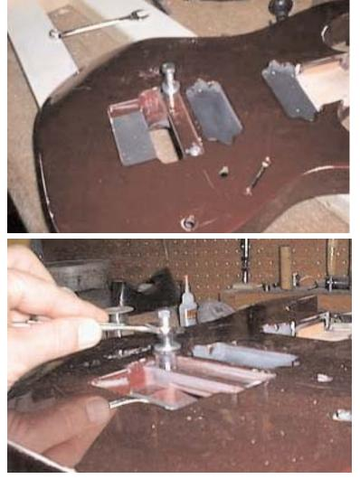
Place the grommet over the stud, insert the bolt through the insert with the washer and nut in place, tighten the nut into the grommet and the stud insert will be pulled out of the wood. (Stew Mac sells one of these but they are easy to make)
