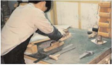
After the bodies are finished and the clear is dry they are sent to the final sanding section where they are first sanded with a stroke sander to level out the finish, and then they are wet sanded to #1000 in a sanding line. The bodies are buffed, and the final control cavity, tremolo routs and pickup routs are done they do this after the wet sanding so the wood does not swell.
