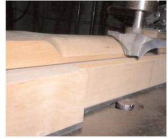
er so that when I shape it on the pin router the neck will be shaped 2mm thinner at the nut area. If I did not have the pin router, I would rough shape the necks back radius on the belt sander.
