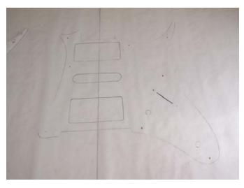
When the pickguard looks good lay another piece of tracing paper over the drawing and make a trace of it to make the pickguard. If you will make more than one pickguard make a template, Other wise you can just make it by hand. Band saw the basic shape and use a hand router and a really small bit 1/8" to copy the routs.
