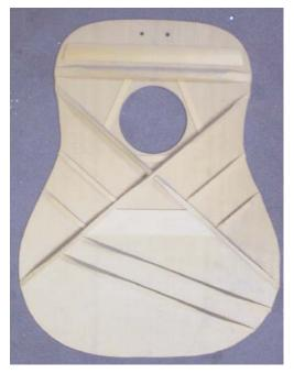
mon nowadays then they used to be. In the old days and still at Martin all scalloping is done by hand. Scalloping is when you shave the braces thinner to give the top better vibration with less stiffness caused by the braces. Asian factories have designed a machine that scallops all the braces simultaneously that they are cut to size and shape. Almost all factories now use some type of scalloped bracing.
