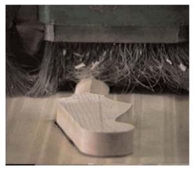
The digitizer is removed and the standard ball mill bit is put on the router and the program makes a perfect copy of every detail of the first neck. If there are any imperfections in the sample neck the computer will copy them but actually smooth them out. For example if there's a big dent in the sample neck the digitizer will copy it but because it can't make a puncture in the wood like a dent it will smooth out that area.
