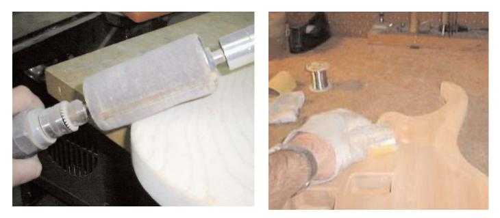
You're nearly done. Use a round block and #120 sand paper to clean up the rasp marks and hand shape the edge to match the rest of the guitar edge round over. You can try to use the hand router with the round over bit, but it's really hard to hold the router. Sand out the body with #120, #180, and #220 and get ready for Paint and Finish
