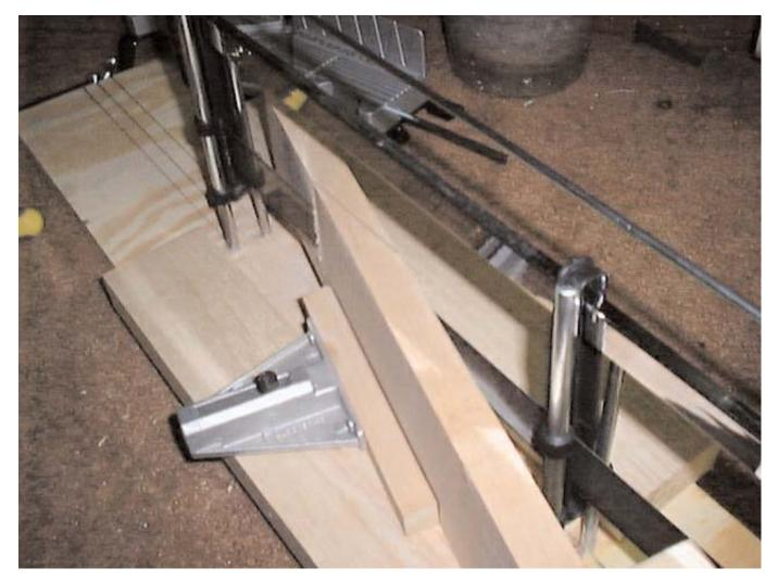
Cut the scarf joint and if you have a jointer plane the wood flat if not use the belt sander to flatten the surface. Once the wood is ready for gluing, take a small amount of water and open the cells in the area that will be joined they were crushed when they were sawed so the glue could easily come loose. Just dampen the area and wait for it to dry before gluing it up.
