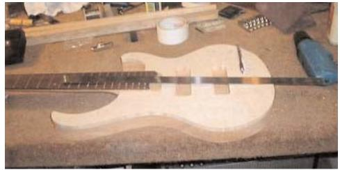
I pretty much stick with the standards on this if the neck is bolt on neck and uses a tremolo I will use a 25.5" scale and if the neck is a set in and uses a non tremolo bridge I always use the 24.75" scale. For basses I use standard 34" scales for almost all of them except for five and six strings that I would maybe use 35" so that the low B string does not flop around.
