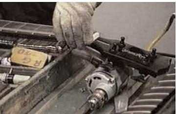
After the guitars are assembled they sit for a day, so that the finish can settle. Then they are sent to the setup area where they are setup to the factories or customers specifications.
