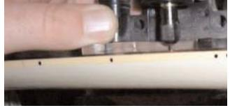
I prefer to radius the frets to size. After the frets are radiused I cut each one to the width of the fretboard you can use a caliper for this if you like but I just hold the fret on the board and cut it to size. If there is binding then I nip the fret ends back as above and gently file the hang over edge flat. The reason for this is that sometimes the nippers don't remove some of the tang.
