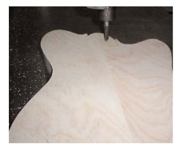
For example, if the binding is 2mm I use an 8mm pin with a 12mm bit this will rout a perfect 2mm channel for binding.
