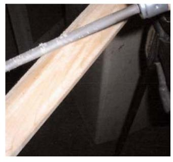
Now comes the fun part final shaping. First, rough out the fretboard radius so that when you hold the neck in you hand it feels natural then use round files to shape the actual necks back profile to the desired feel. Keep checking the shape with your hand and feel each area of the neck to verify it is what you want.
