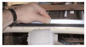
spots that may cause trouble and set the neck as straight as possible by eye. Then take a long straight ruler and lay it against the top of the frets and adjust the rod until all the frets are against the ruler. On a detachable neck lay it flat on a table if it has a tilt back headstock keep the headstock over the edge of the table so that the fretboard is sitting flat.
