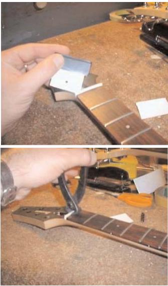
To install a new nut measure the nut slot and nut material. Cut and shape the nut material to the exact size of the nut slot before gluing it in. I use super glue to mount the nut, but you can use white glue if you want.
