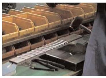
The frets are first hammered in manually, just to set them and then the frets are pressed in using an arbor press.
