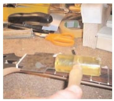
The next procedure is to remove the frets, be careful not to chip the wood around the fret tangs. The way I do this is to use a solder iron and rosin core solder used for wiring the electronics. I use the solder iron and actually melt the soldier across the top of the fret.
