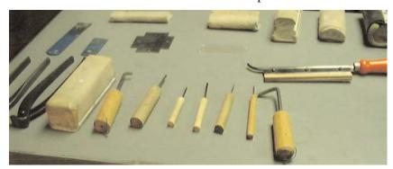
er to use than a standard angled wrenchs, second they are easier to find on a crowded desk and best of all then can be setup on a work bench for easy access. To do this I just use a grinder to make the wrenches straight and drill into the dowel the correct size and super glue the wrench in. The upper left tools are hand made scrappers that I make from old hack saw blades. Next is my custom nut cutting template that
