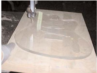
but up around the neck pocket these cuts are harder to make. Nowadays I use 1/4" band saw blade because it can get into the area well, make turns and get back out. For the deep cutaways at the neck area make straight cuts in from the outside to different points in the cutaways before making the main cut, so that the blade does not get stuck in the middle and stop.
