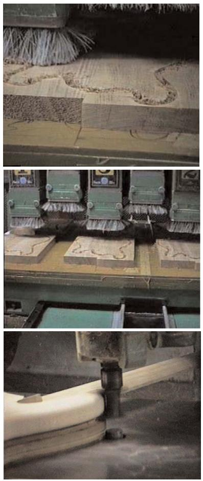
After the bodies are rough, cut on the CNC they are moved to the sanding section where the comfort cut is added and any imperfection or tear out is removed.
