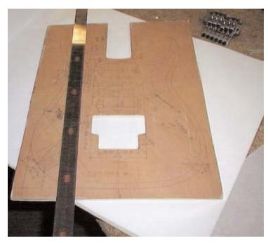
First, you need to do something, maybe install a tremolo, add a humbucker to a Strat or something that needs routing. Most tremolo systems that you purchase come with a drawing of a template that you can make. Even the sink I installed in my bathroom had a template drawing on the box for the hole size to cut in the counter top.
