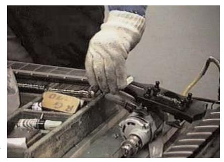
tion, string retainer, intonation, neck set, top arch, mounting ring holes. For shaping necks on the pin router I have a jig that shapes as well as has the truss rod channel template in it.
