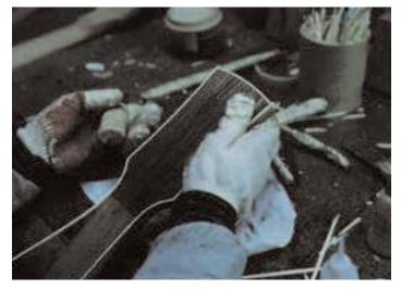
After the body is dry and removed from the side presses the binding channel is cut around the body using a modified router table; The body is then bound.
