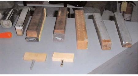
This is a collection of tools I made for set up. Just Allen wrenches set in dowel rods. First, they are much easi-
