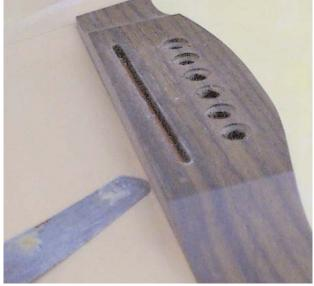
made a simple bridge template that I double stick tape on the top, and I just use a standard hand router and slowly rout down the bridge until it is just a micro thin piece over the top and the last piece just peels off leaving the top perfect for the new bridge.
