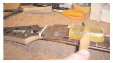
On a blank style nut I use a small metal bar to pop off the nut. With a Fender® style nut I try to wiggle it out with a pair of dull fret nippers, be careful you can easily take the wood with it. I read somewhere to saw the nut in half-long ways down the center. I tried this and it worked however, I always like to keep the original nut intact for at least marking the nut slots for the new nut.
