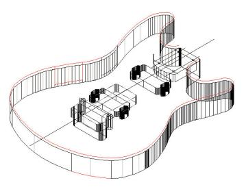
Once the drawing is finished, we use it to either make the templates or to make the actual CNC program that will cut the bodies. The drawing will always be the main reference for all production models.
