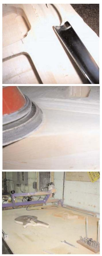
The left side is the copy area, and this is where the template goes. There are different size pins available that match the size and radius of the router bits.
