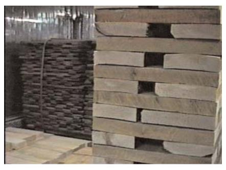
The woods are first sorted, cut to size, planed to the correct thickness and placed in a drying room to sit for a few days until the moisture content is stable.
