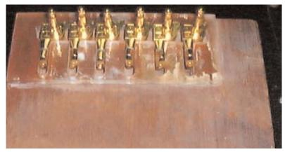
I made this jig for machine heads, because when I replaced necks sometimes I had a hard time getting the tuners straight. This was a pain so I milled out a piece of wood to the exact location of the six tuners. I put the tuners in the jig and set the neck on it, put the nuts and washer's on the posts and tighten. This places all the tuners in a perfect line. Next I just drill the screw holes and add the screws.
