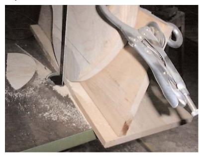
Trussrod channels can be either milled or routed I have a few ways of doing it but for a hand router. I made truss rod channel jig for routing the channel slot.
