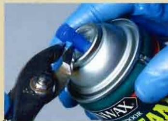
**ADJUSTING THE ORIENTATION.** A pair of pliers may be used to turn the nozzle to get a vertical spray pattern.
