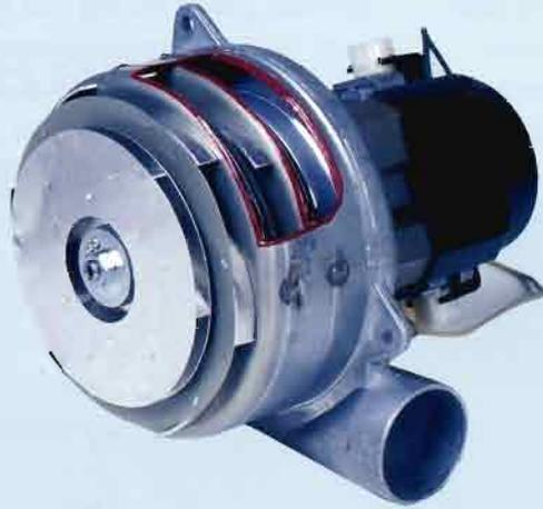
**TURBINE-POWERED HVLP SPRAYERS** are driven by high-speed compression fans that rotate at about 20,000 rpm. Each fan is called a "stage." In general, the more stages, the more varieties and thicknesses of finish the unit can spray.
