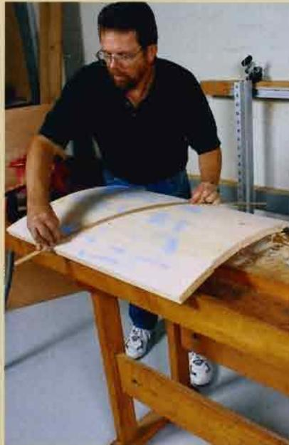
**CHALKING HIGH SPOTS.** A thin batten is coated with chalk, then bent across the surface to find high spots in the curve. The chalk marks are sanded away with a sanding block.
