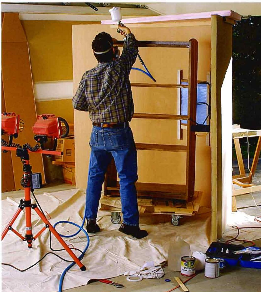
**GARAGE SPRAY BOOTH.** The spray booth fits into a garage-door opening, and a box fan draws some of the overspray into the filter and fumes into the open air.
