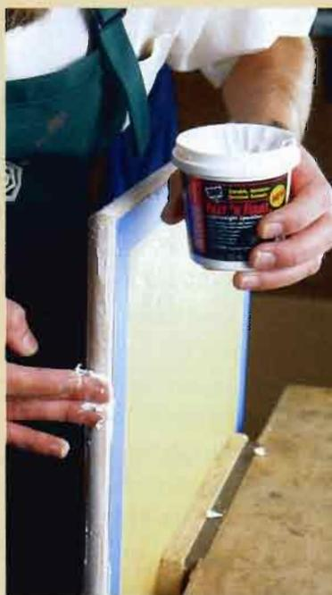
**SPACKLE FILLS VOIDS IN MEDIUM-DENSITY FIBERBOARD.** After masking off the veneered top of his table with paper and acrylic adhesive tape, the author rubs wallboard spackle onto the MDF edges. The spackle adheres well, dries quickly, and sands beautifully.
