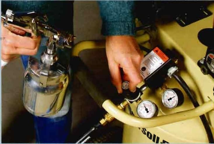
**SET THE AIR PRESSURE.** With the gun’s trigger depressed to allow only air to pass, set the outlet air pressure at the compressor, taking into account the hose-pressure drop (see the chart below).
