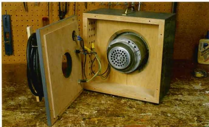
**MOUNTING ELECTRICALS.** Switch, cord, and circuit breaker are mounted in the back panel. Holes in the side of the back chamber are for motor-cooling air. A wooden cleat holds the wound cord.
