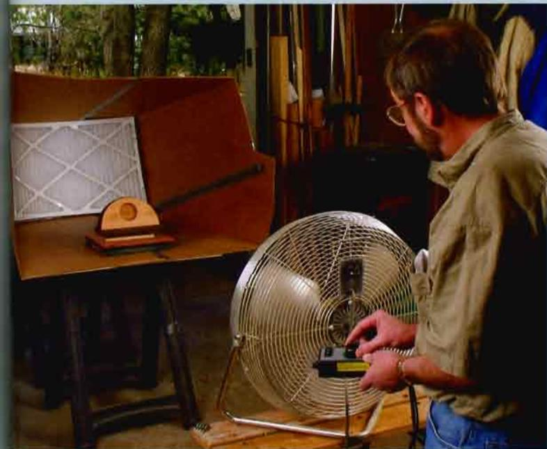
**A GENTLE BREEZE.** A router speed control slows the fan driving air through the spray booth. Without this reduction, the force of air would bounce the overspray and vapors back into the operator's face.
