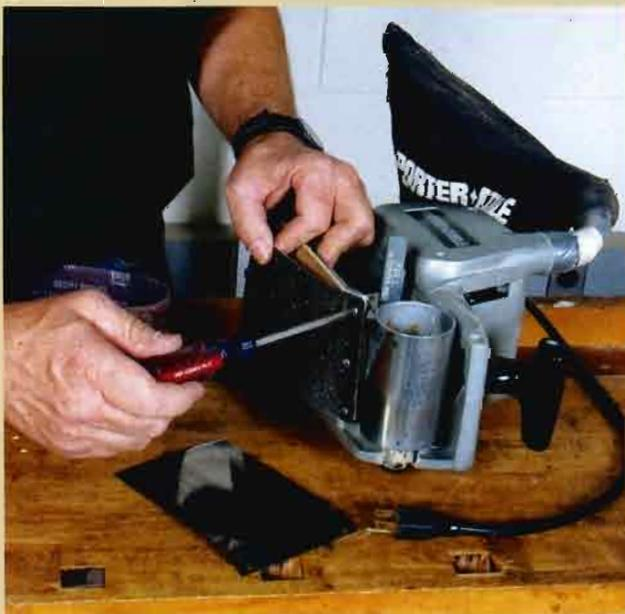
**AN UNEVEN SANDER WON'T FLATTEN ANYTHING.** The author replaces a belt sander's metal platen with graphite-coated canvas using the old platen as a pattern. A new, flat platen can make a big difference in a machine's performance.
