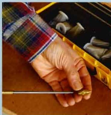
**CHOOSE THE RIGHT-SIZE NEEDLE/NOZZLE.** The higher the viscosity of the finish, the larger the needle/nozzle to achieve good atomization.
