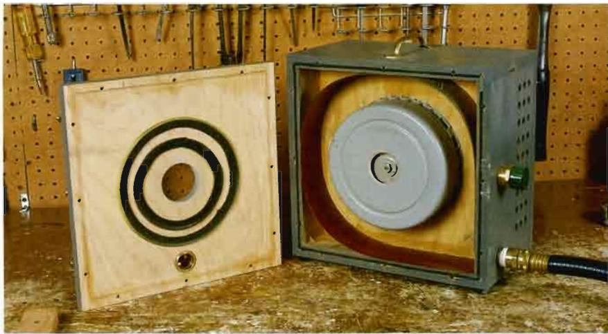
**IMPROVING SPRAYER OUTPUT.** Plastic laminate coiled in the outlet chamber acts as a fairing and increases output by lowering resistance. Weatherstripping and rubber tubing form gasket seals.
