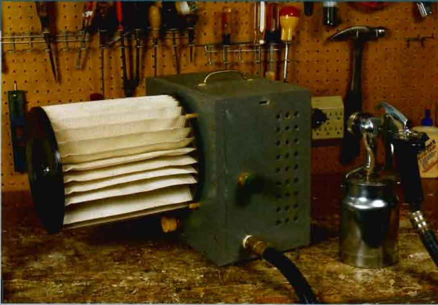
**HVLP IN A SMALL PACKAGE.** At 15 in. sq. and 18 lbs., the shop-built turbine-powered HVLP spray unit in the photo at left is a fraction of the size and weight of the standard medium-sized compressed air setup in the photo at far left.
