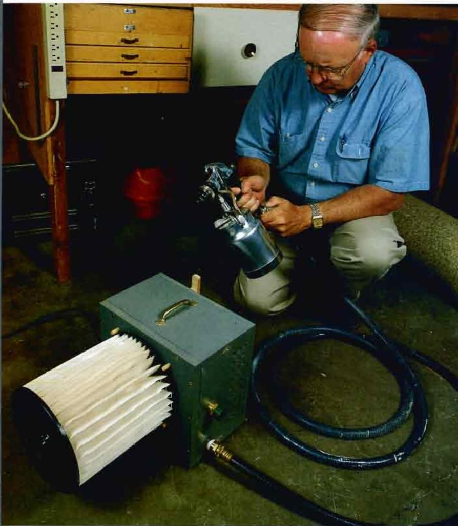
**SHOP-BUILT SPRAY UNIT.** A high-volume, low-pressure unit like this one that the author built is ideal for on-site work or in the shop.
