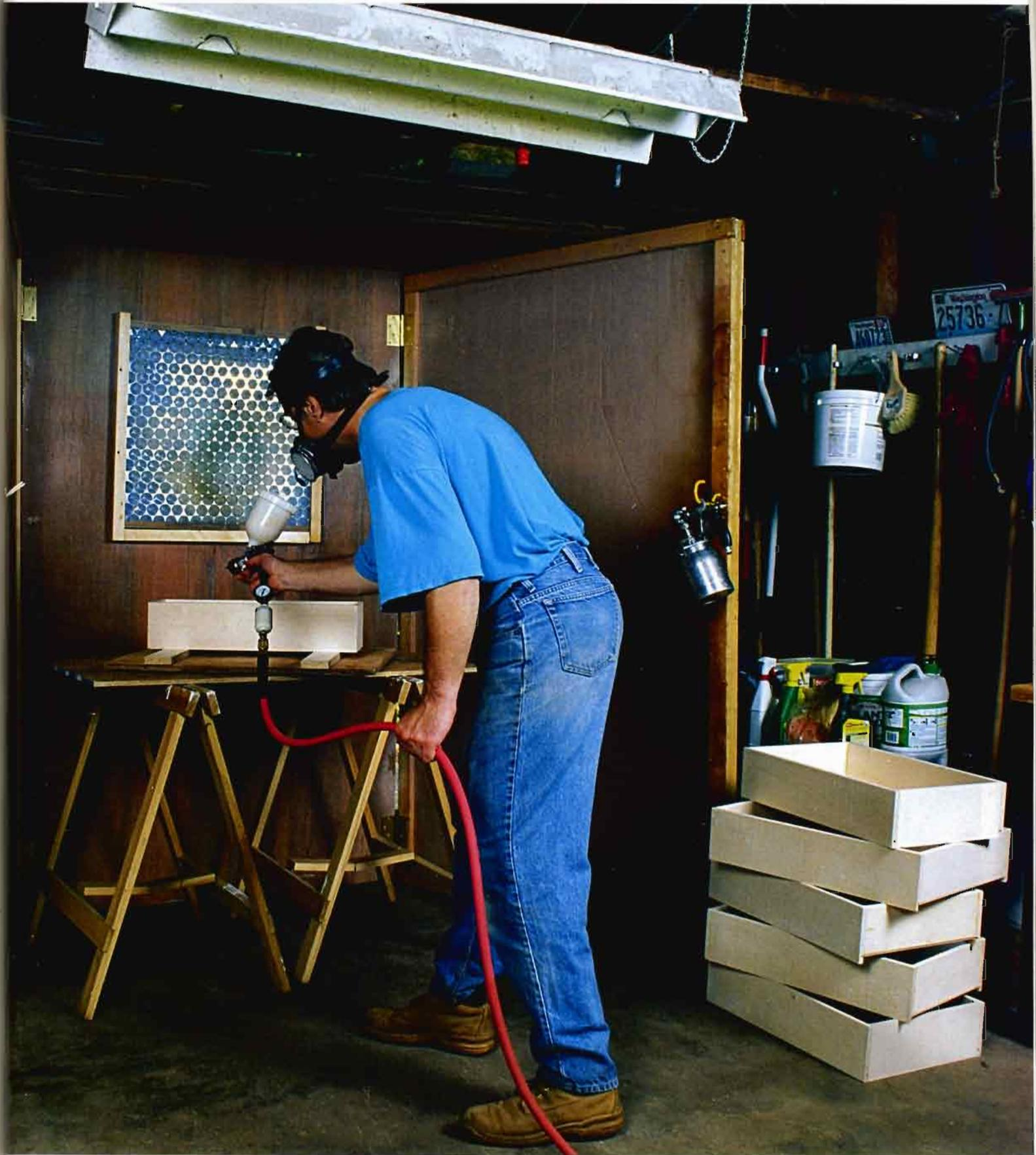
1,725 rpm, and it moves 2,000 cfm of air at 0 static pressure.) I recommend using at least a 16-in. fan and an explosion-proof motor, even with nonflammable water-based finishes. The fumes may not be flammable, but the fine dust that accumulates around the intake area and the discharge opening is a potential source of ignition. Check local electrical codes for making the proper electrical connections for the fan.
