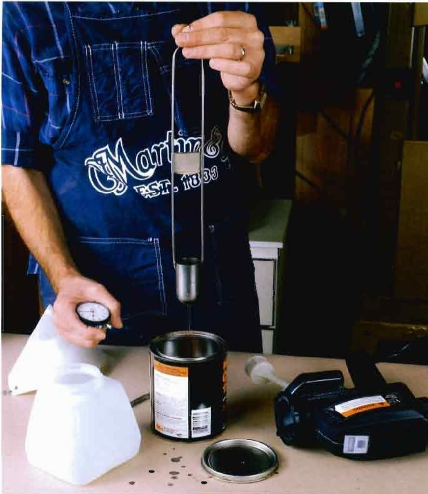
**CHECK THE FINISH WITH A VISCOSITY CUP.** A stopwatch and the recommended viscosity cup show whether thinner must be added. Once thinned, the finish is passed through a filter.
