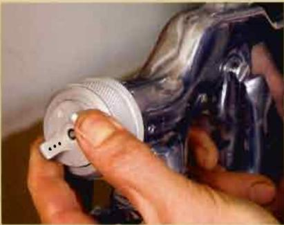
**TURBINE GUNS ARE ADJUSTED AT THE FRONT.** To adjust the pattern from circular to horizontal to vertical, just turn the air cap.
