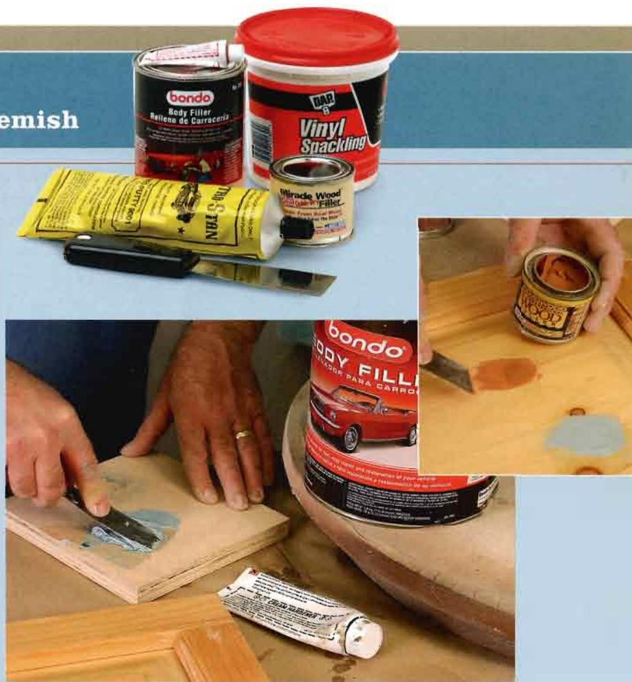
**A SMOOTH SURFACE.** Large holes are best filled with an auto-body filler that must be mixed with a hardener (above). Fast-drying wood filler is ideal for medium-size holes (center right).
