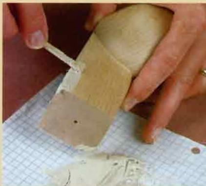
**TWO-PART AUTO-BODY FILLER WON'T SHRINK**, so it's great for leveling defects in wood. Using plastic-covered graph paper to measure the proper amount of filler and catalyst, Minick mixes the filler. After he packs the filler, he uses a knife to strike the repair flush with the surface, which will reduce sanding later. Areas of the leg that will be glued have been masked off. The filler cures quickly.
