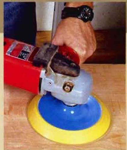
**ALWAYS HOLD IT STEADY AND FLAT.** Some newer orbital sanders are as aggressive as belt sanders. As with any sander, the pad should be held flat on the surface. Any time the pad is tilted, it digs a crater in the surface of the work. Back up a grit or two to remove them.
