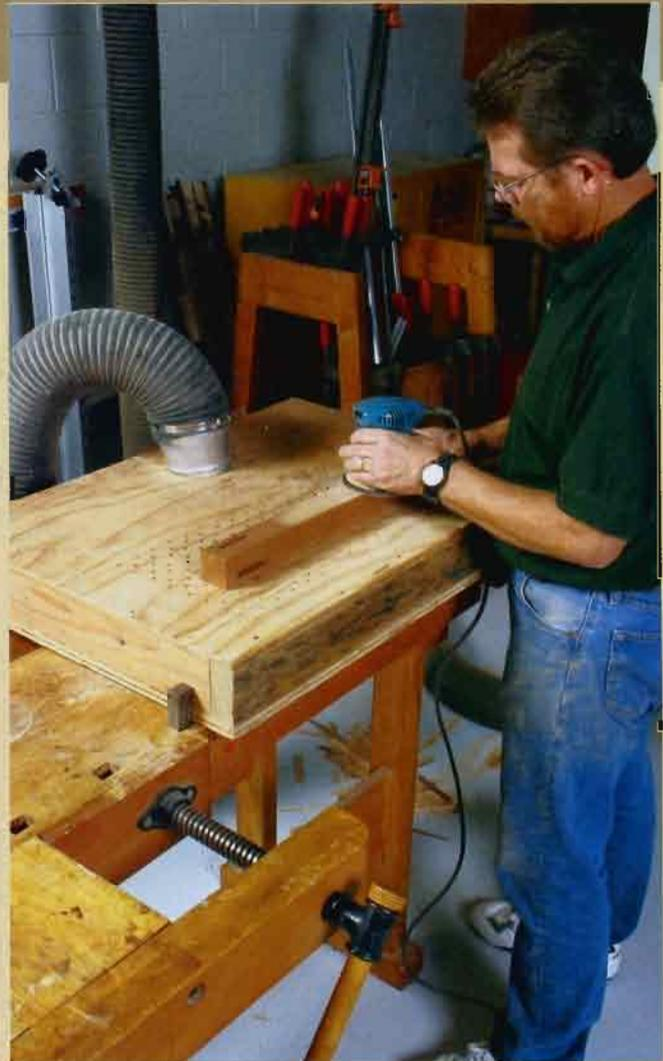
**A DOWNDRAFT TABLE KEEPS IT CLEAN.** The author's sanding table is just a box drilled with holes to suck the dust away. This simple box, made of plywood and 2x4s, hooks up to a dust-collection system or shop vacuum.
