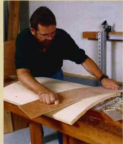
**PLIABLE SANDING BLOCK.** The author glues sandpaper to  $\frac{3}{4}$ -in. plywood, which bends and slides smoothly over the surface, keeping a curve in line.
