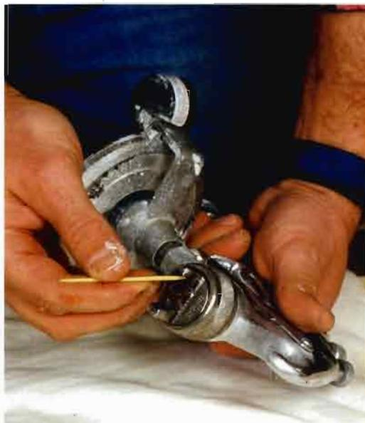
**CLEAR THE AIR PASSAGES.** Wood toothpicks won't damage the precisely machined air-cap orifices, which can get clogged with finish.
