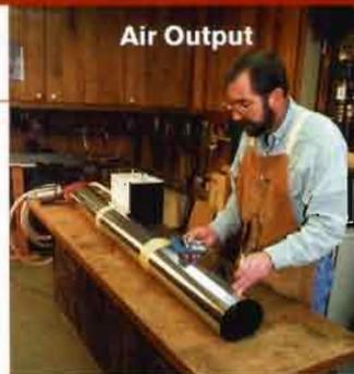
**MEASUREMENTS OF ACTUAL AIR OUTPUT, made with an anemometer, did not agree with those of most of the manufacturers.**
