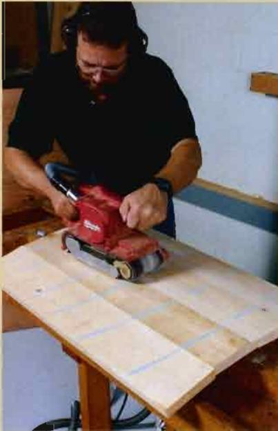
**ROUNDING THE GLUELINES.** Horizontal chalklines stripe the surface, and only the highest spots—the gluelines—are sanded in vertical stripes until the curve nears its final shape.
