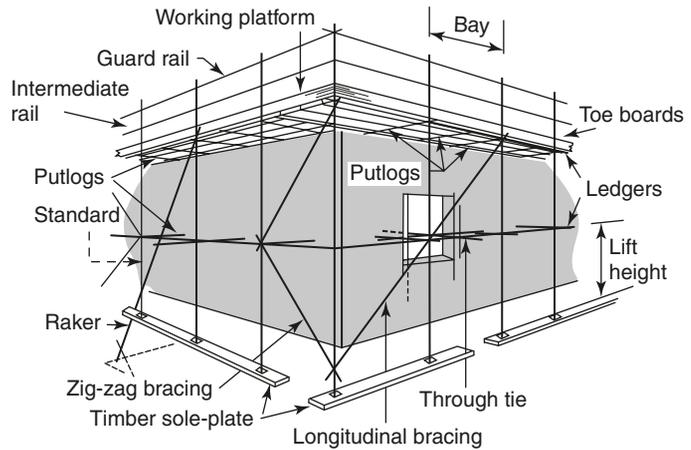
**Fig. 10.10** Putlog-scaffold arrangement
