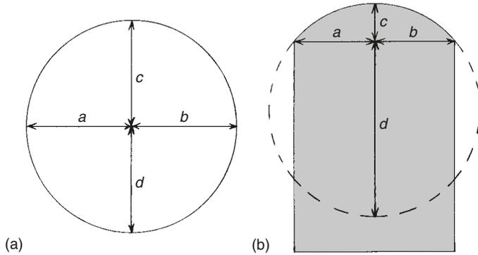
**Fig. 4.9** Calculating the radii for an arc
