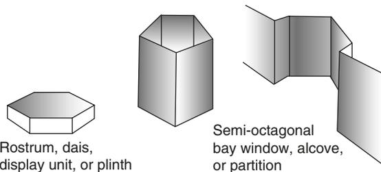
**Fig. 1.23** Regular and semi-regular polygons and examples of use
