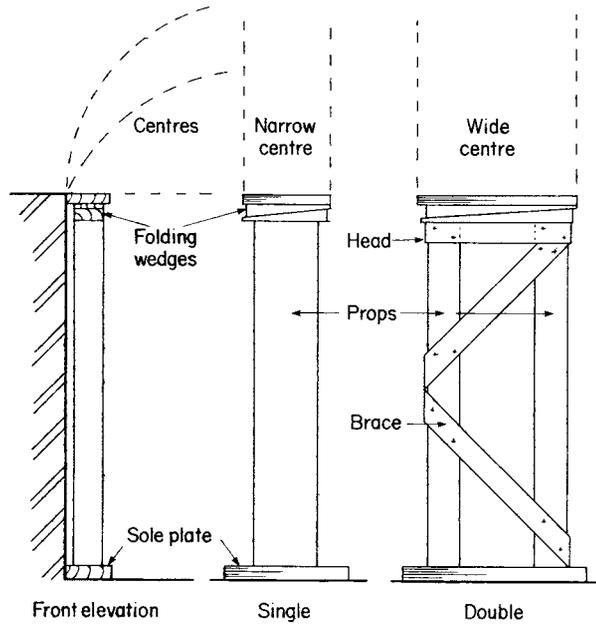
**Fig. 4.18** Centre placed on timber props and levelled in place
