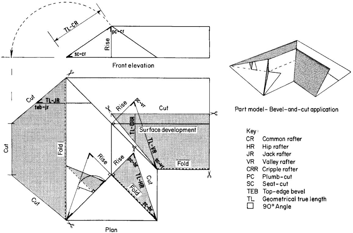
**Fig. 8.9** *Roof geometry*
