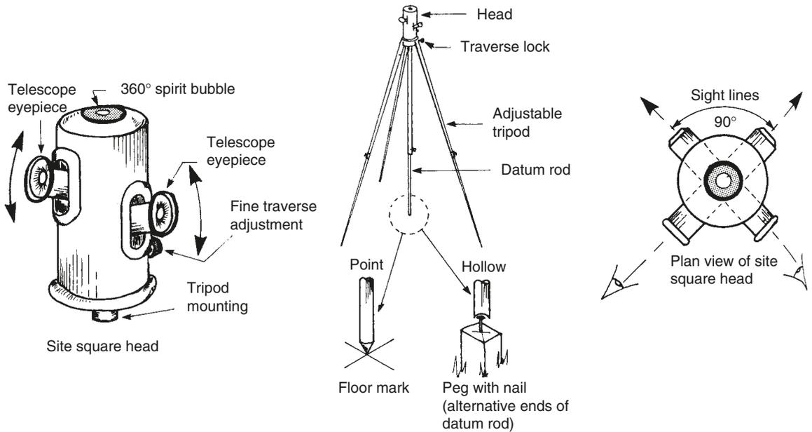
Note: Telescopes are set at right angles to one another – both move vertically
