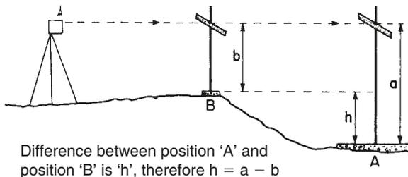
Fig. 1.41 Measuring different heights
