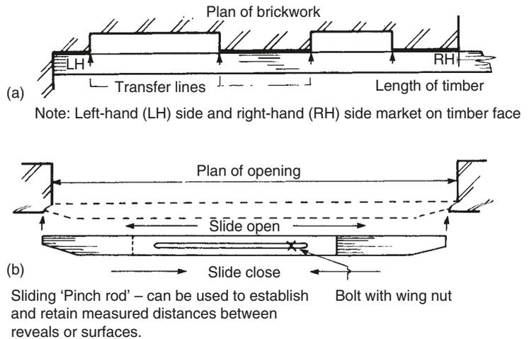
Fig. 1.7 Useful devices for transferring measurements
