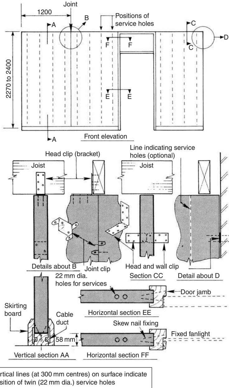
Fig. 9.13 Possible partition arrangement using the 'Karpfos' non-demountable system
