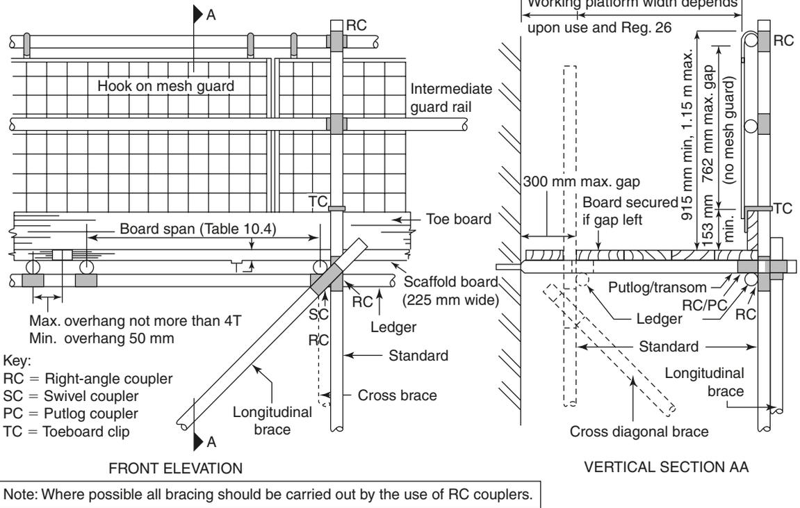
Fig. 10.16 Working platform for a tubular scaffold
