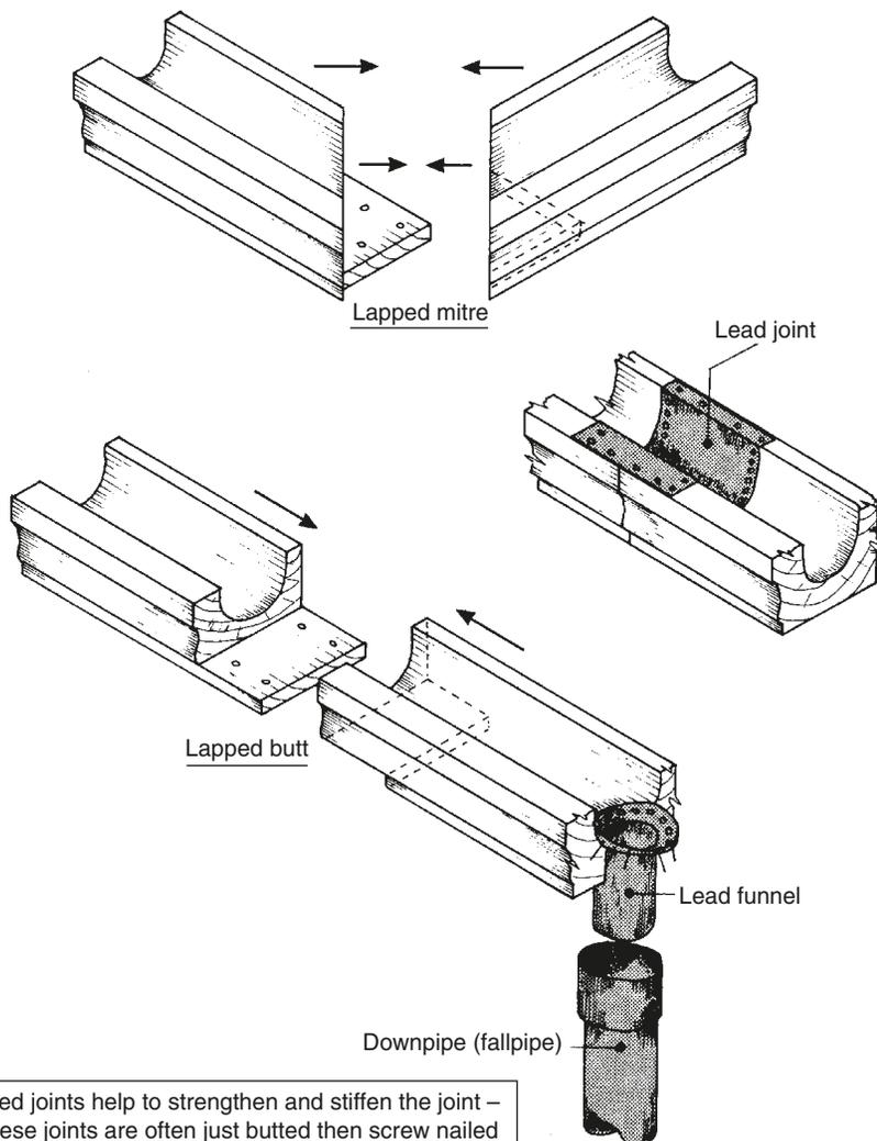
**Fig. 8.36** *Traditional wooden gutter joints and connections*
