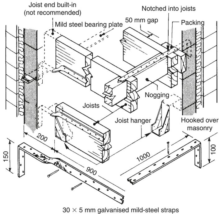
Note: Joists strapped to walls at intervals of not more than 2 m
