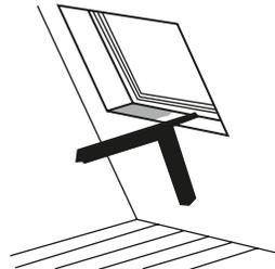
Using the extension arm to measure the angle of an inclined window cill or bracket
