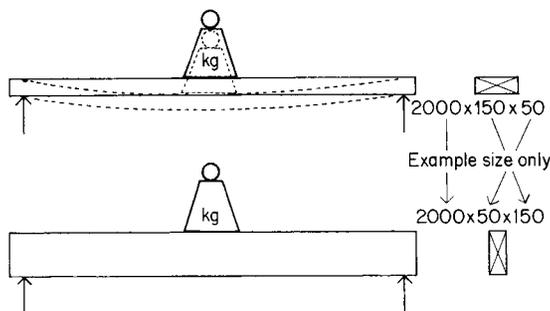
Note: the order of dimensioning drawings—length x width x depth
