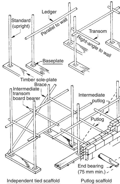
N.B. Couplers not shown (all load bearing couplers to be load bearing fittings)
