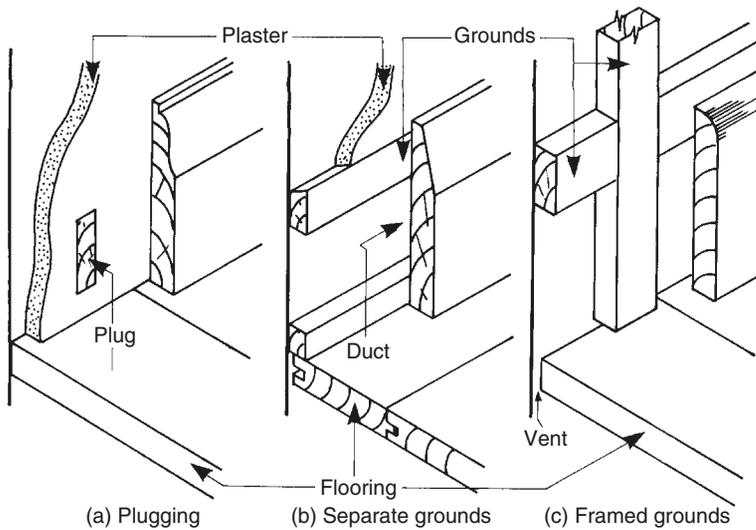
**Fig. 5.29** *Methods of fixing skirting boards to walls*
