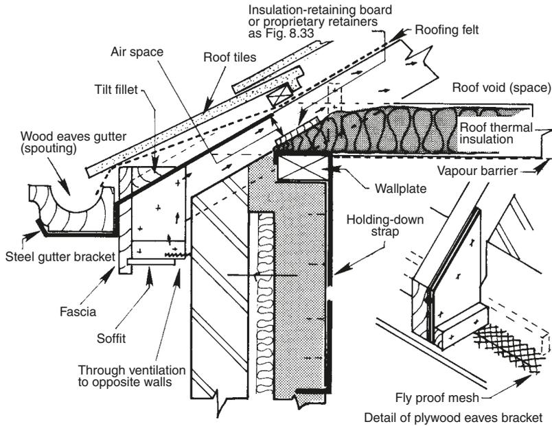
**Fig. 8.32** *Insulation and eaves detail (traditional roof construction)*
