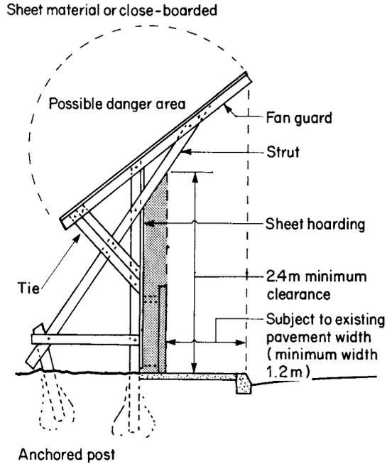
**Fig. 2.16** Fan hoarding: a diagrammatic representation
