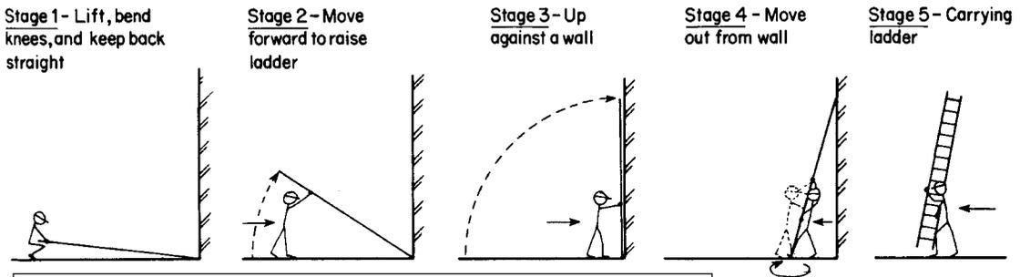
NOTE: Erecting and moving ladders over short distances—beware of overhead cables etc. Metal ladders must not be used in areas where electric cables are present
