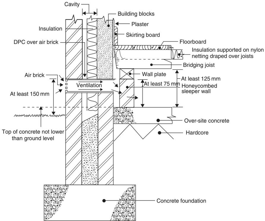
Note: Actual ventilation opening to each external wall at least 300 mm<sup>2</sup> for each metre run of wall
