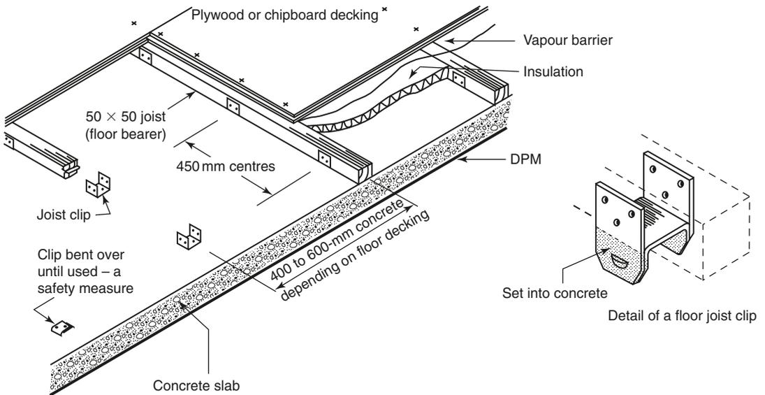
**Fig. 5.16** Joists (floor bearers) to a concrete floor
