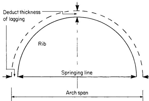
Fig. 4.11 Allowing for lagging
