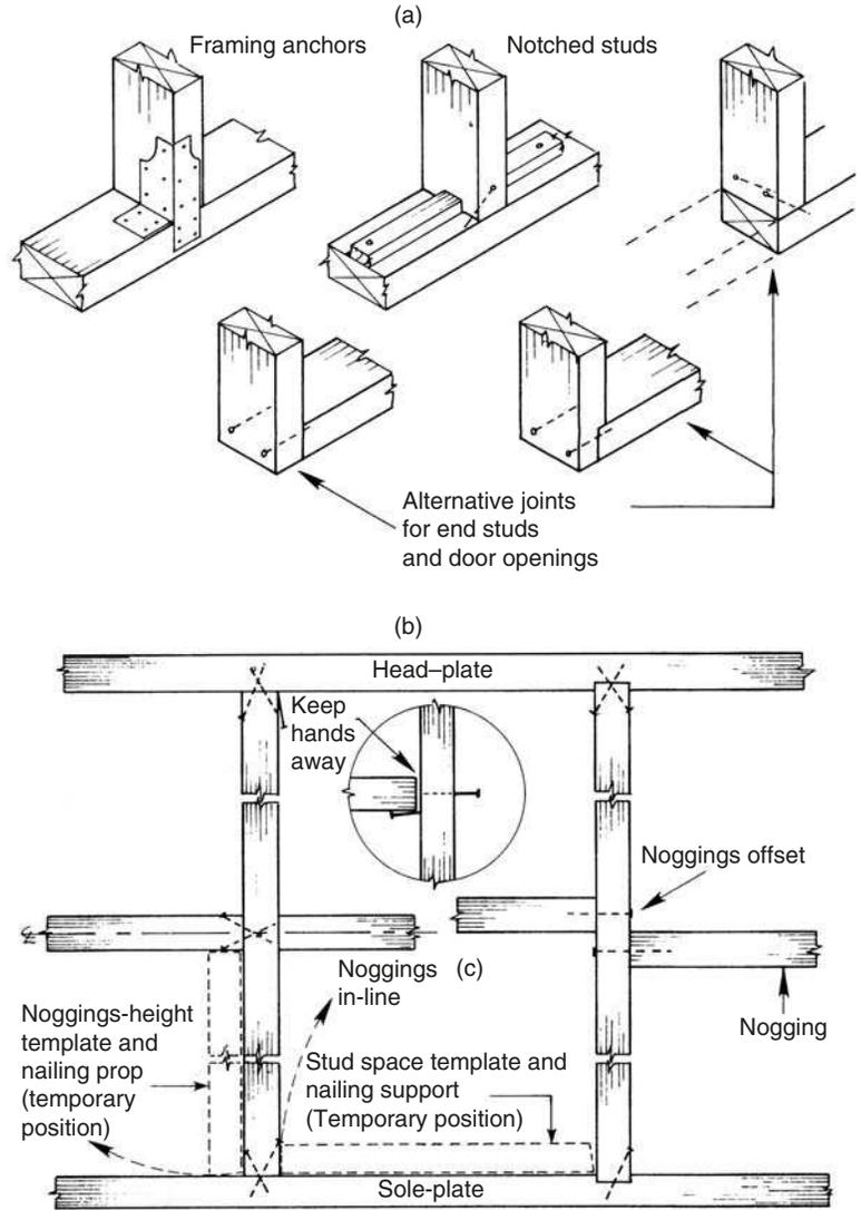
**Fig. 9.5** Joints and built-in framework
