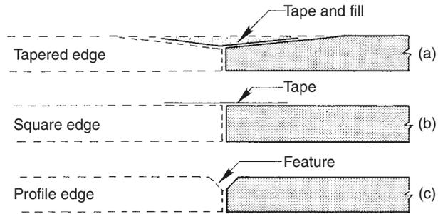
**Fig. 9.11** *Plasterboard-edge profiles*
