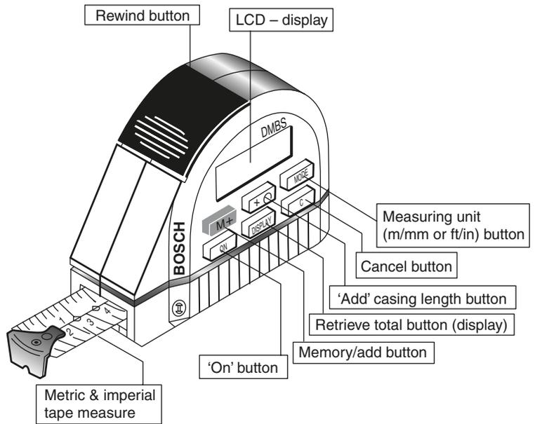
**Fig. 1.1** Bosch digital measuring tape
