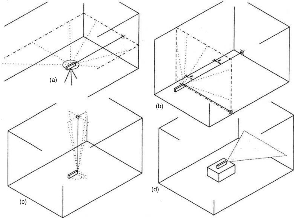
**Fig. 1.43** Applications: (a) Making a 'datum' level (perimeter of a horizontal plain); (b) Marking the perimeter of a vertical plain; (c) Transferring a ground point vertically; (d) Marking a straight line
