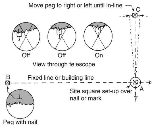
Fig. 1.16 Setting out a right angle with an optical square
