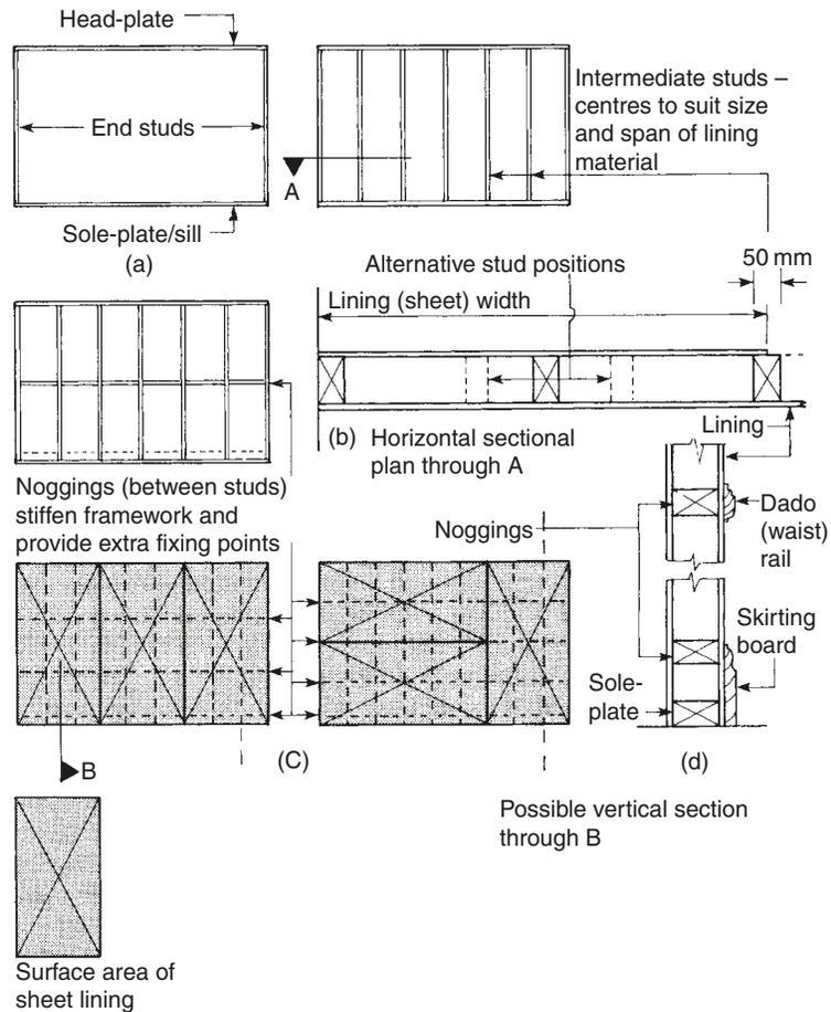
Note: Positions of studs and noggings will vary according to the size of lining sheets, amount of stiffening required, and fixing points for trims etc.
