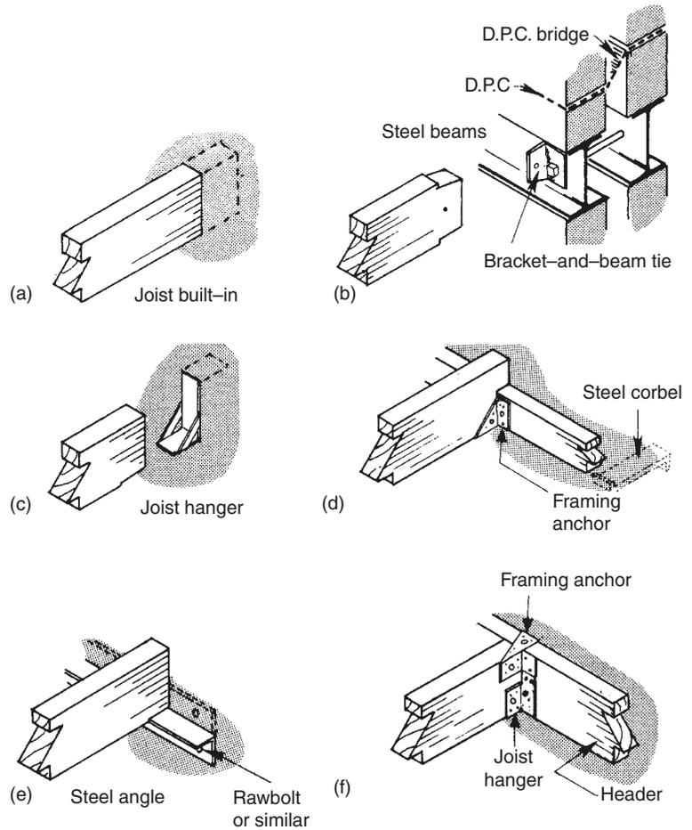
**Fig. 7.5** Joist bearings – abutting a wall (furring pieces not shown)
