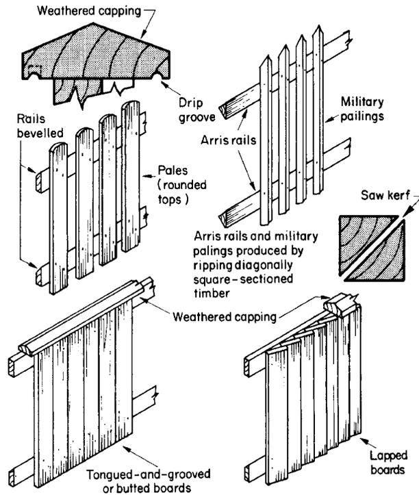
**Fig. 2.4** *Palisade and close boarded*
