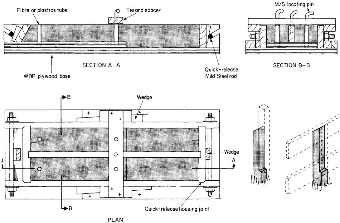
Fig. 3.5 Double mould box for pre-cast concrete posts
