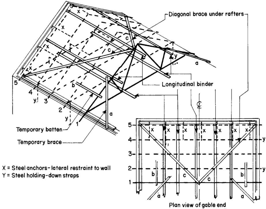
**Fig. 8.26** *Trussed-rafter-roof erection*
