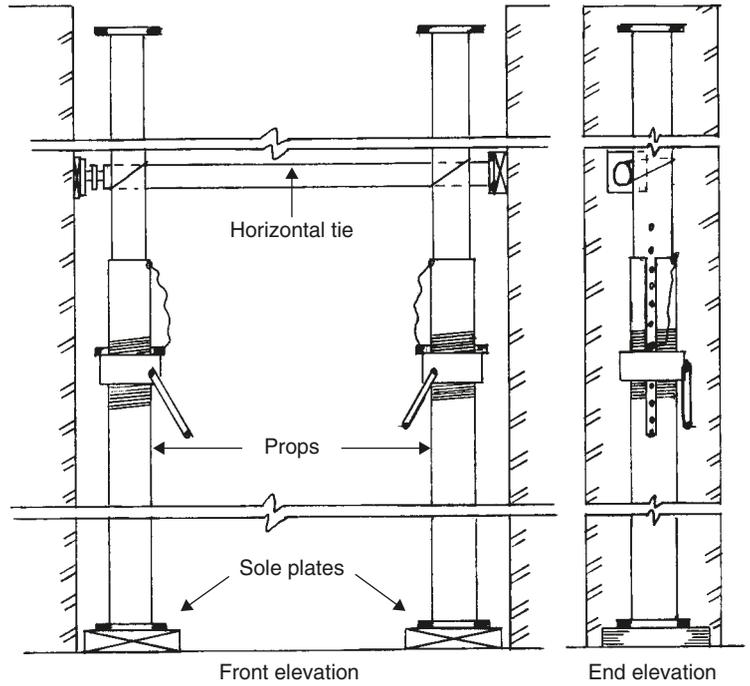
**Fig. 4.17** Supporting props levelled to receive arch centre
