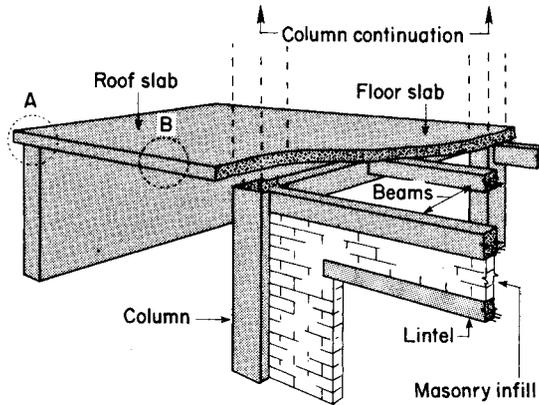
**Fig. 3.2** *Key to in situ structural elements*
