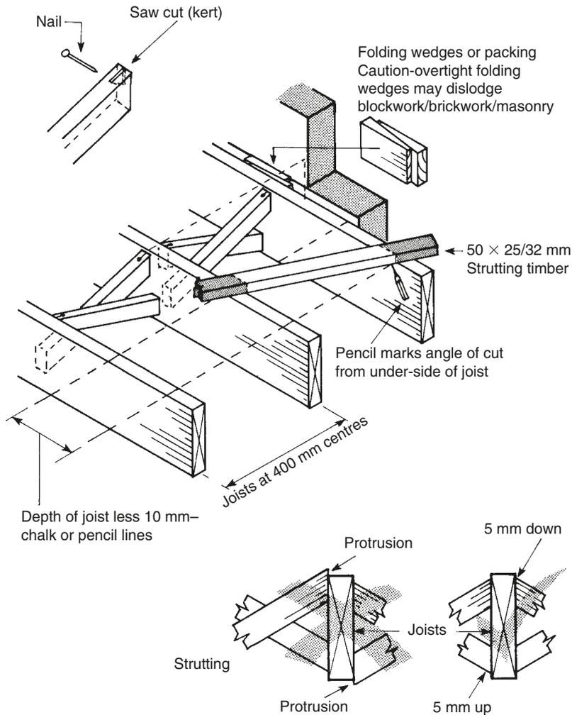
**Fig. 6.10** *Marking, positioning, and fixing herring-bone strutting*
