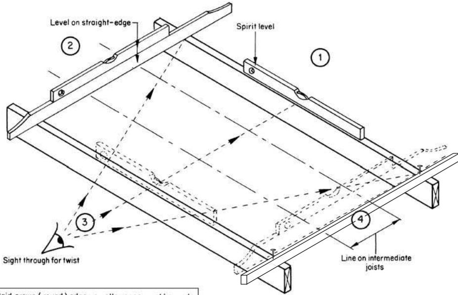
Note: joists laid crown (round) edge up – allowance must be made when levelling and sighting through
