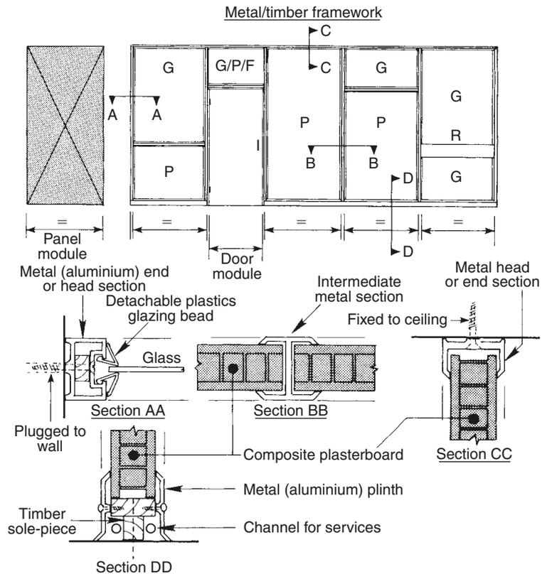
**Fig. 9.12** Typical demountable partition system, using metal section, composite plasterboard panels, and glass
