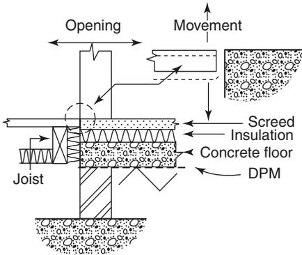
Always avoid butting timber and concrete surfaces together – uneven movement will damage floor coverings.
