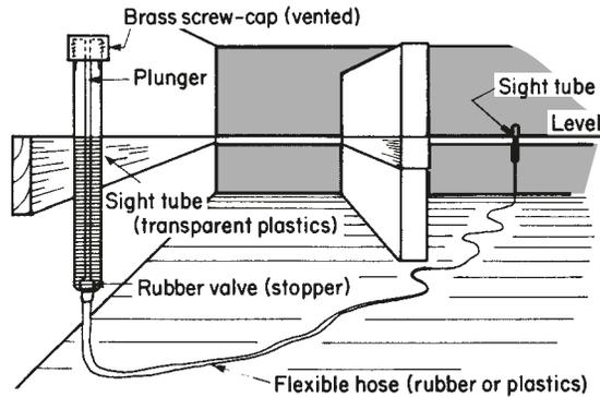
**Fig. 1.32** Two-man-operated water level
