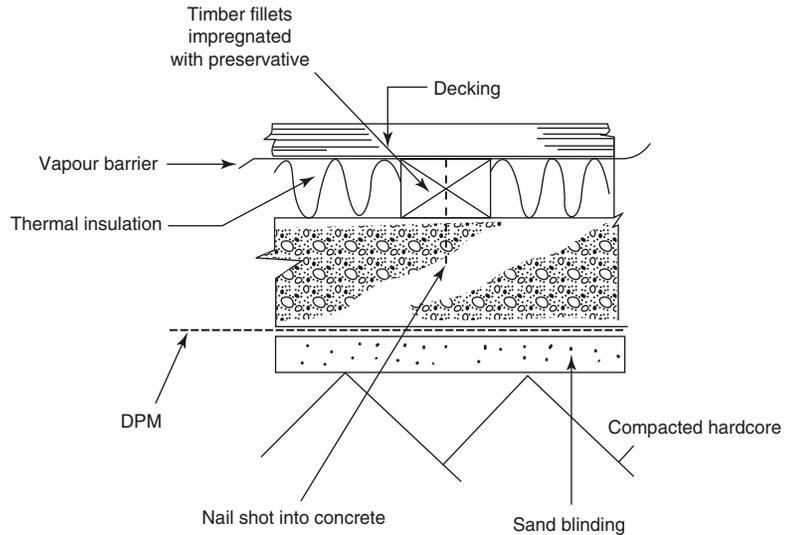
**Fig. 5.17** Vertical section of floors which incorporate timber
