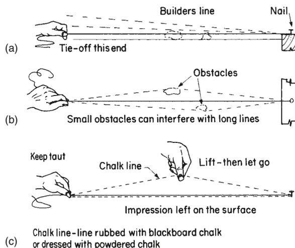
**Fig. 1.9** Using a builder's line to leave a straight chalk line impression on a flat surface
