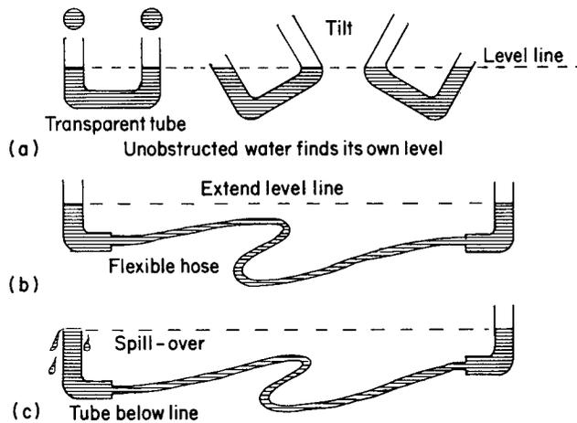
**Fig. 1.31** Basic principles of a water level
