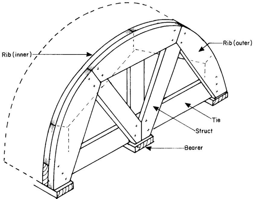
Note: a set of two laminated frames are required for each centre-assembled similarly to Fig. 4.14
