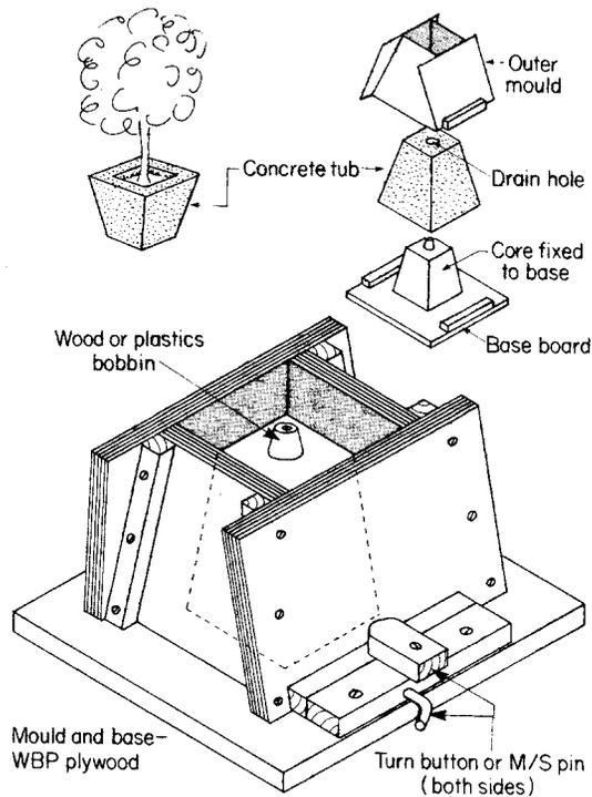
**Fig. 3.6** *Mould box for plant tub or litter bin*
