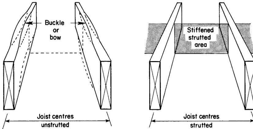
Note: Deep thin beams are inclined to buckle under load
