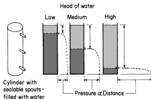
**Fig. 3.3** *The effects of hydrostatic pressure*
