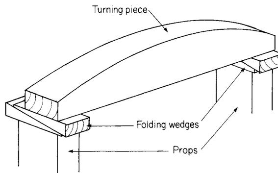
Fig. 4.10 Turning piece
