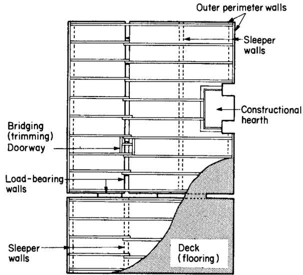
**Fig. 5.10** Ground-floor joist layout
