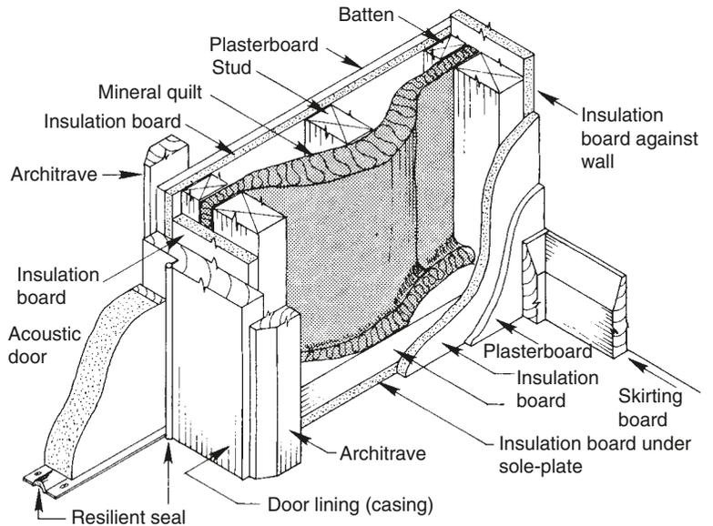
**Fig. 9.20** Improving sound insulation
