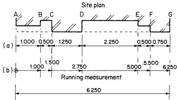
**Fig. 1.3** *Transferring measurements from a drawing to site*
