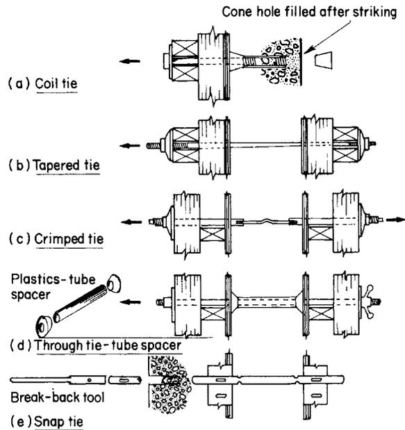
Note: Ties withdrawn in the direction of the arrow
