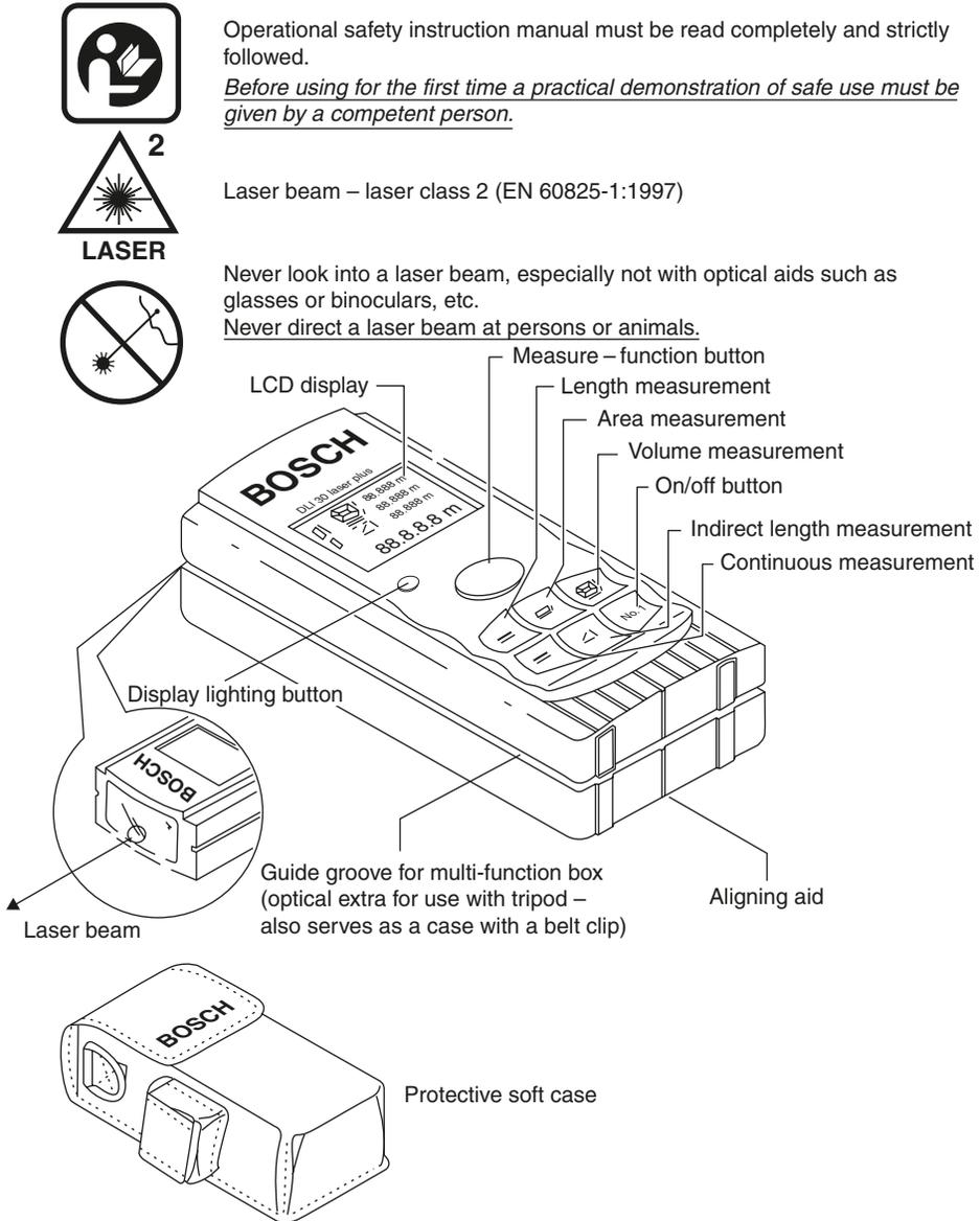
Fig. 1.4 Bosch Laser 'Rangefinder'
