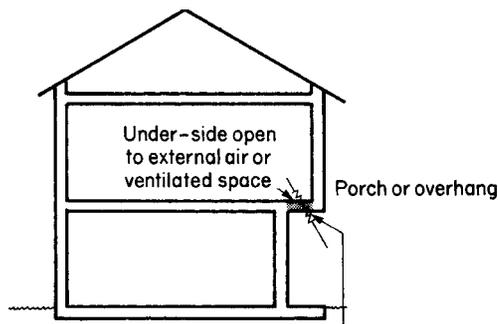
**Fig. 6.14** Floors requiring thermal insulation
