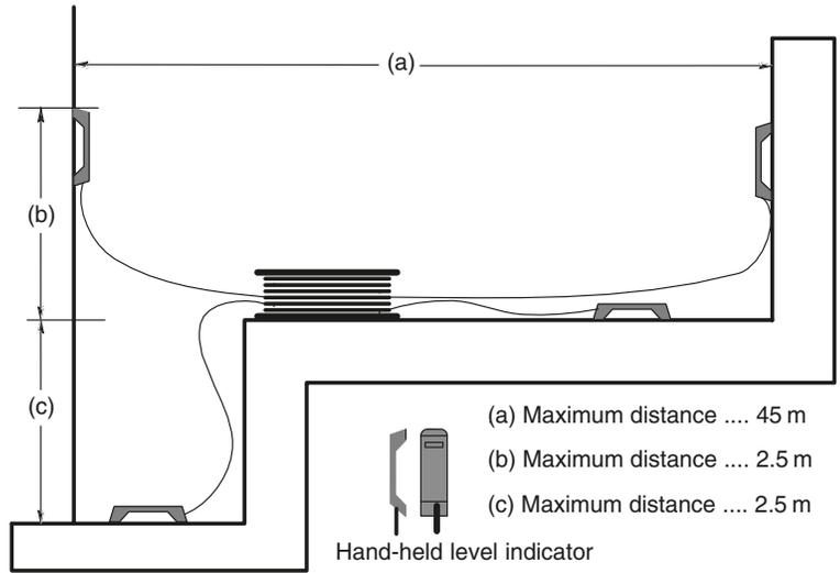
**Fig. 1.35** Horizontal and vertical range
