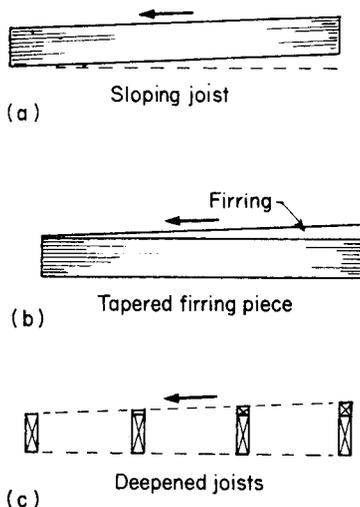
**Fig. 7.3** Alternative joist arrangements
