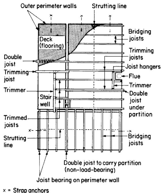
**Fig. 6.1** *Upper-floor joist layout*
