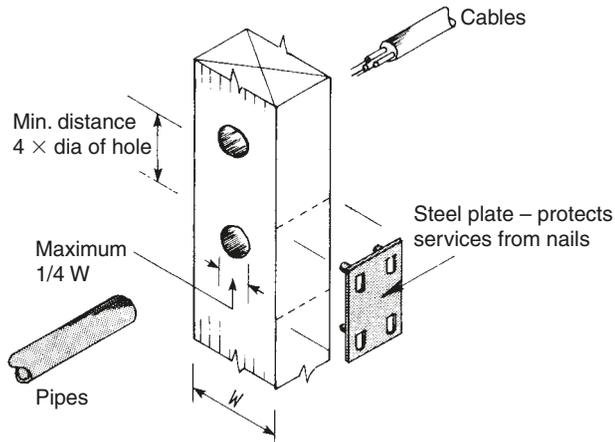
**Fig. 9.10** Positioning holes in framework for service pipes and cables (non-load-bearing partitions)
