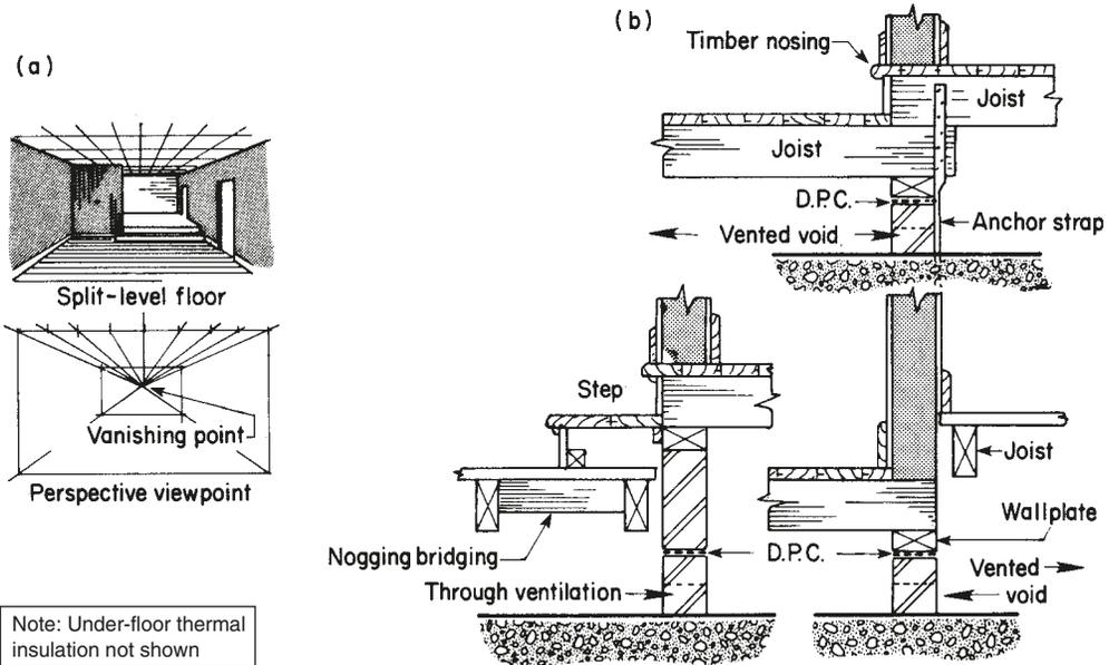
Fig. 5.14 Vertical section through timber-to-timber split level floors
