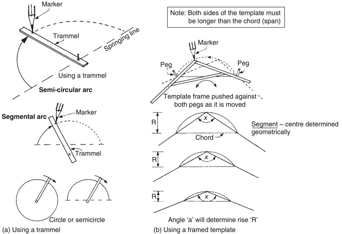
Fig. 1.26 Setting out large circles segments and arcs
