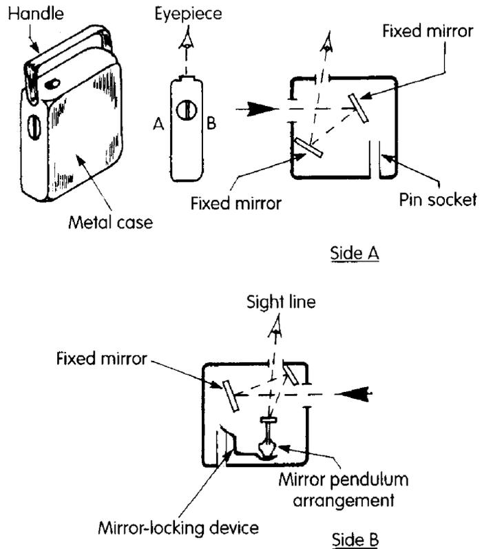
**Fig. 1.37** Cowley level and mirror arrangement
