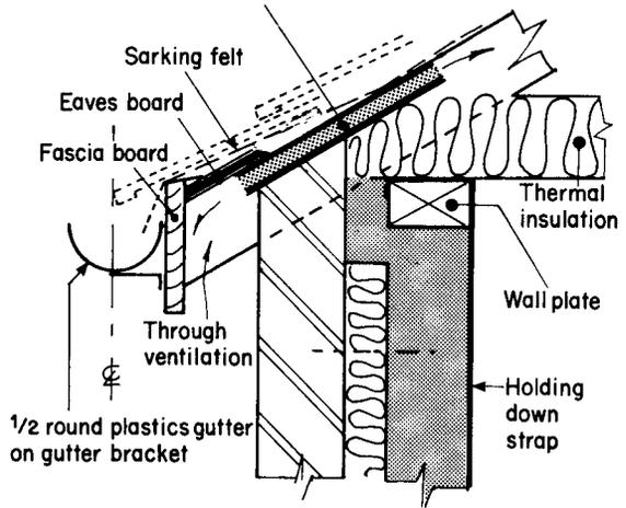
**Fig. 8.33** Proprietary roof ventilator used in conjunction with open eaves
