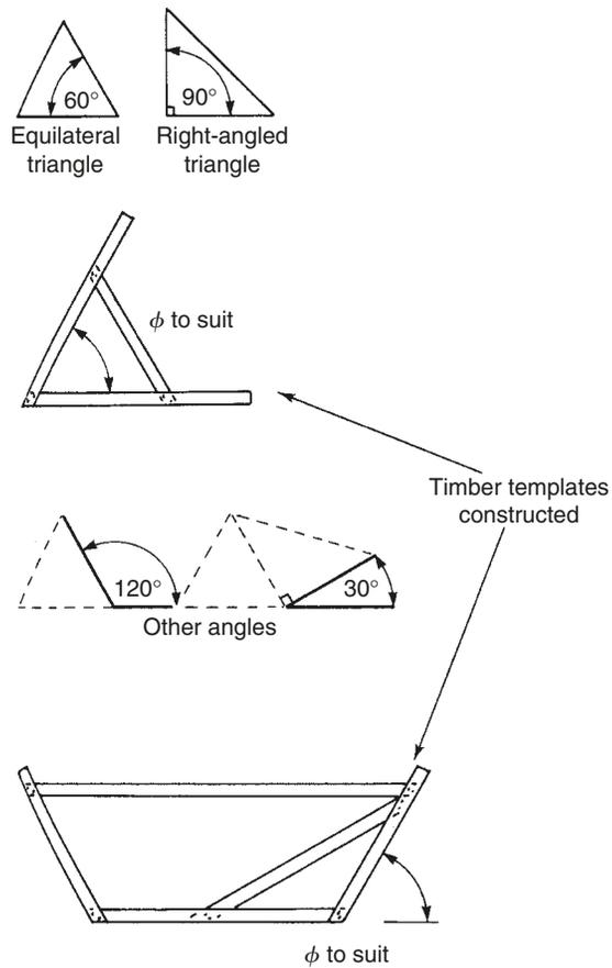
**Fig. 1.22** Fabricating angle templates
