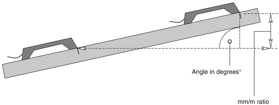
**Fig. 1.36** Positioning the hand-held device to inclined surfaces
