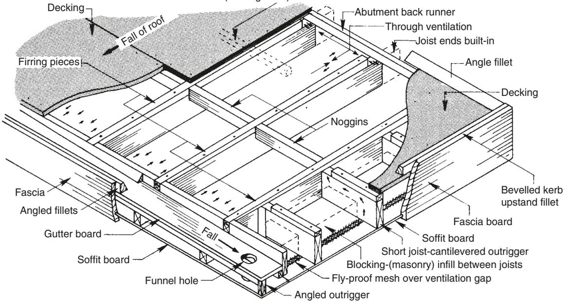
Note: Joists laid with 'crown' edge up. For the sake of clarity thermal insulation is not shown (see Fig. 7.10, 'Means of promoting cross ventilation')
