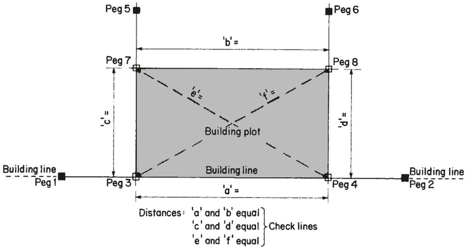
Fig. 1.20 Setting out a rectangular building plot
