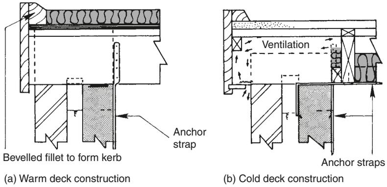
Note: For placement of thermal insulation see section 7.8. Cavity wall insulation not shown
