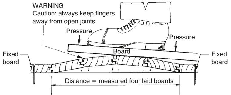
**Fig. 5.24** Folding method of laying floor boards
