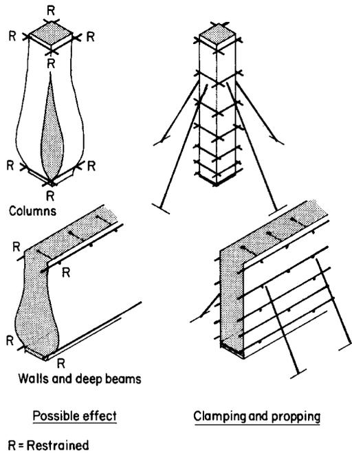
**Fig. 3.9** Resisting the effects of hydrostatic pressure
