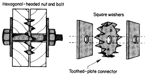
Fig. 8.21 Toothed-plate connection (double-sided connector)
