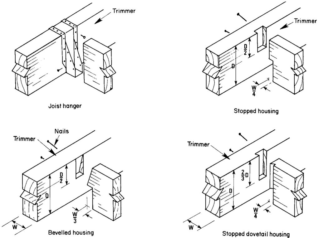
**Fig. 6.7** Joints – trimmed joist to trimmer
