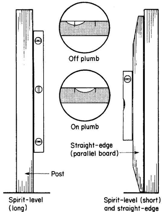
**Fig. 1.47** *Testing for plumb with a spirit level*
