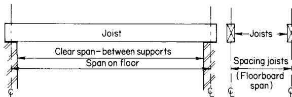
**Fig. 5.5** Floor joist end section in relation to its span
