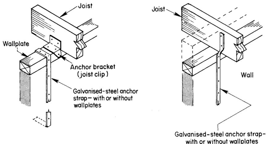
Fig. 7.8 Joist and wallplate anchorage
