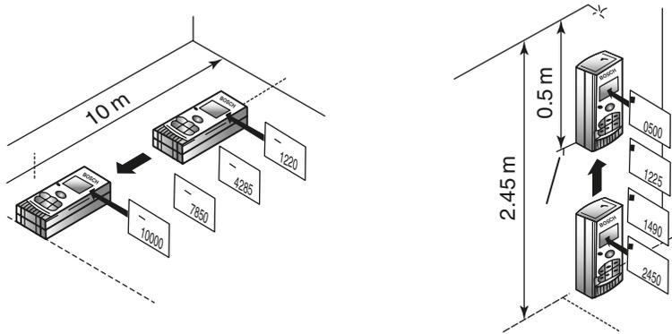
As the 'Rangefinder' is moved horizontally or vertically from a solid object or surface – distances are registered on the LCD panel
