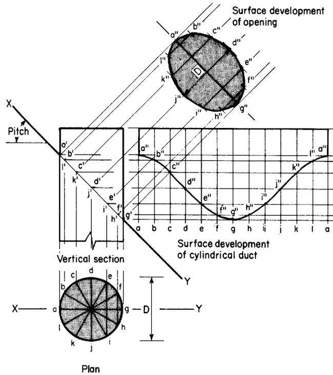
**Fig. 8.31** Cylindrical duct piercing a pitched roof
