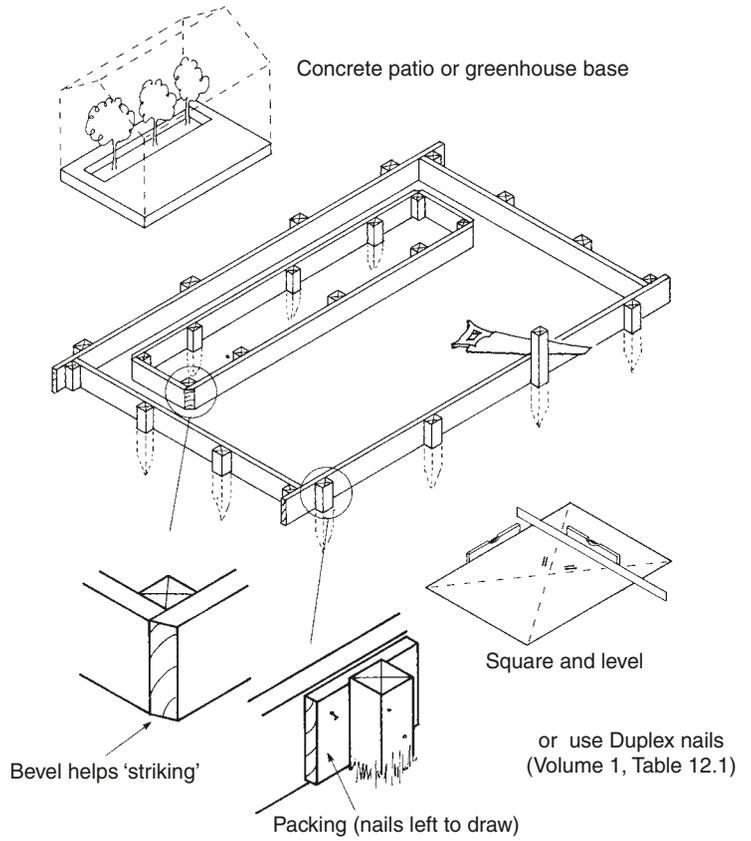
**Fig. 3.8** Formwork for an in situ concrete patio or base
