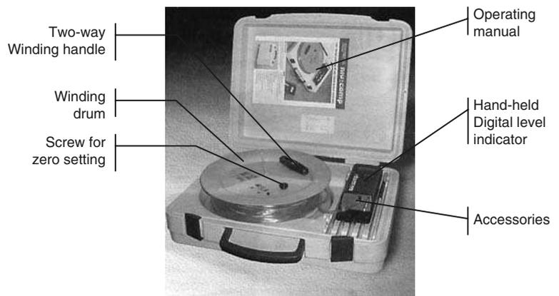
**Fig. 1.33** The 'Comp-Mark' electronic level
