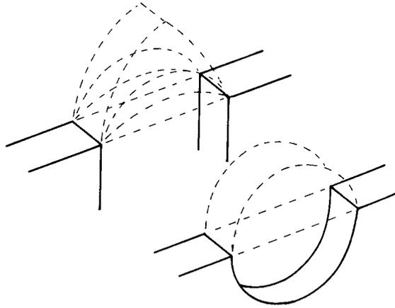
**Fig. 4.2** Centres predetermine the shape of an opening
