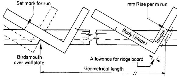
**Fig. 8.16** *Applying a steel roofing square to produce a pattern rafter*
