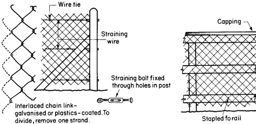
**Fig. 2.2** *Chain-link fencing (galvanised or plastics coated)*
