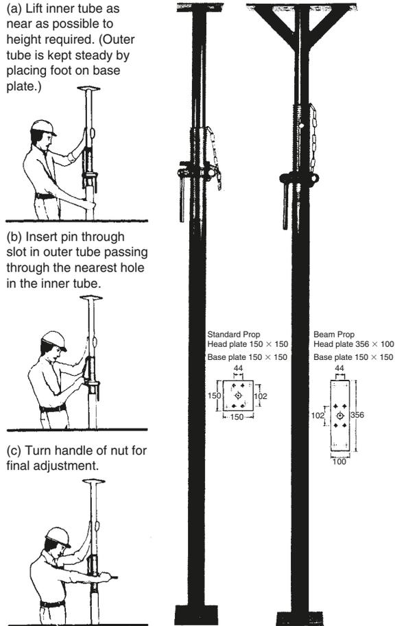
**Fig. 3.20** 'Acrow' adjustable steel props
