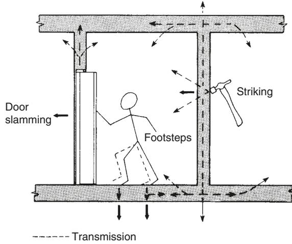
**Fig. 9.18** Impact sound (structure borne)
