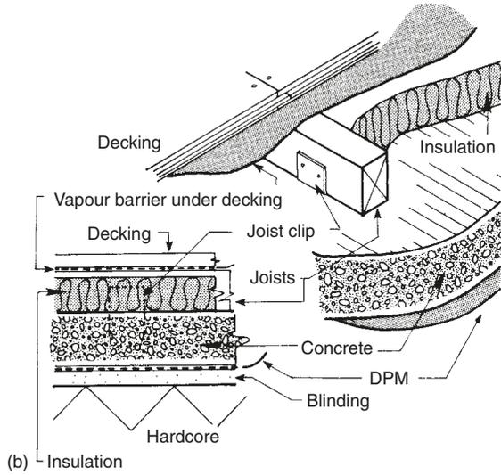
Note: Method (b) unsuitable in situations where water may be spilled over the decking – water would be held back by the vapour barrier.
