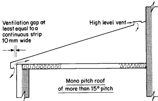
**Fig. 8.34** Method of promoting cross-ventilation to a roof space
