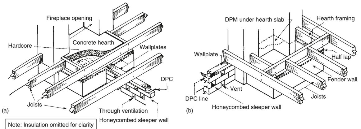
**Fig. 5.12** Alternative joist arrangement to a ground-floor construction hearth
