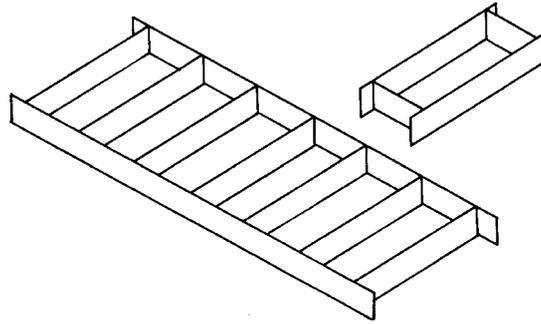
Fig. 3.4 Single and multiple casting units
