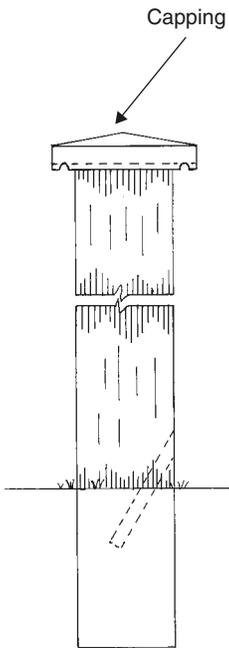
**Fig. 2.22** Using capping
