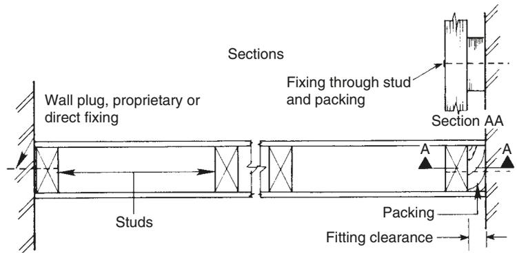
Figure 9.7(b) shows how a pre-assembled framework is wedged and packed-up off the floor before fixing. Where the head-plate falls between two ceiling joists, noggings are used as restraints and fixings.
