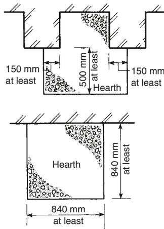
**Fig. 5.11** Constructional hearths (solid fuel and oil-burning appliances)
