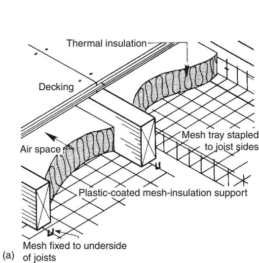
Note: Plastic netting may also be used to retain thermal insulation.
