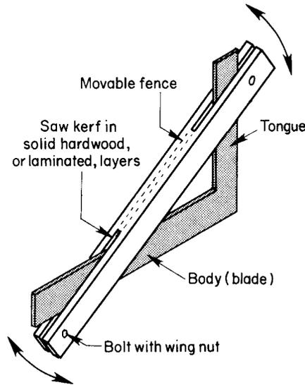
**Fig. 8.17** *Steel roofing square with movable fence*
