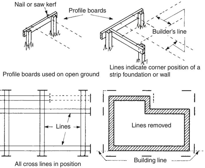
**Fig. 1.21** Using profile boards to line out the position of a wall and/or foundation
