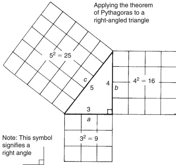
**Fig. 1.12** Using a ratio of 3:4:5 to form a right-angled triangle
