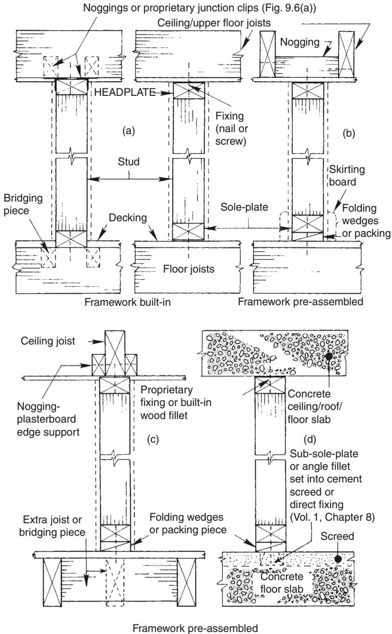
**Fig. 9.7** Vertical sections through built-in and pre-framed partitions
