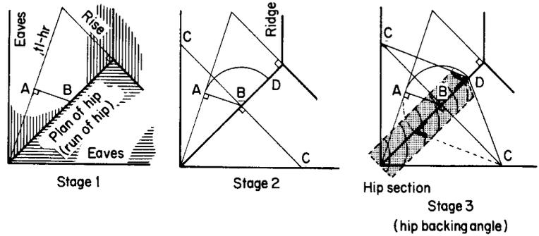
**Fig. 8.10** Hip-rafter backing (half-dihedral) angle
