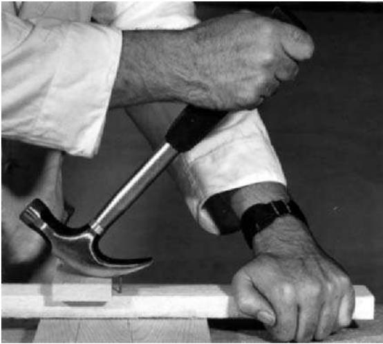
**Fig 5.68** Withdrawing a nail using a claw hammer. Leverage should be terminated and a hammer repositioned by using a packing (as shown) before the hammer shaft reaches the upright position, or an angle of 90 degrees to the face of the work piece – otherwise undue stress could damage the hammer shaft
