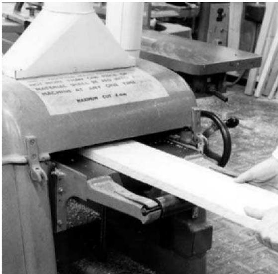
**Fig 9.34** Thicknesser displaying a notice stating that 'not more than one piece of material shall be fed into this machine at any one time'
