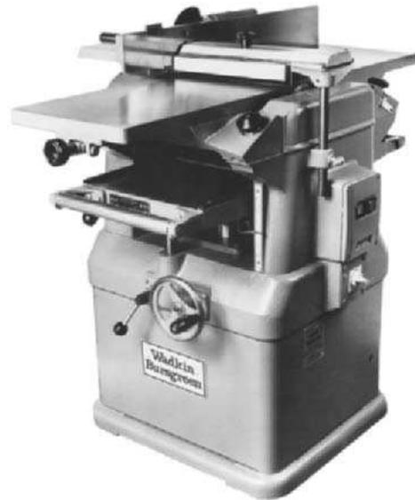
**Fig 9.24** 'Wadkin' surface planer and thicknesser combined
