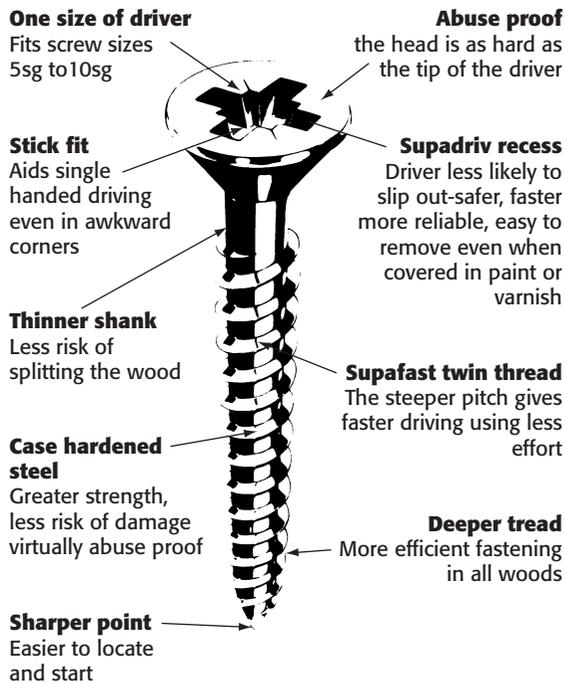
**Fig 12.6** Supafast threaded screws
