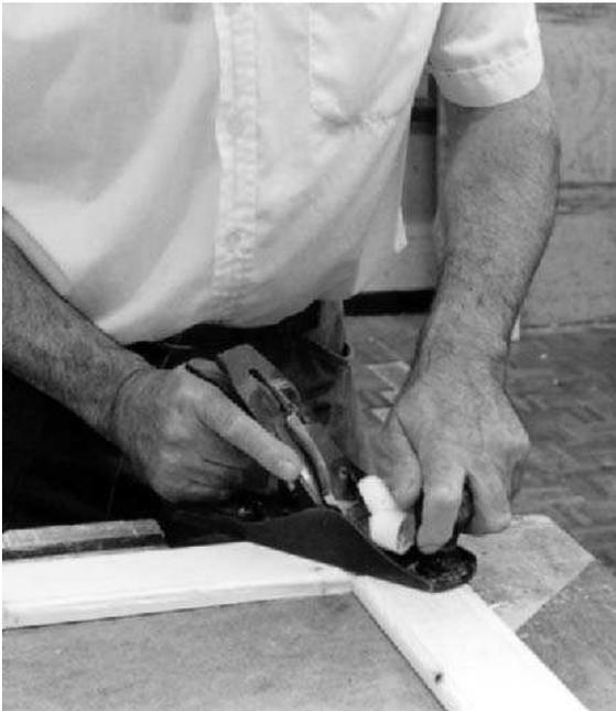
(b) Dressing flat a joint between door stile and rail – a slow turning action towards the joint helps to avoid unnecessary tearing of the grain
