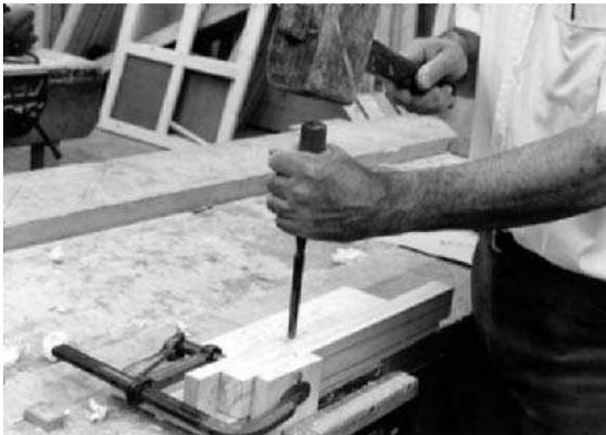
**Fig 5.64** Chopping a mortice hole – notice the use of scrap wood to protect the bench and work piece, and how the clamp has been laid flat with protruding bar and handle positioned towards the well of the bench, out of harms way
