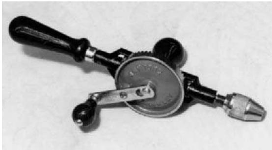
**Fig 5.58** Hand drill (wheel brace) (with kind permission from Stanley tools limited)
