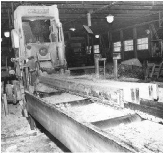
**Fig 1.9** Vertical frame saw or gang saw
