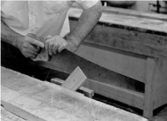
**Fig 5.16** Sawing down the grain with the material angled – two saw lines are visible
