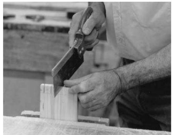
**Fig 5.19** Dovetail saw – starting a cut
