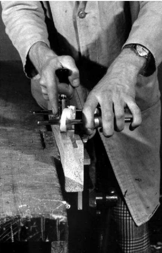
**Fig 5.48** Cutting a groove with a plough plane
