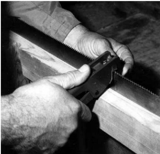
**Fig 5.113** Setting saw teeth. **Note:** exposed teeth should be covered with a blade sheath (Fig. 102b & c)
