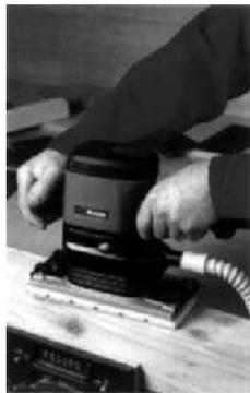
Orbital sander in use with attached dust extraction hose
