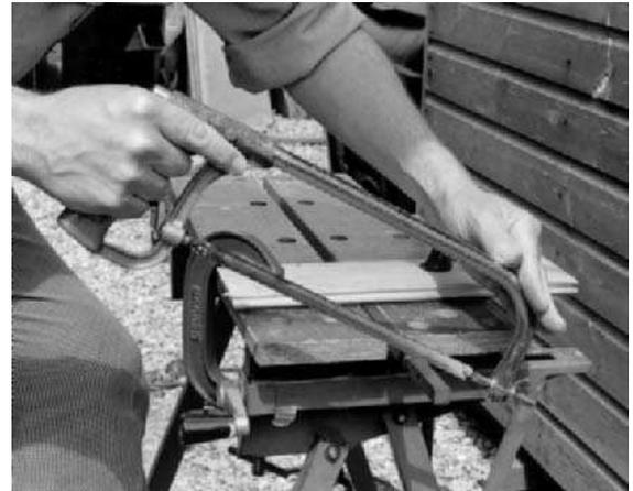
**Fig 5.21** Using a standard hacksaw
