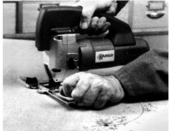
**Fig 6.35** Using a jig saw with a circle cutting attachment
