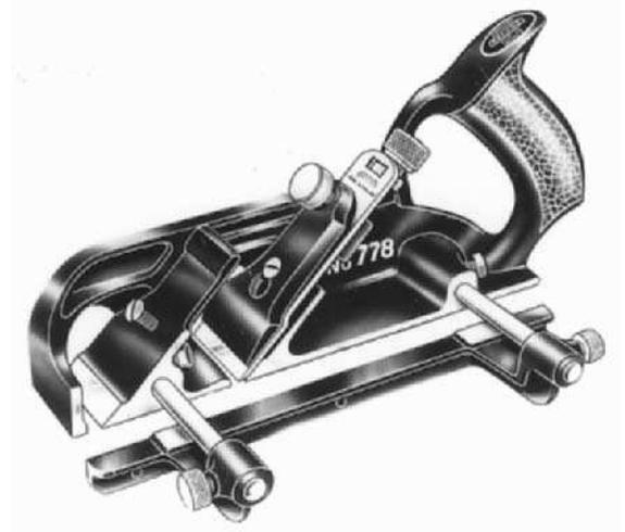
**Fig 5.32** Rebate plane (with kind permission from Record tools limited)
