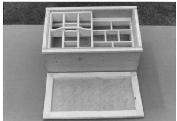
**Fig 15** Fitting trays into the chest
