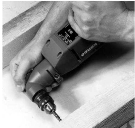
(b) Using an angle-drill attachment
