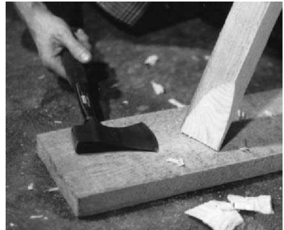
**Fig 5.65** Using an axe to cut a taped end on a short length of timber
