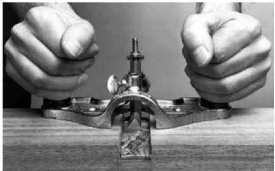
**Fig 5.37** Open – throat router and its use (with kind permission from Stanley tools limited)
