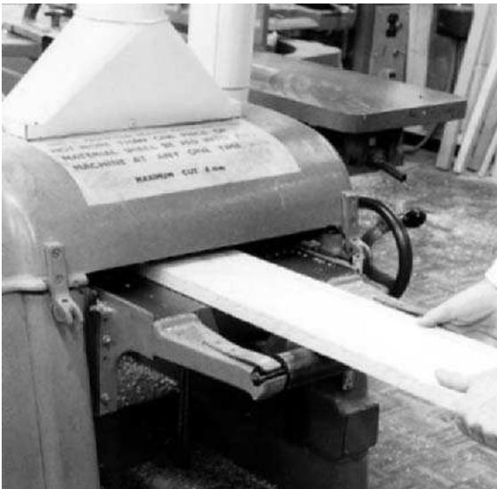
**Fig 9.37** Thickener displaying a notice stating that 'not more than one piece of material shall be fed into this machine at any one time'
