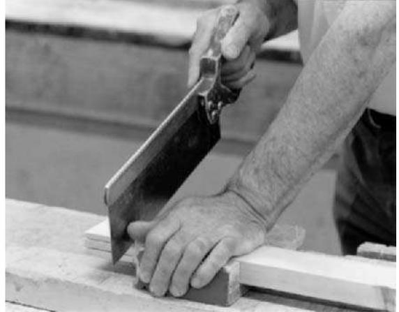
**Fig 5.17b** Tenon saw – starting a cut using a bench hook
