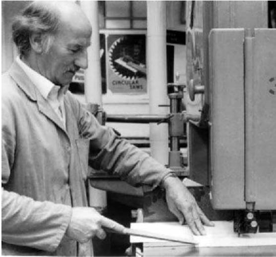
(a) Ripping - using a push stick to finish the last 300mm of cut
