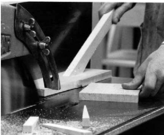
**Fig 9.11** Using a jig to cut wedges. Note: a pushstick must be used to hold the wood being used as wedges against the jig
