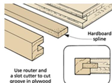
For the splines, I like to use hardboard. Its uniform thickness makes it easier to fit the spline into the grooves. So all you have to do is rip the splines to width to fit the grooves.
