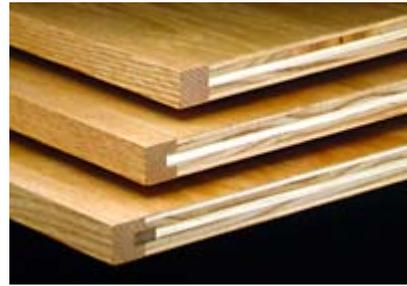
There are a number of ways you can edge plywood — from iron-on veneer to plastic T-moulding. But I generally have enough solid wood scraps lying around that I don't need to buy edging. I just have to decide how to apply the narrow strips to the edges.
