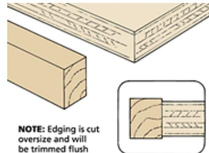
This method works fine for shorter pieces. But when you've got a longer piece of plywood, keeping the edges aligned can get a little tricky (even with oversized strips). One way to get around this problem is to nail the edging in place. (Note: Drill holes for the nails to prevent splitting.)
