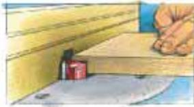
**4 Router table with a straight bit.** Although you can't easily rabbet large pieces on a router table, this method has some distinct advantages over a handheld router. First, a router table has a fence that ensures a perfectly straight rabbet (a bearing-piloted bit will follow any irregularities in the workpiece edge). And, although a piloted rabbeting bit will help you cut a rabbet up to 1/2" wide and 1/2" deep, you can put a large straight bit in a router table and cut rabbets up to 1X1".
