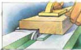
**5 Jointer.** We admit we rarely use a jointer to cut rabbets, but if you must cut a perfectly smooth rabbet over 1" wide, and along a straight, outside edge, look to a jointer. You can cut a rabbet as wide as the length of your jointer's cutterhead. The maximum cutting depth of your jointer will limit the depth of the rabbet, typically to 1/2".
