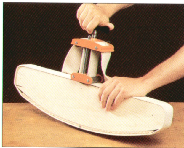
The slats for a ladder-back chair like the one shown on page 50 can be bent dry, using the jig shown above. Made from two thin wood strips face-glued together, each slat is held by a web clamp against a form, which is cut to the desired curve.
