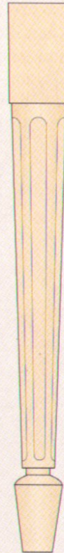
Turned leg A decorated version of the Hepplewhite-style leg shown at left. This leg is turned on the lathe (page 102); the flutes that run lengthwise can be produced by hand or with a router and a fluting jig while the leg remains on the lathe
