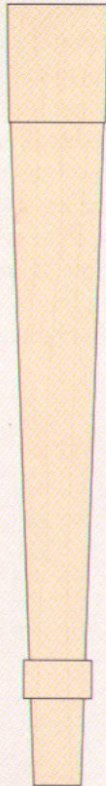
Tapered leg with square bead A variation of the tapered leg with a taper on four sides and a bead fashioned by hand; a feature of some Hepplewhite furniture
