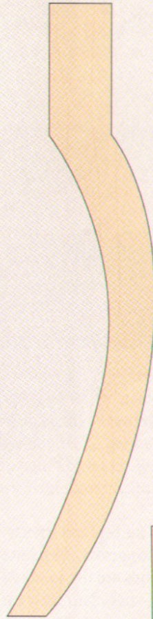
Saber leg A traditional leg design for chairs in formal settings; the saber shape can be produced on the router table in the same manner as the rear legs for a frame chair (page 31)
