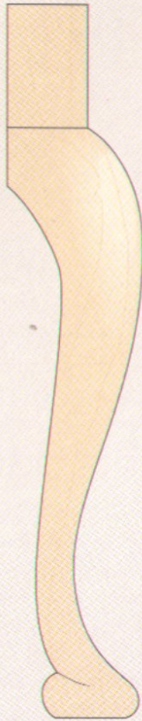
Cabriole leg A traditional leg style cut on the band saw and shaped by hand (page 98)
