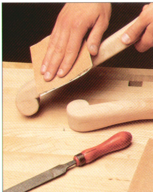
A pair of chair arms is given a final sanding before being installed. Depending on the design of the chair, the arms can be left square or shaped with gentle curves, as in the graceful arms shown above.
