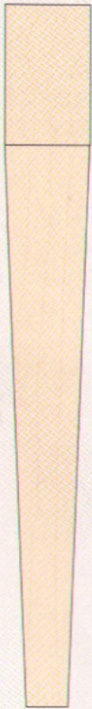
Tapered leg with pommel Adaptable to many designs; tapered on two or four sides on the jointer or table saw (page 101)
