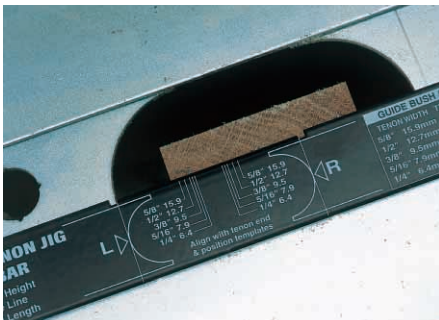
The setting bar uses the centre line of the joint to align everything correctly.
